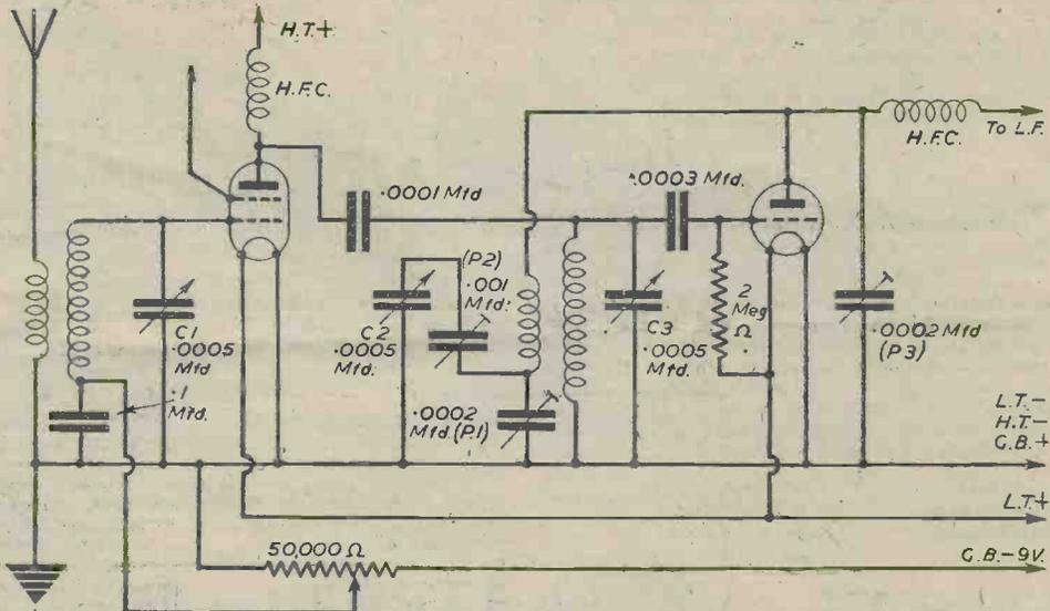
Fig. 3.—Automatic reaction will make the receiver sensitive throughout the tuning range.
