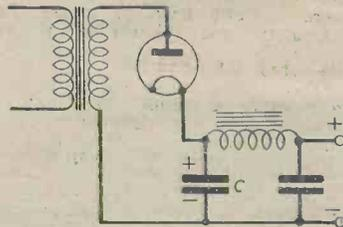
Fig. 3.—What would be the effect of a "break" in the reservoir condenser C?
