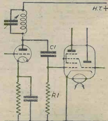
Fig. 2.—With tuned-anode coupling there is always danger of passing hum ripple from the anode circuit to the following grid; and component values should be chosen to attenuate such frequencies as much as possible.
