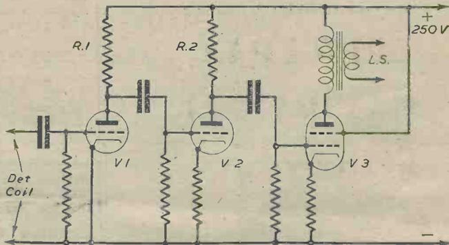
Fig. 3.—A similar circuit to Fig. 2 but with a triode input stage.
