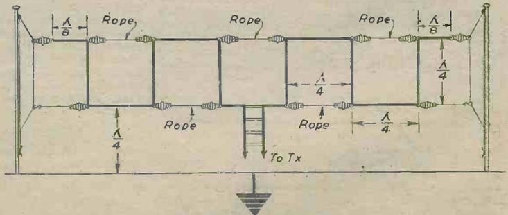
Fig. 5.—A Bruce folded aerial—ideal if there is sufficient room to accommodate it with two or more wavelengths.
