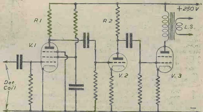
Fig. 2.—Result of eliminating certain of the decoupling components from Fig. 1.
