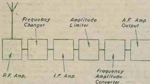
Fig. 1.—This block diagram shows the basic stages of a frequency-modulated superhet receiver.
