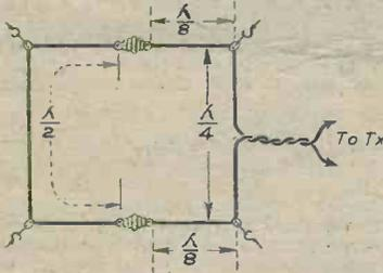
Fig. 4.—A folded dipole with reflector which can be easily fitted up in a loft for 14 mc/s or higher.
