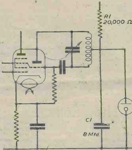
Fig. 3.—The use of a voltage stabiliser to prevent frequency variation caused by audio frequency feed-back or hum.
