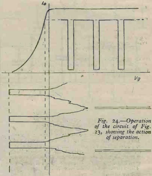
Fig. 24.—Operation of the circuit of Fig. 23, showing the action of separation.
