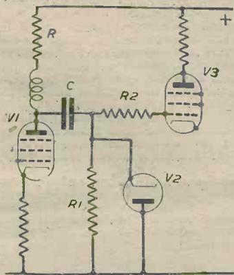
Fig. 25.—When the synch separator is fed from the video stage through a resistance-capacity coupling, a D.C. restoration diode must be inserted as shown.
