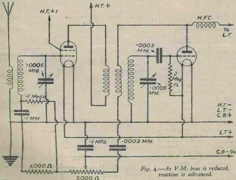
Fig. 4.—As V.M. bias is reduced, reaction is advanced.
