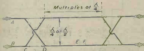
Fig. 3.—The Sterba, and modifications of it, follows the above form. 600-ohm feeders may be taken from AB, CD or EF, according to the size of the array.
