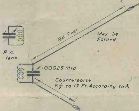
Fig. 2.—The W3EDP aerial, which is very efficient and may be folded to occupy small space without greatly impairing efficiency.
