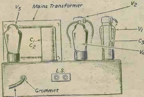
Fig. 4.—A rear view of the completed amplifier.
