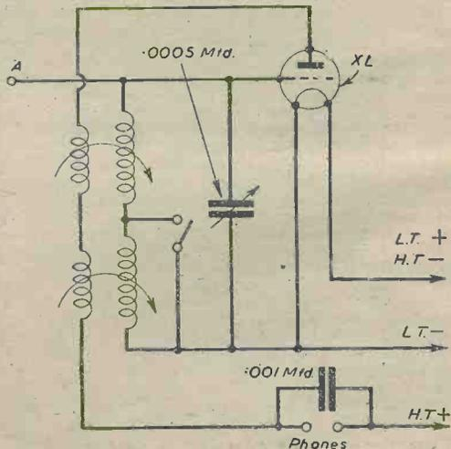
Fig. 3.—The circuit diagram of the pocket receiver.
