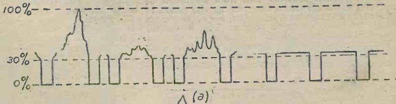
Fig. 20.—When the D.C. component is removed from the vision signals as at (b), synch separation by means of an amplitude filter is not possible.
