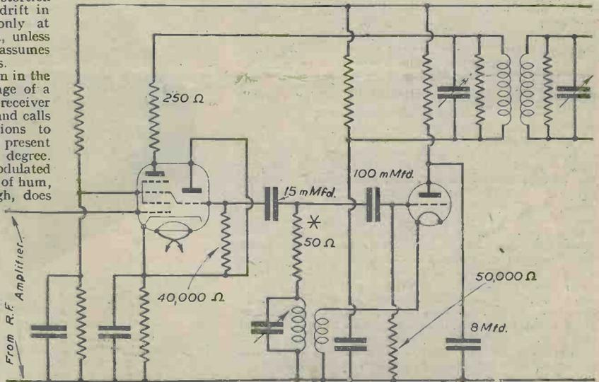
Fig. 4.—The basic circuit of a frequency-changer stage, used by the writer for 24-30 mc/s; decoupling condensers were all .05 mfd. (paper, except for the 8 mfd.) and all were shunted by .0001 mica. Resistance marked \* must be non-inductive. Values used were 6K8 (triode-hexode) and 6K5 (triode).
