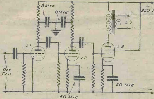
Fig. 1.—Standard L.F. amp. circuit with decoupling.
