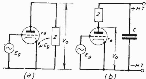
Fig. 1—A simple problem circuit. Are  $Z$  and  $r_a$  in series or parallel?
