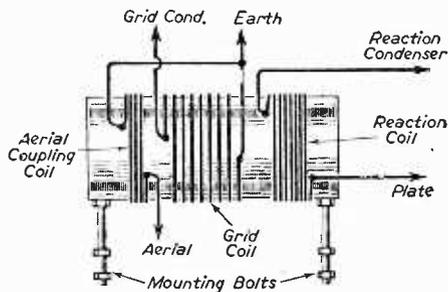
Fig. 5.—A simple short-wave coil.
