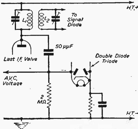
Fig. 6.—Typical circuit showing how the A.V.C. voltage is sometimes obtained from the anode of the last I.F. valve. In this case  $L_2$  is not included in the A.V.C. circuit.
