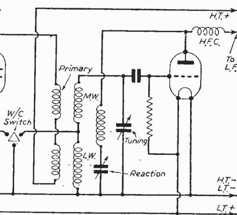
Fig. 6.—Ultra-short-wave coils may be made up as shown here.
