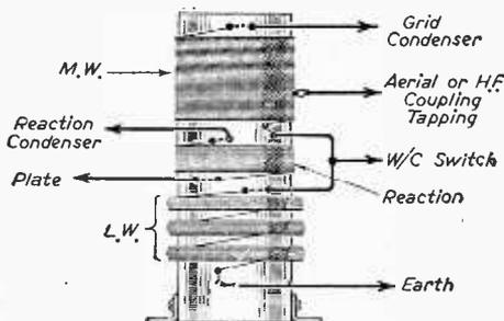
Fig. 1.—A simple dual-range coil.
