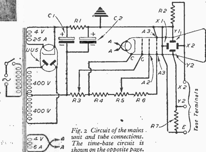
Fig. 2 Circuit of the main unit and tube connections. The time-base circuit is shown on the opposite page.
