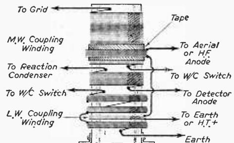
Fig. 2.—A dual-range coil of the H.F. transformer type.
