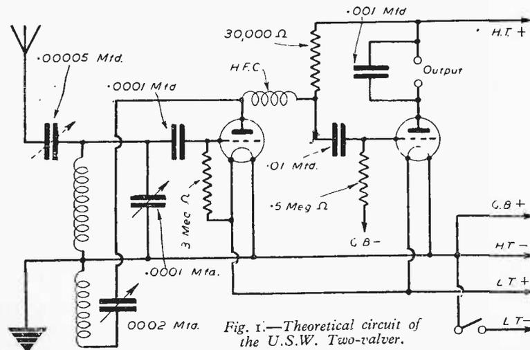
Fig. 1.—Theoretical circuit of the U.S.W. Two-valve.
