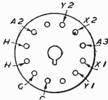
Fig. 4. Connections to the tube base.
