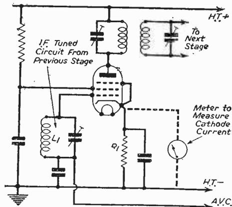
Fig. 2.—Circuit of A.V.C. controlled I.F. stage, A.V.C. being applied to the grid of the valve via coil L1. The "trimming meter" is connected across resistance R1.
