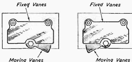
Fig. 5.—This illustrates how two different positions of an air-spaced trimmer will give the same capacity.
