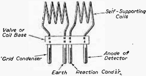
Fig. 7.—Another form of interchangeable U.S.W. coil.
