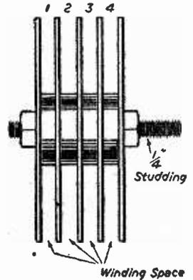
Fig. 4.—Bobbin assembled on  $\frac{1}{2}$  in. rod for holding in winding mechanism. This can be an ordinary geared drill brace or a specially built machine.
