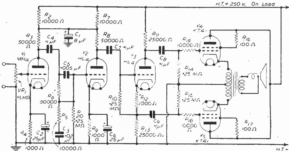
Fig. 3.—Circuit of the complete amplifier described here
