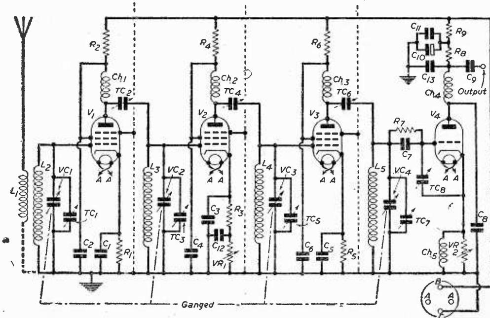
Theoretical circuit of the 4-valve U.S.W. receiver, showing plug for connection to suitable amplifier.
