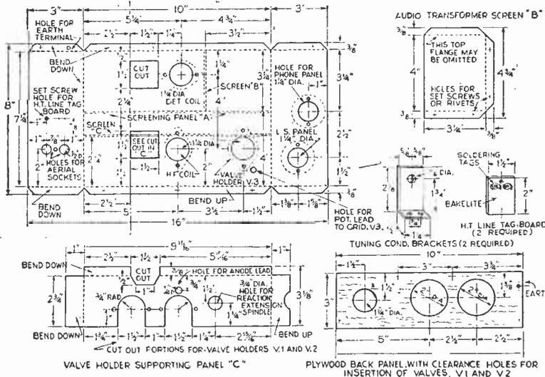
Fig. 4.—Cutting and drilling details for the chassis, screen, etc.
