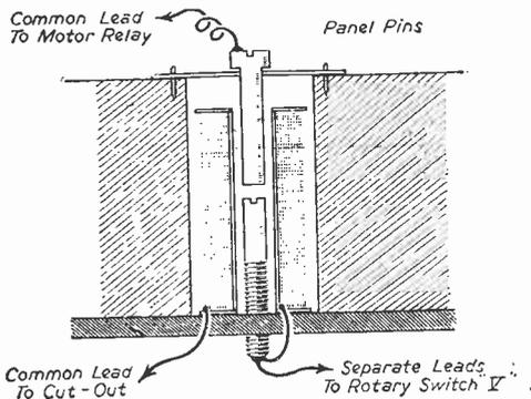
Fig. 4.—Details of the relay construction.
