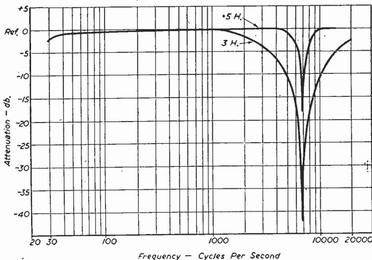
Fig. 2.—Showing the response curves obtained with a flat input when the 5 henry tap and the 3 henry tap are in use.
