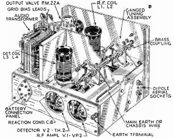
Fig. 1.—Pictorial view of the completed receiver. The photograph on the cover shows the under view of the set.
