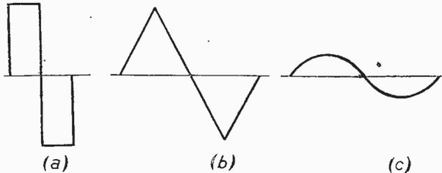
Fig. 6.—None of these look very much like "sine-waves," but each is made up of a number of pure sine-waves of different frequencies, i.e., each contains a number of "harmonics."
