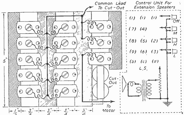
Fig. 5.—Details of assembly of the complete relay bank, and, on the right, the control unit wiring for the extension speakers.
