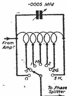
Fig. 1.—Shows the choke and condenser forming a tuned circuit between the pre-amplifier stage and the phase-splitting stage.
