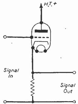
Fig. 4.—The cathode loaded valve stage.
