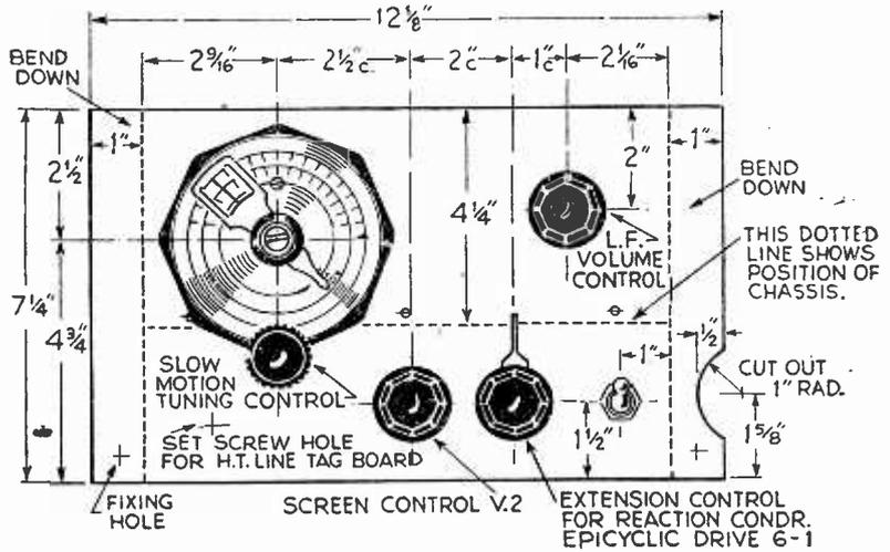
Fig. 5.—Drilling and layout details for the panel and controls.
