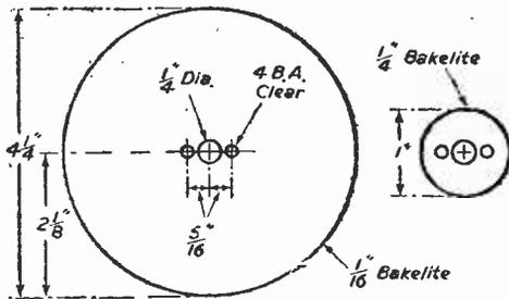
Fig. 3.—Details of the discs for the bobbin showing drilling dimensions.
