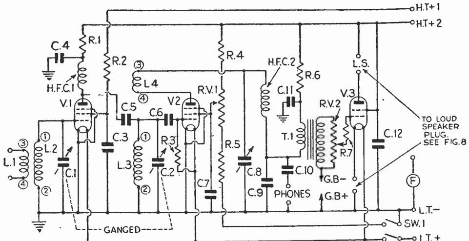
Fig. 2.—Circuit of the Short-wave Battery Three.
