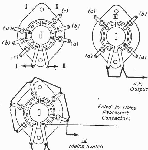
Fig. 3.—Connections of the switch wafers.
