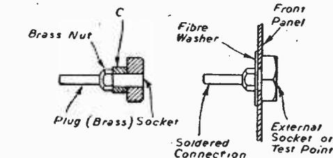
Method of making insulated sockets.
