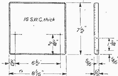
Fig. 4.—Details of the end plates. Two are required, one left-hand and one right-hand.
