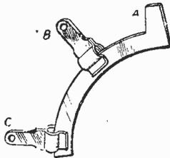
Fig. 1.—The arrangement adopted in one of the well-known, British makes of multi-contact switch.
