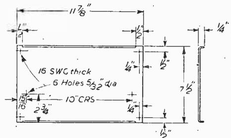
Fig. 3.—Details of the panel.
