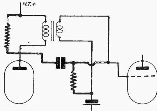
Fig. 7.—Diagram illustrating the changes necessary between L.F. transformer and resistance-capacity coupling, the latter indicated in heavy lines.
