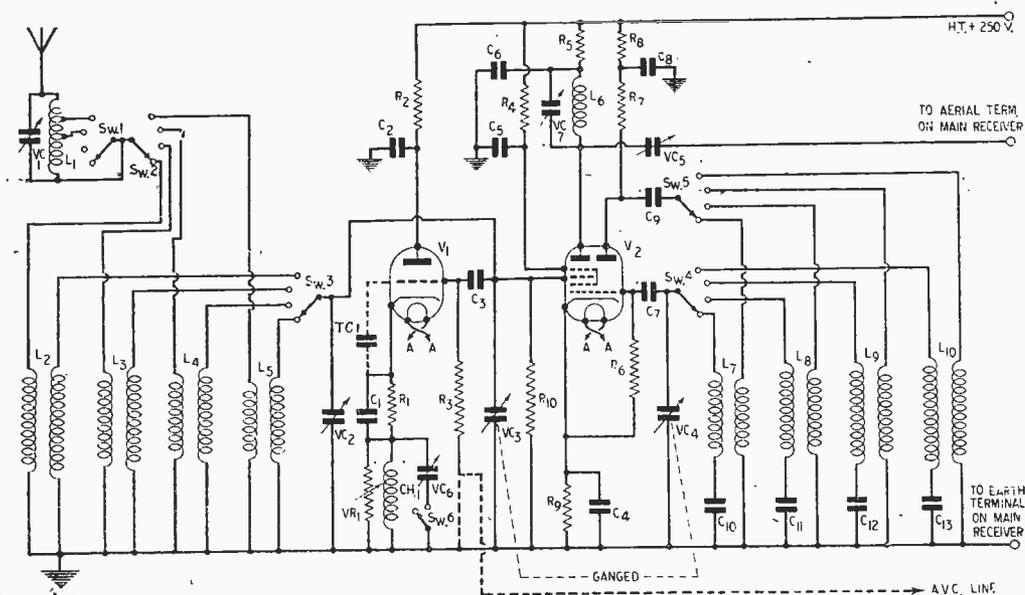
Fig. 1.—Theoretical circuit of the converter unit.
