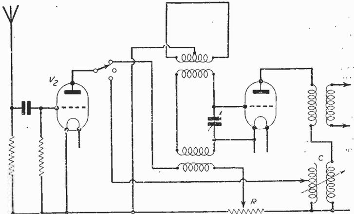
Fig. 5.—An interesting circuit, using an aperiodic loop and tuned circuit.
