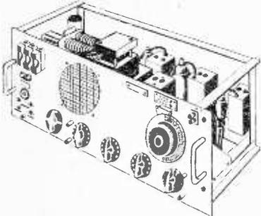
This is a very fine set built with precision; the frequency coverage is from 10-60 mc s. c., 5-30 metres. The receiver with power supply for working off mains or 6v. battery and 6in. loud-speaker is built on a steel chassis and housed in a steel cabinet. The chassis slides into the front of the cabinet and has handles for withdrawal. The circuit is Stage of R.F., combined frequency
