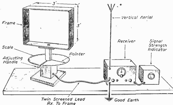
Fig. 6.—Layout for investigation of frame aerial properties. The pointer on the frame is set for cardioid working. The vertical aerial may be taken externally if the distance is not too great.
