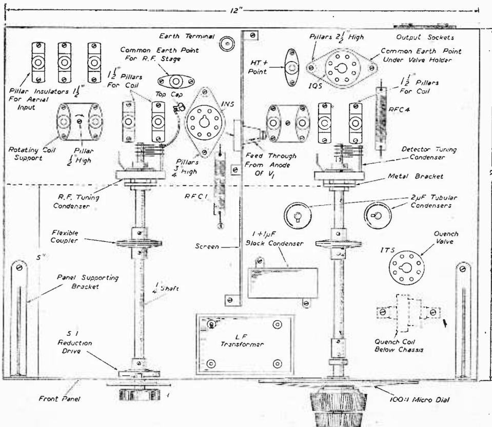
Fig. 2.—Layout of the chassis, and essential components.
