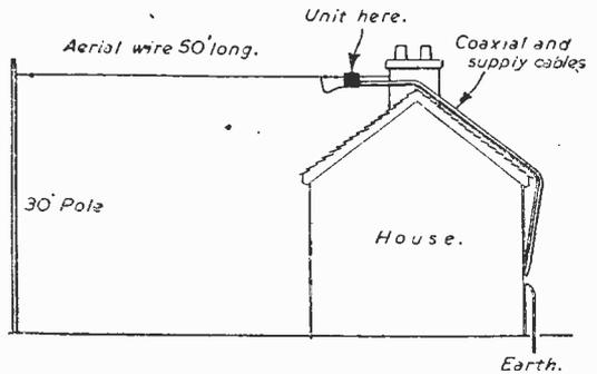
Fig. 5.—Diagram illustrating the complete Antistatic aerial layout.
