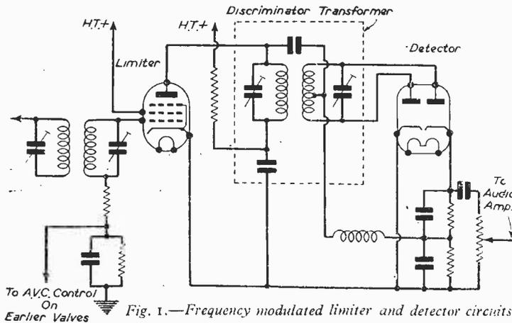
Fig. 1.—Frequency modulated limiter and detector circuits.
