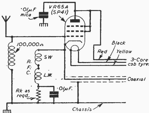
Fig. 2.—Theoretical Circuit of the aerial portion of the unit described here.
