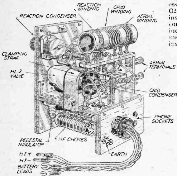
Fig. 1.—A general view of the completed receiver.
