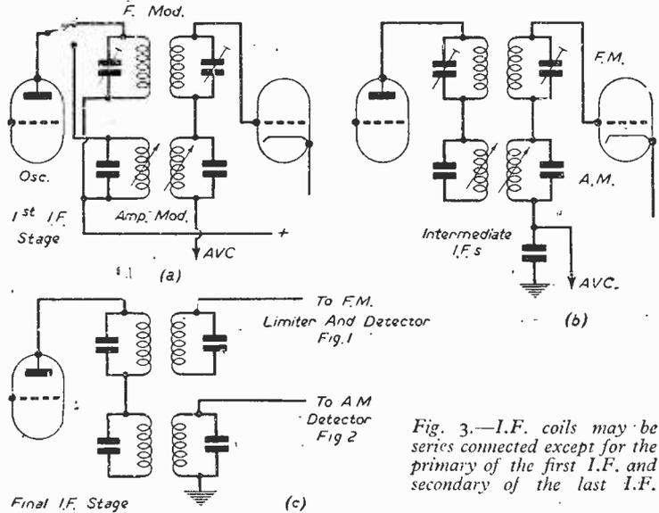
Fig. 3.—I.F. coils may be series connected except for the primary of the first I.F. and secondary of the last I.F.
