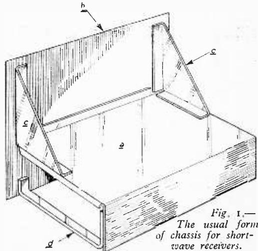
Fig. 1.—The usual form of chassis for short-wave receivers.
