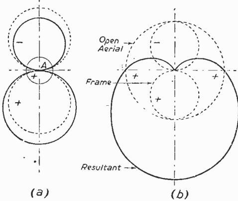
Fig. 4.—On the left are the combined open and frame aerial polar diagrams, and on the right the developed cardioid diagram.
