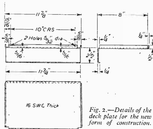
Fig. 2.—Details of the deck plate for the new form of construction.
