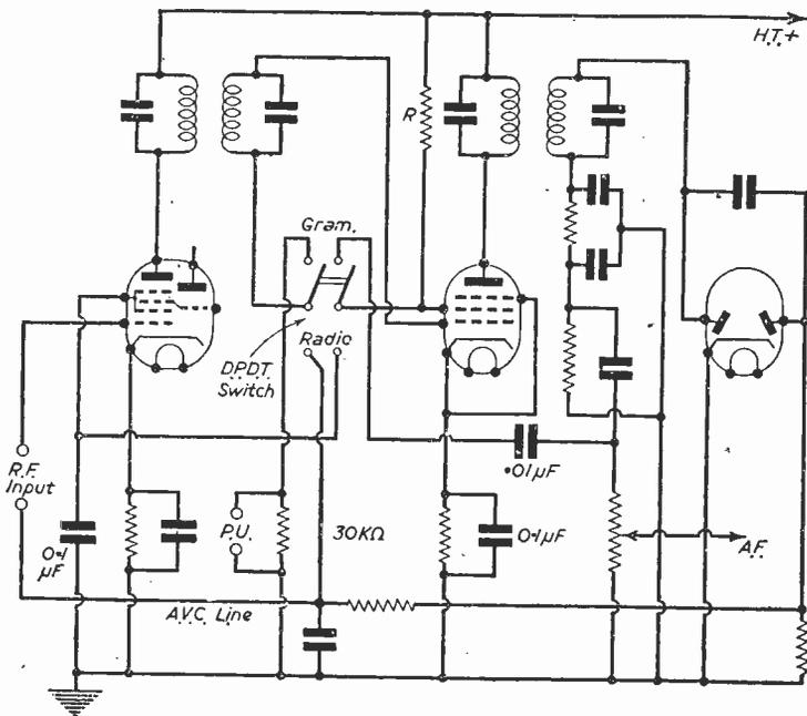
stages, and if the particular pick-up calls for some special form of control, this will have to be switched in when the receiver is switched over to 'gram. No doubt, this could be arranged by means of a ganged switch,
