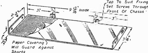
Fig. 11.—Note the use of a paper covering to avoid the risk of short circuits.
