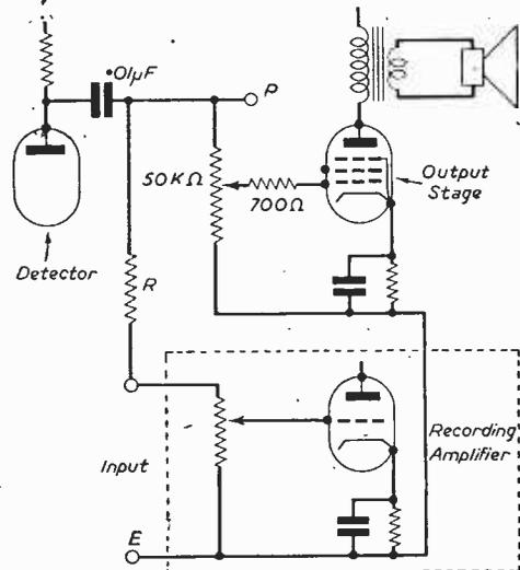
Fig. 3.—Coupling the circuit of Fig. 2 to the recording amplifier. Resistance R (250,000 ohms to 1 Megohm) provides high bridging-resistance and lowers the available AF voltage to that needed to load the recording amplifier.
