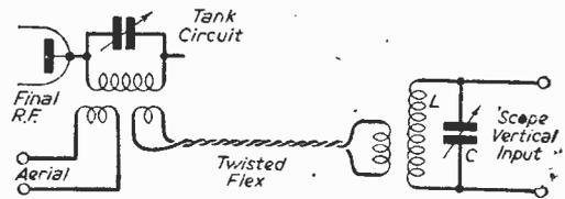
Fig. 11.—A method of eliminating transmitter harmonics.
