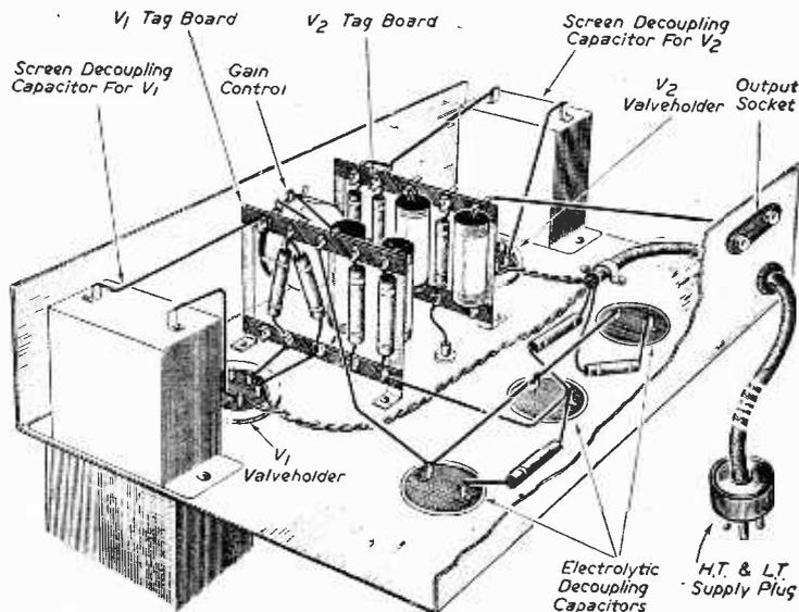
Fig. 4.—Underneath view of the suggested layout.
