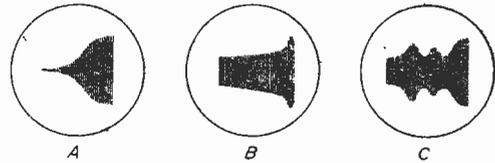
Fig. 14.—Other forms of distortion will show up as indicated here.
