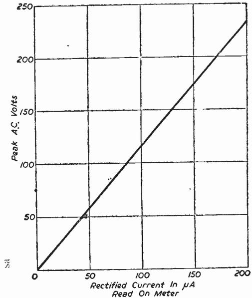
Fig. 2.—Typical calibration curve of the peak valve voltmeter.
