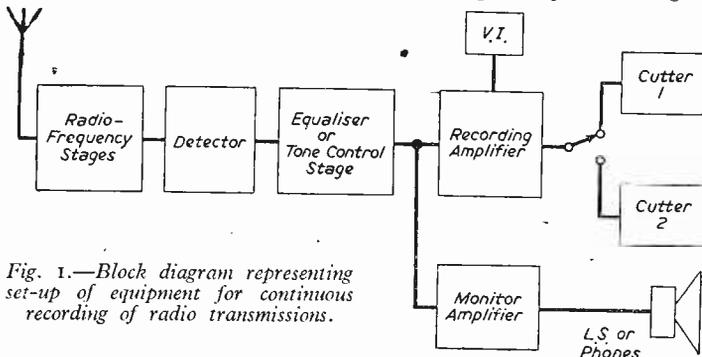
Fig. 1.—Block diagram representing set-up of equipment for continuous recording of radio transmissions.
