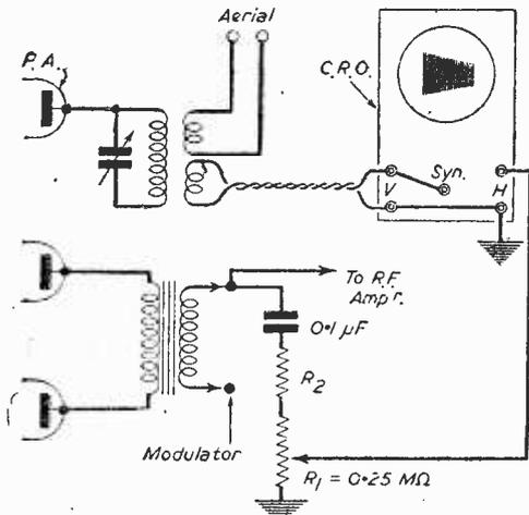
Fig. 12.—The Trapezoidal method of taking modulation oscillograms.
