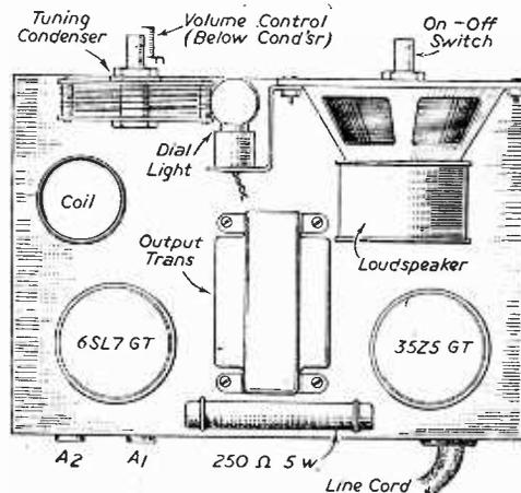
Fig. 2.—Layout of the receiver.
