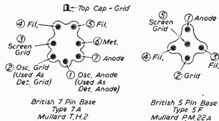
Fig. 12.—Valveholder pin connections as seen from the underside.
