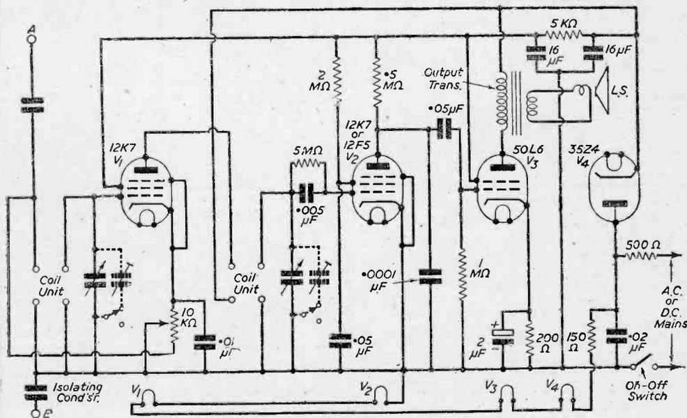
Fig. 1.—Theoretical circuit of the "Utility" Four.
