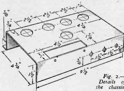
Fig. 2.—Details of the chassis.
