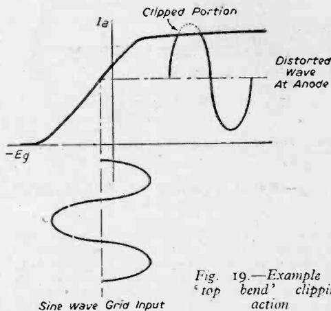
Fig. 19.—Example of 'top bend' clipping action
