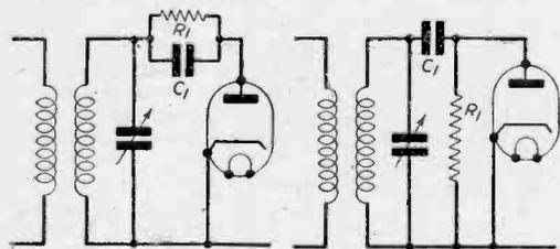
Fig. 1.—Fundamental circuit of series-fed diode detector.
