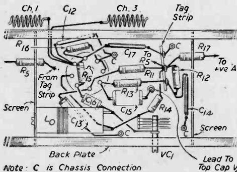
Fig. 4.—Layout of the frequency-changer stage. In this illustration the parts appear more spaced out than they are in practice.
