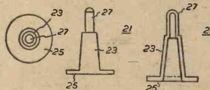
Figs. 2, 3 and 4.—Details of the vibration-eliminating sleeve.
