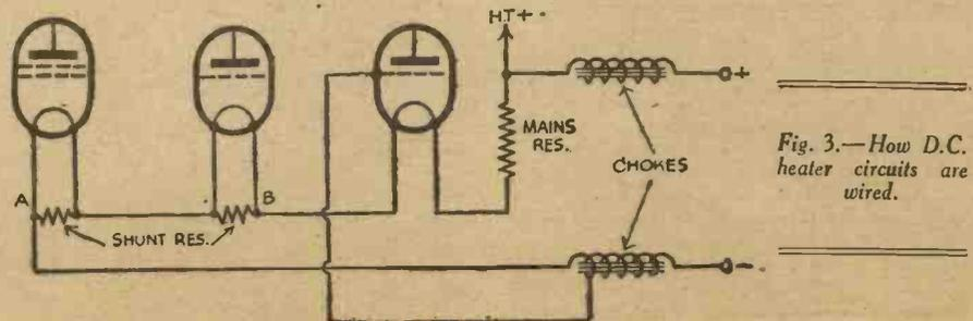
Fig. 3.—How D.C. heater circuits are wired.
