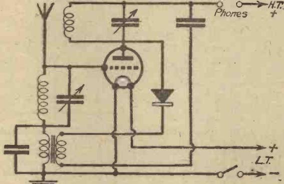
Fig. 4.—An early form of valve-crystal reflex circuit.
