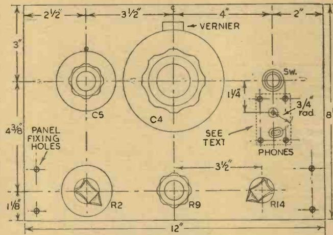
Fig. 3.—Panel layout and drilling diagram.
