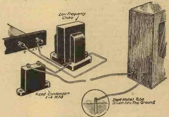
Method of connecting a loudspeaker when it is to be used at a distance from the set.
