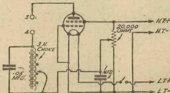
A modulated dynatron oscillator, which can be used with a tuner for wavelength checking, or for adjusting the trimmers in a set having ganged tuning condensers.
