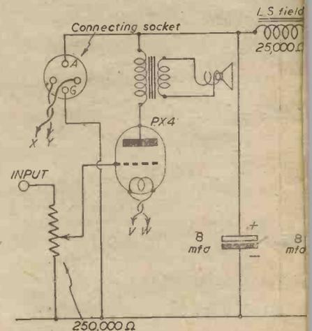
Fig. 5.—Alternative amplifier and power section circuit diagram.
