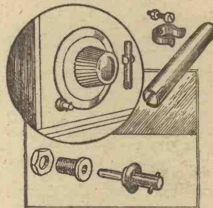
Details of a slow-motion remote control device.
