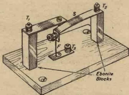
A novel switching arrangement for emergency lighting.
