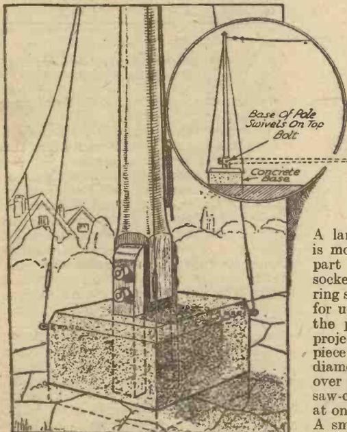
Method of mounting an aerial in a concrete block—the mast supports could project through the underside of the block and into the ground for some distance.—S. PARKER (Pinner).
