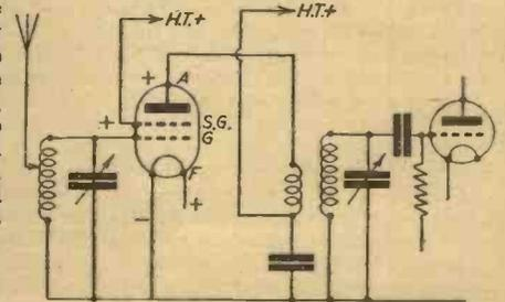
Note how the second grid is inserted in the S.G. valve.
