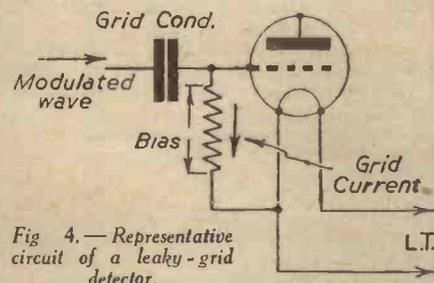
Fig. 4.—Representative circuit of a leaky-grid detector.
