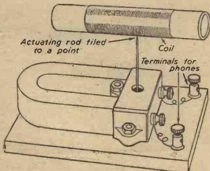
An improvised counter for fine coil windings.
