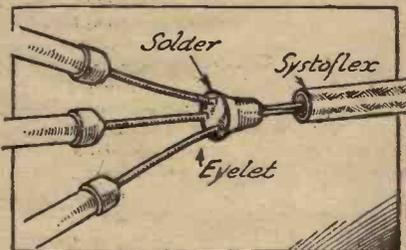
An effective method of making multiple connections.
