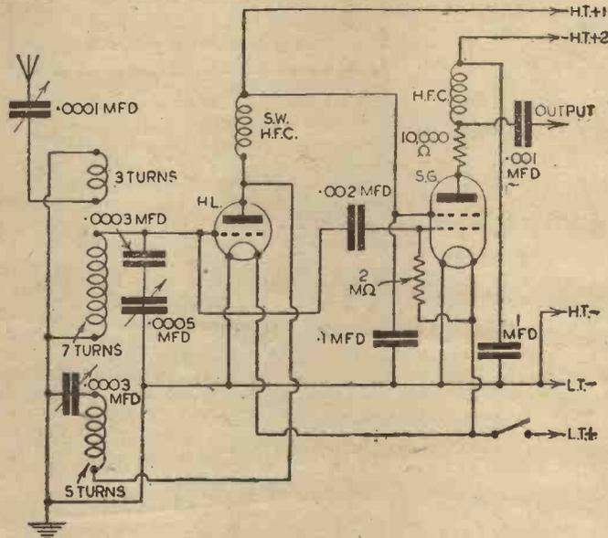
Circuit of a typical 2-stage S.W. superhet converter.
