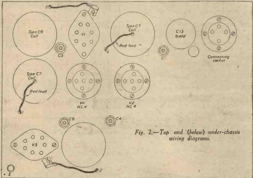
Fig. 2.—Top and (below) under-chassis wiring diagrams.
