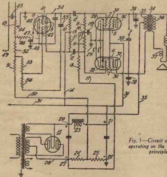
Fig. 1—Circuit of amplifier operating on the Class AB principle.
