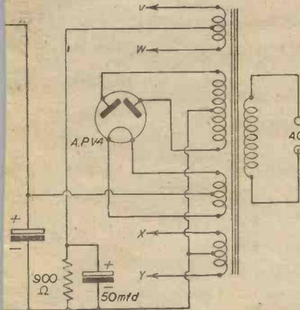
main section using a valve rectifier.
