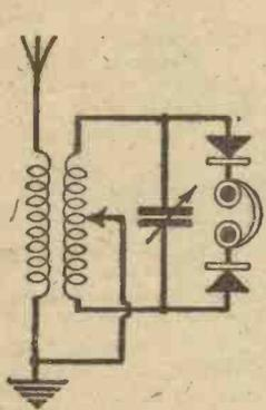
Fig. 2.—A crystal receiver using full-wave rectification.
