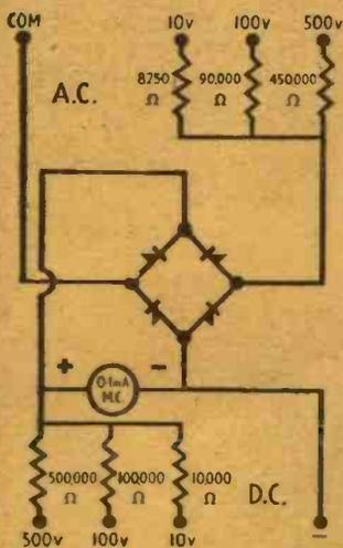
3. Descriptive pamphlet No. 11-B contains full details for the construction of a simple and robust A.C.-D.C. test set, suitable for reading D.C. and A.C. volts, and for measuring L.F. voltages in radio receivers. It also describes how the meter may be calibrated to read watts or decibels and also deals with the design of current transformers to enable high ranges of alternating current to be measured. Use the coupon and get your copy now
