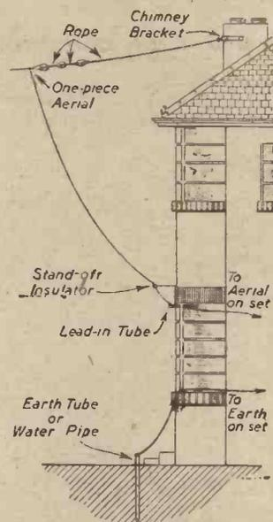
Fig. 2.—A neat and efficient inverted "L" type of aerial. Note the three insulators, continuous length of wire and good earth connection.
