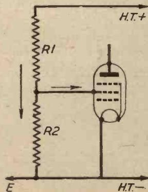
Fig. 2 (Left).—This simplified skeleton diagram shows more clearly the fixed potentiometer included in Fig. 1.
