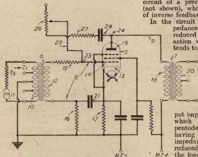
amplifier, the feedback connection would provide an input impedance considerably below that value without the use of the divider circuit comprising the resistors 27, 26 and 15. By choosing the resistor 15 of a proper value, such as 56,000 ohms,
