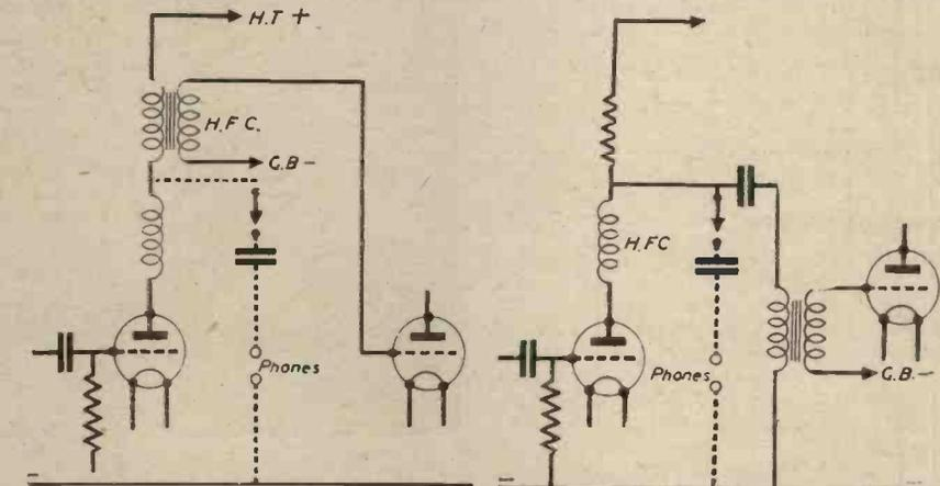
Fig. 2.—Showing how 'phones can be connected to intermediate stages. This procedure is better than connecting them in the output stage.
