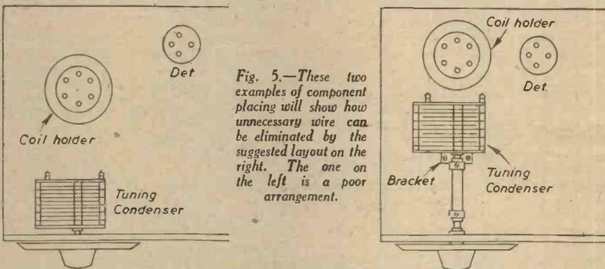
Fig. 5.—These two examples of component placing will show how unnecessary wire can be eliminated by the suggested layout on the right. The one on the left is a poor arrangement.
