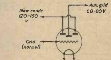
Fig. 4.—Method of utilising a double-diode valve to operate as a screened-grid valve.
