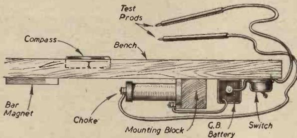
Details of a simple continuity testing apparatus.
