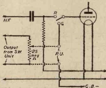
Fig. 5.—If the unit feeds into pick-up terminals a potentiometer is required as shown by broken lines.
