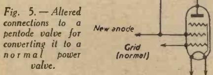
Fig. 5.—Altered connections to a pentode valve for converting it to a normal power valve.
