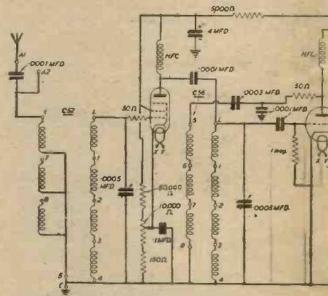
Theoretical circuit diagram of the A.C. Four-wave receiver, with some components omitted to avoid complications when
