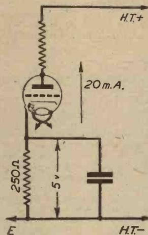
Fig. 4. — In this diagram figures are given to show the method of obtaining the value of a bias resistor wired in the cathode lead of an indirectly-heated valve.
