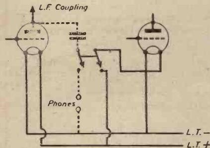
Fig. 3.—With battery sets it is often advisable to save L.T. current. The switching system shown cuts out the unwanted valve.
