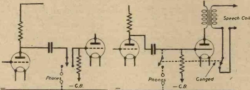
Fig. 4.—The loudspeaker becomes dead when the 'phones are brought into circuit when these forms of switching are used. The grid-leak must be returned to G.B.—or earth.
