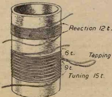
Fig. 2.—Details of the simple home-made coil.
