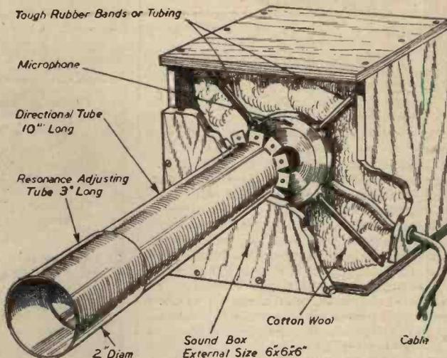
Fig. 2.—Part sectional view showing construction of sound box and directional resonator tube.
