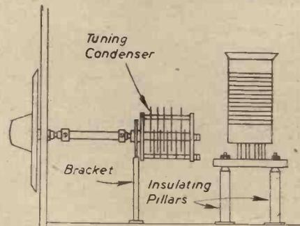
Fig. 4.—When good use is made of brackets at pillars, wiring can be simplified and efficiency increased.
