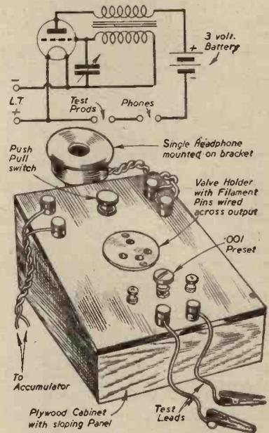
Circuit diagram and pictorial view of an easily-made oscillator unit.
