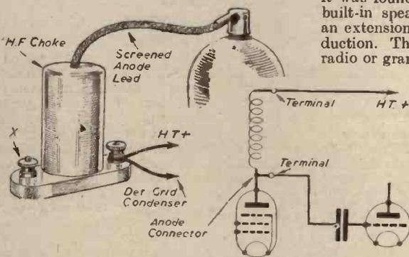
Fig. 2.—An H.F. Det.-L.F. receiver gave very poor results because the H.F. choke in the anode circuit of the H.F. valve was connected as shown. The inset diagram shows the proper connections.
