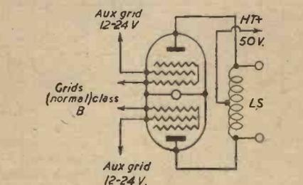
Fig. 6.—A novel modification of a Q.P.P. valve.
