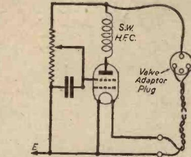
Fig. 4.—Connections when the unit is serving as an adapter.
