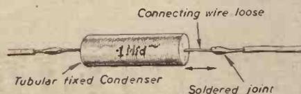
Fig. 1.—Intermittent crackling was traced to a loose wire connection on an S.G. by-pass condenser. The wire had been loosened by applying too much heat when making the soldered point.
