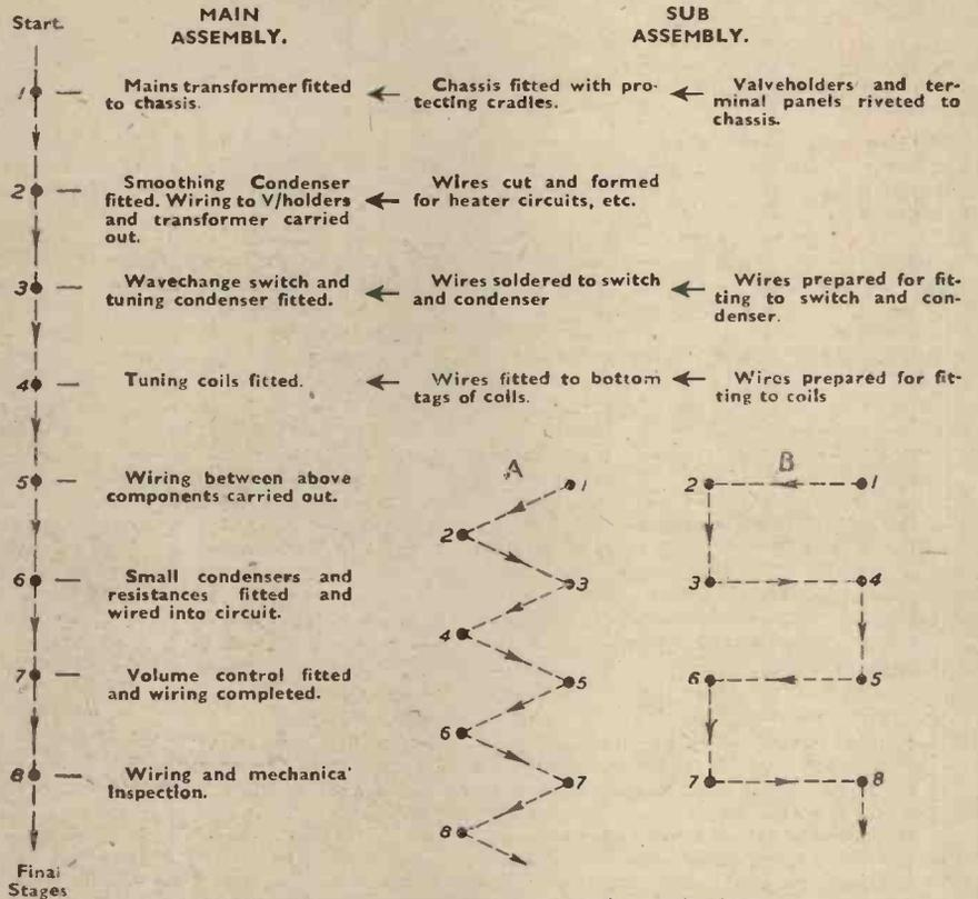
Assembly line chart of operations in a modern radio factory.
