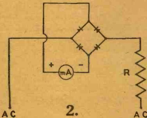
2. By adding a series resistance "R" the A.C. milliammeter is easily converted into an A.C. voltmeter. The value of "R" depends on the full scale reading required.
