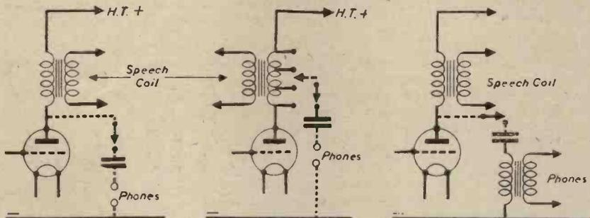
Fig. 1.—Three arrangements which enable headphones to be connected in the output circuit of a receiver. That on extreme right is the best for A.C./D.C. sets.
