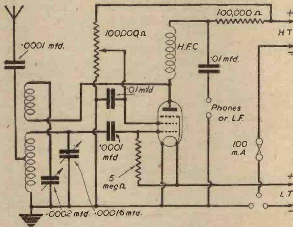
Fig. 1.—Circuit of the unit, suitable for use as a one-valve or in conjunction with an L.F. amplifier.
