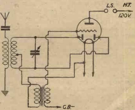
Fig. 7.—Method of modifying a double-diode-triode valve.
