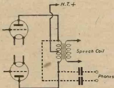
Fig. 5.—A simple method suitable for use with Class A, Class B, or Q.P.P. push-pull circuits.
