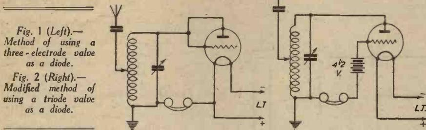
Fig. 1 (Left).—Method of using a three-electrode valve as a diode.
