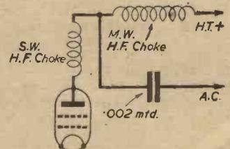
Fig. 3.—Modified anode connections when using the unit as a superhet converter.
