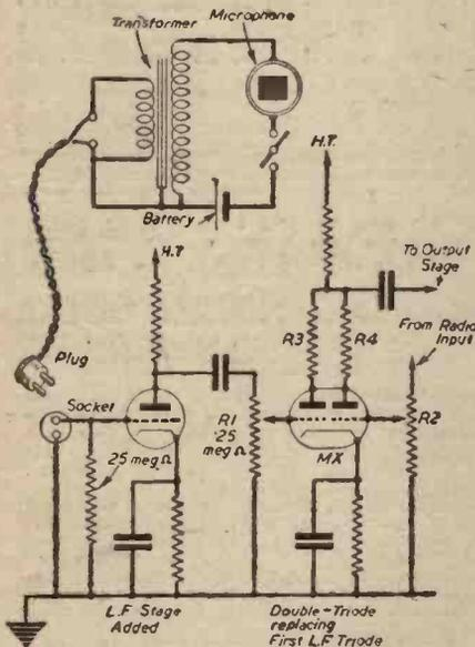
Fig. 1.—Circuit diagram of the complete apparatus. R3 and R4 are each twice the A.C. resistance of a single triode.
