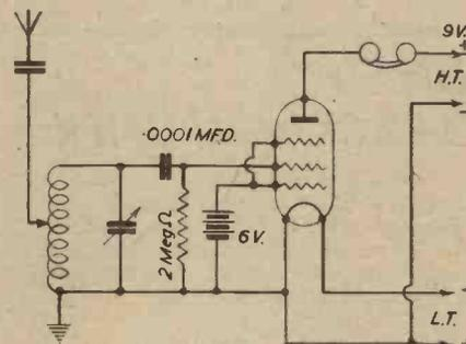
Fig. 3.—Using a pentode as a four-electrode valve.
