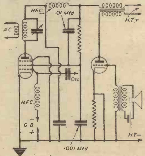
Fig. 6.—Combined anode and screen modulation of an R.F. pentode. The two condensers in the screen circuit form an A.F. potentiometer; values assigned are very approximate.
