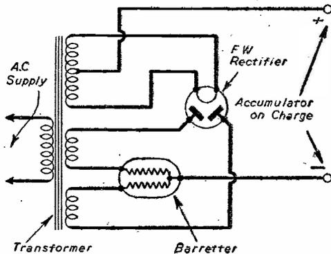
Fig. 2.—Typical circuit for battery charging.
