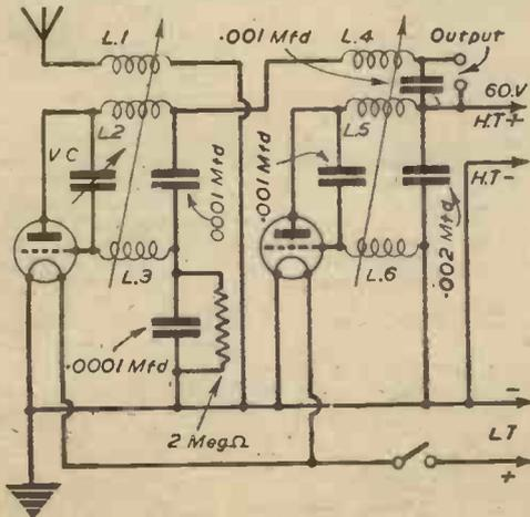
Fig. 1.—Quench-operated circuit for U.H.F.
