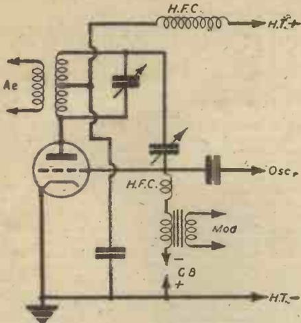
Fig. 3.—A grid-bias-modulated R.F. amplifier.
