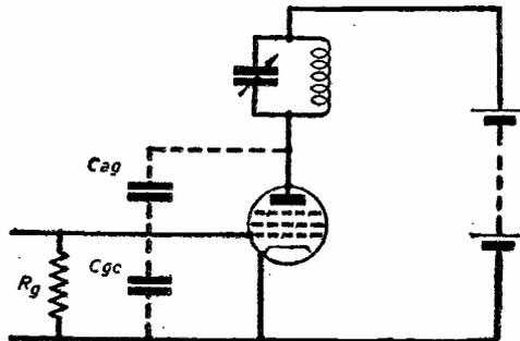
Fig. 3.—Method of varying the applied frequency.
