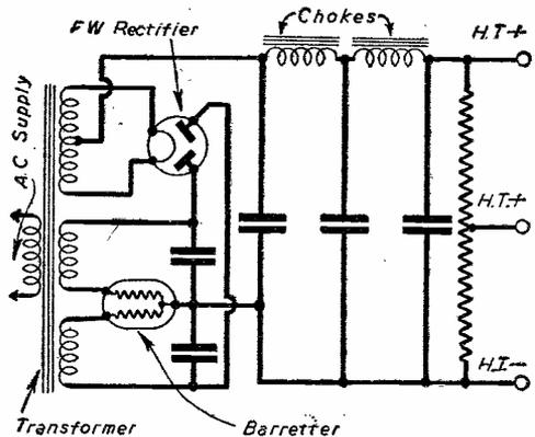
Fig. 3.—Circuit for H.T. supply of battery receiver.
