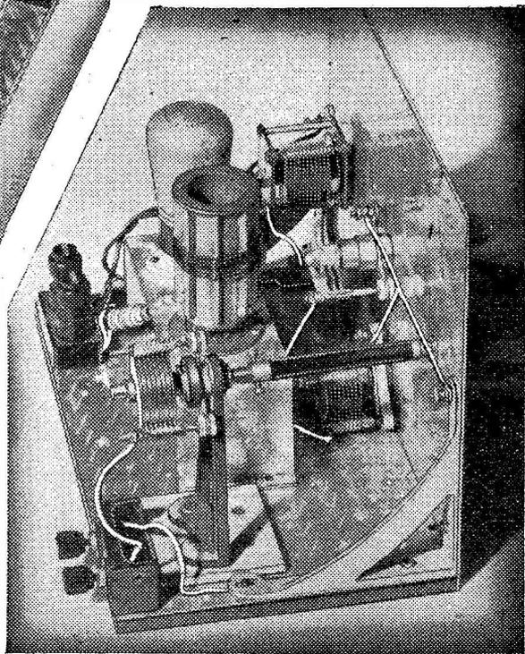
*Figs. 1 and 2.—Two views of the DX 1-valver.*
