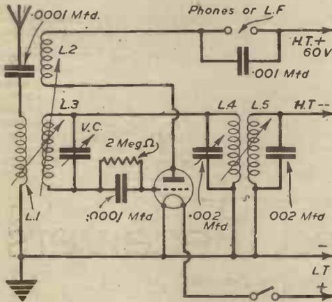
Fig. 3.—Single valve quench-operated receiver.
