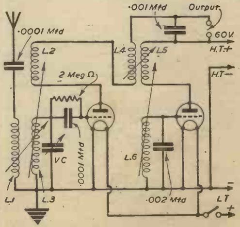
Fig. 2.—Circuit for short and medium waves.
