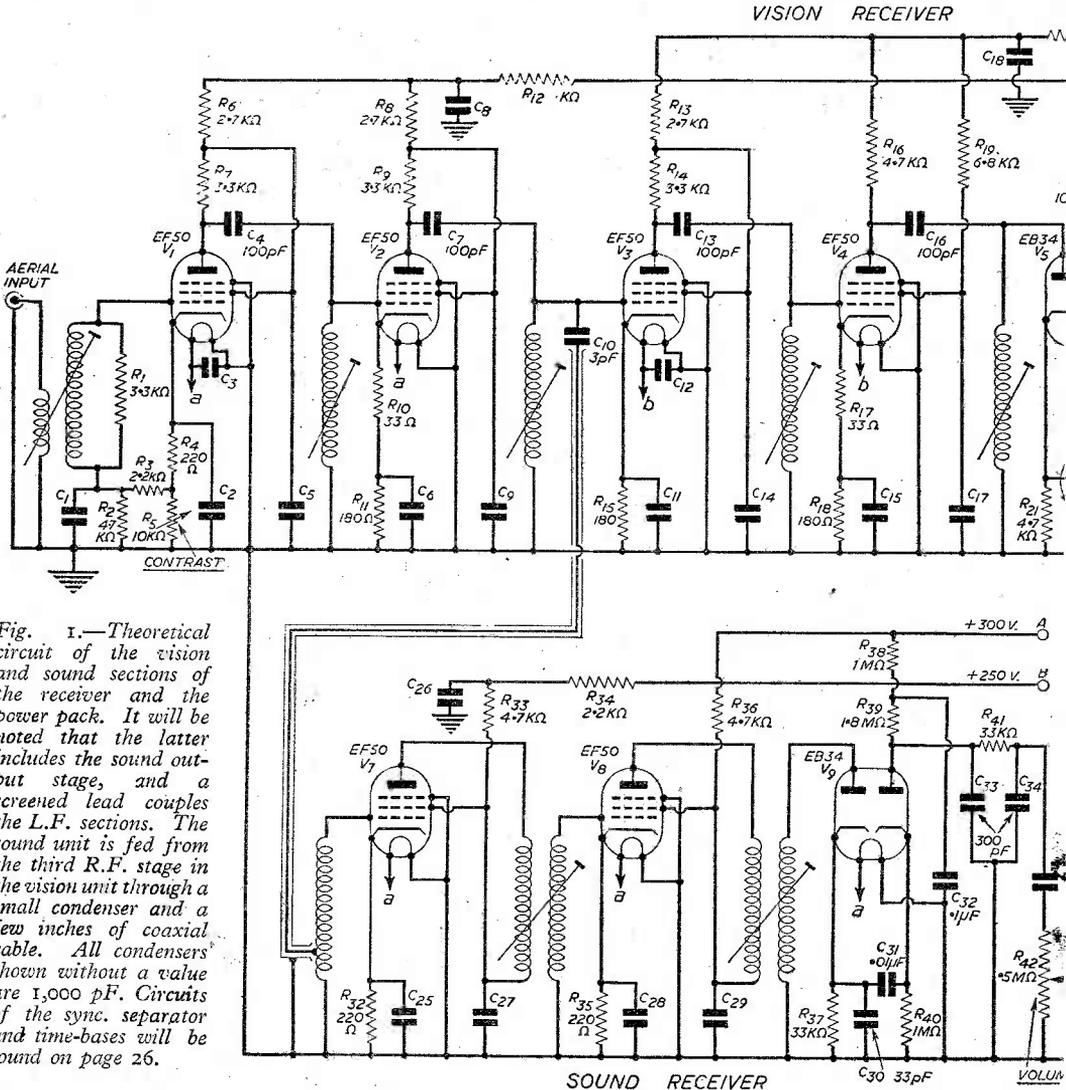
*Fig. 1.—Theoretical circuit of the vision and sound sections of the receiver and the power pack. It will be noted that the latter includes the sound output stage, and a screened lead couples the L.F. sections. The sound unit is fed from the third R.F. stage in the vision unit through a small condenser and a few inches of coaxial cable. All condensers shown without a value are 1,000 pF. Circuits of the sync. separator and time-bases will be found on page 26.*
