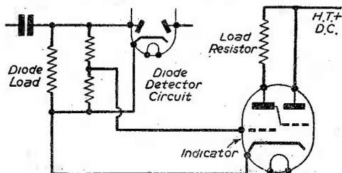
Fig. 4.—Another circuit with diode control.
