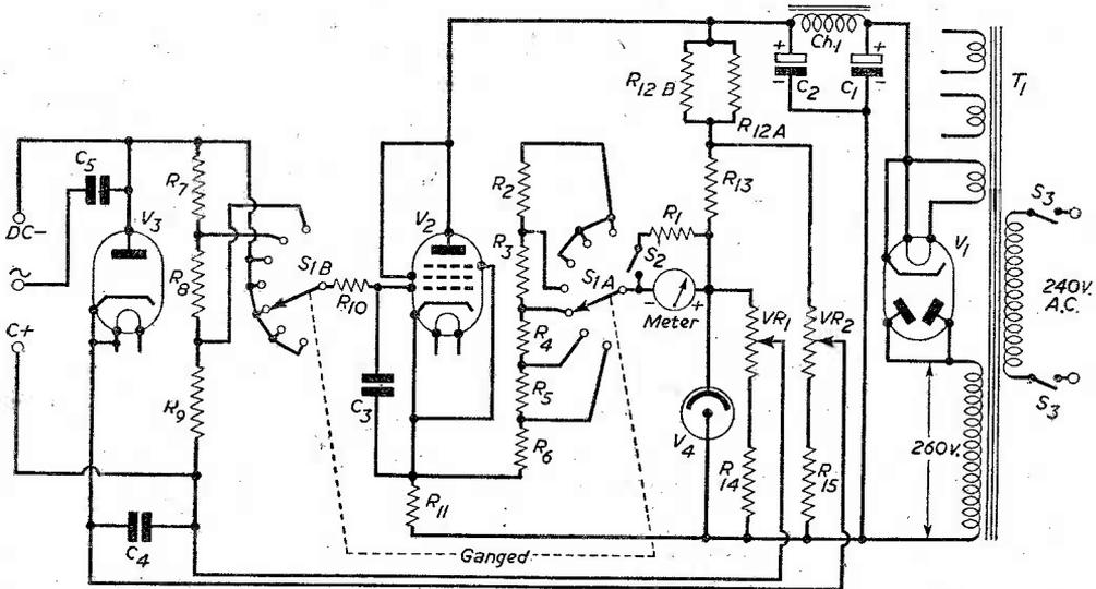
Fig. 1.—Theoretical circuit of the valve voltmeter. The neon must be connected the right way round to ensure stability—that is, with cathode earthed.
