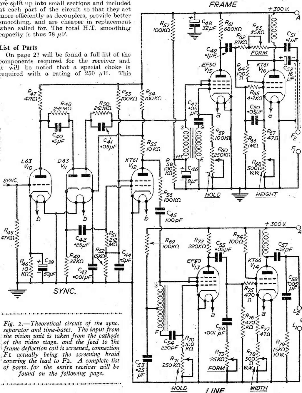
Fig. 2.—Theoretical circuit of the sync. separator and time-bases. The input from the vision unit is taken from the cathode of the video stage, and the feed to the frame deflection coil is screened, connection F1 actually being the screening braid covering the lead to F2. A complete list of parts for the entire receiver will be found on the following page.
