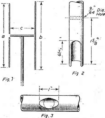
Fig. 1.—Standard "H" aerial with main measurements indicated. Fig. 2.—The lower ends of the aerial are cut as shown here. Fig. 3.—Centre of the cross piece.
