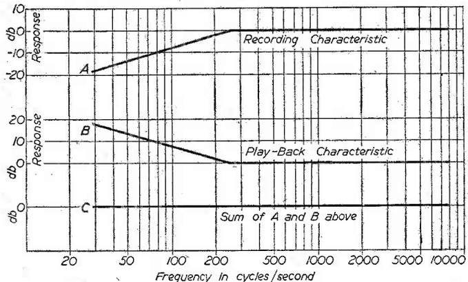
Fig. 2.—Method of correcting for recording loss at bass frequencies.
