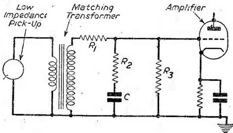
Fig. 4.—Simple bass-correction circuit that can be designed to give boost at 6 db per octave up to any desired frequency. See text for the design formula.
