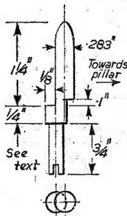
Fig. 27.—Details of the record centre support. This fits into the top of the turntable centre spindle and supports the records until they are released.
