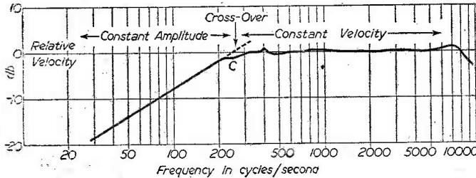
Fig. 1.—Response/frequency characteristics of disc recorder head. Note the cross-over at 250-300 c.p.s.
