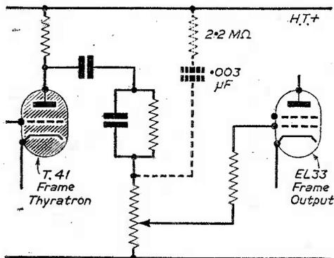
Fig. 3.—Modification to the frame time-base circuit to correct for non-linearity of the frame scan.
