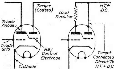
Fig. 1.—Essential parts of the tuning indicator. Fig. 2. (right)—Standard circuit showing how the indicator functions.
