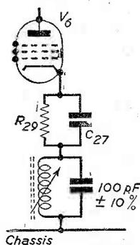
Fig. 1. — The sound trap is included in the cathode lead of the last I.F. valve.
