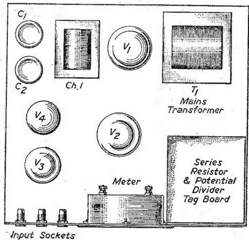
Fig. 3.—Chassis layout.
