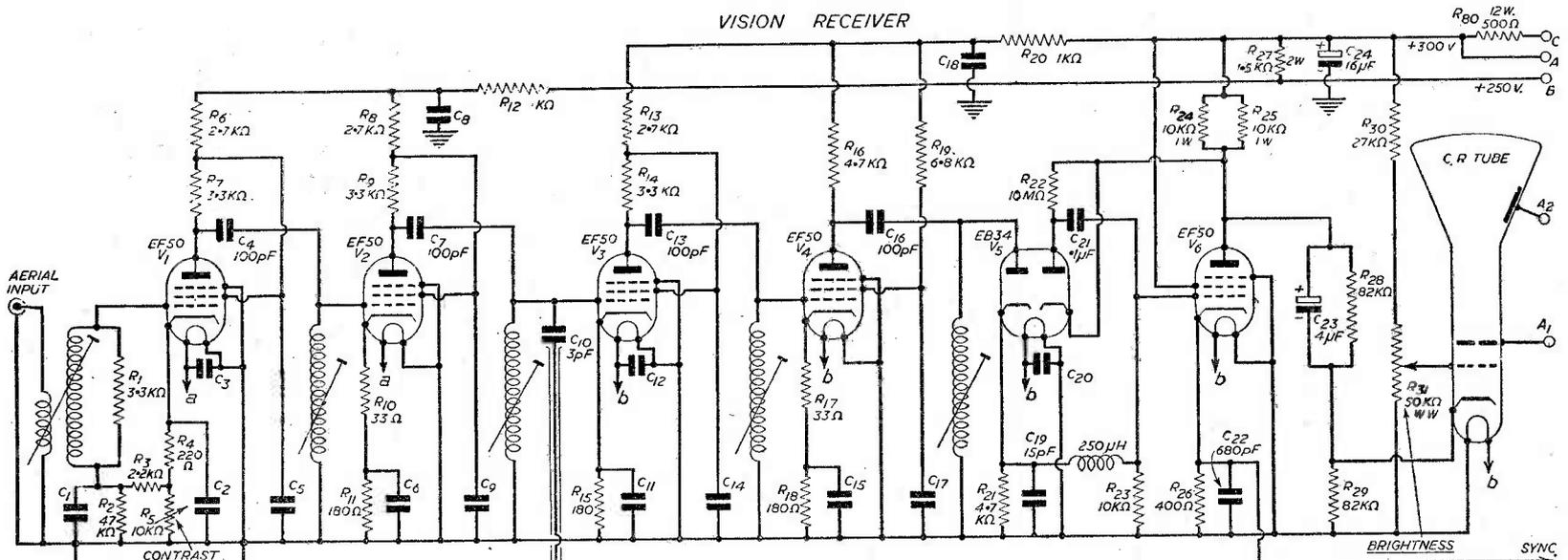
Fig. 1.—Theoretical circuit of the vision and sound sections of the receiver and the power pack. It will be noted that the latter includes the sound output stage, and a screened lead couples the L.F. sections. The sound unit is fed from the third R.F. stage in the vision unit through a small condenser and a few inches of coaxial cable. All condensers shown without a value are 1,000 pF. Circuits of the sync. separator and time-bases will be found on page 26.
