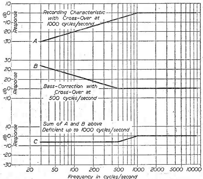
Fig. 3.—Showing the effect of play-back with the wrong bass-correction characteristic.
