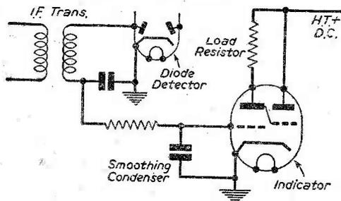
Fig. 5.—In this circuit delayed A.V.C. is utilised.
