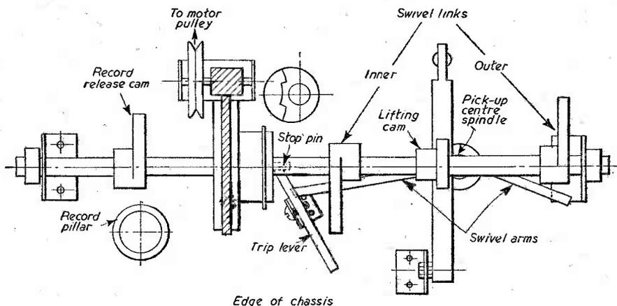
Fig. 31.—General view of the layout of the parts on the main spindle. As shown, the mechanism is in the "stop" position, with the pick-up on the edge of the record.
