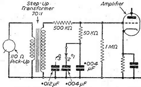
Fig. 5.—The circuit of Fig. 4 modified to give any of three characteristics. Boost is available for cross-over frequencies of 250, 500 or 1,000 cycles/second.
