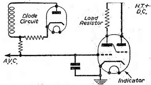
Fig. 3.—Typical indicator connected to the A.V.C. line.
