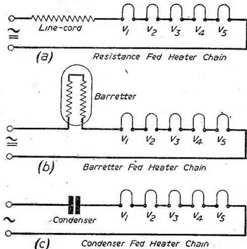
Fig. 1.—The basic feed methods for a series heater chain.
