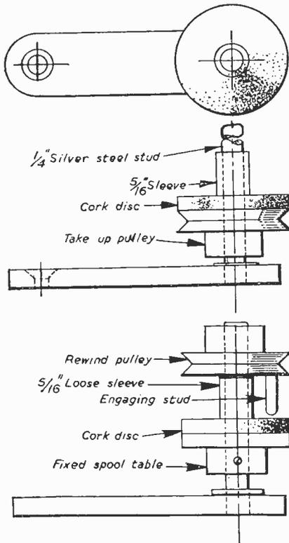
Fig. 3.—The feed-spindle with rewind pulley.
