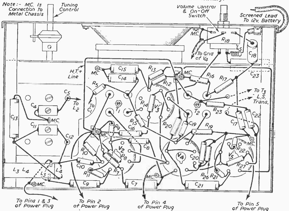
Fig. 8.—Wiring details of the main receiver portion.
