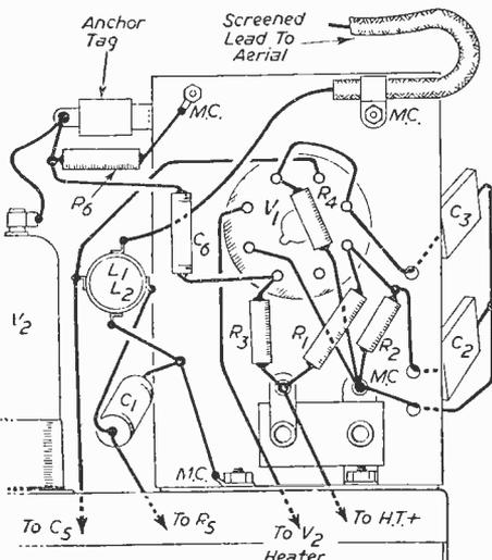
Fig. 10.—Wiring of underside of V1 platform.
