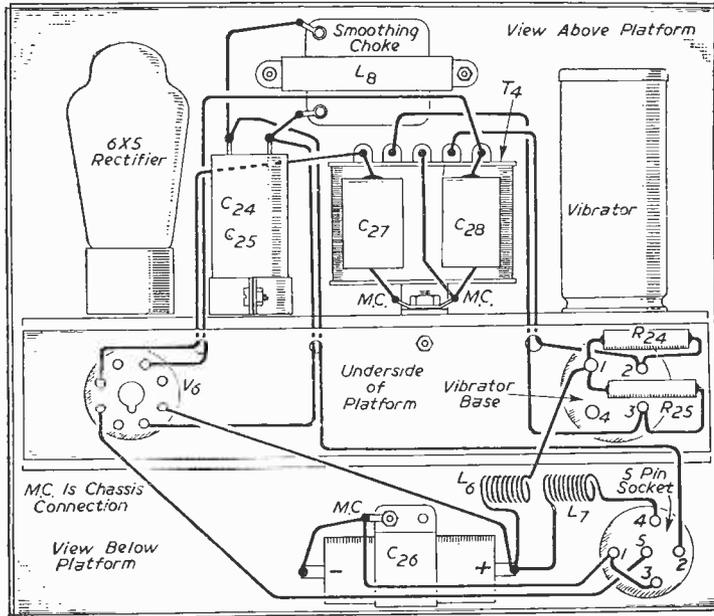
Fig. 9.—Wiring details of the power pack.
