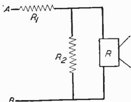
Fig. 1.—Normal output circuit in theoretical form.
