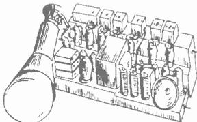
**SOUND, VISION, TIME BASES, POWER PACK AND SPEAKER ON ONE 1355 CHASSIS:** Absence of expensive RF units, an absolute minimum of extra parts, and its remarkably
