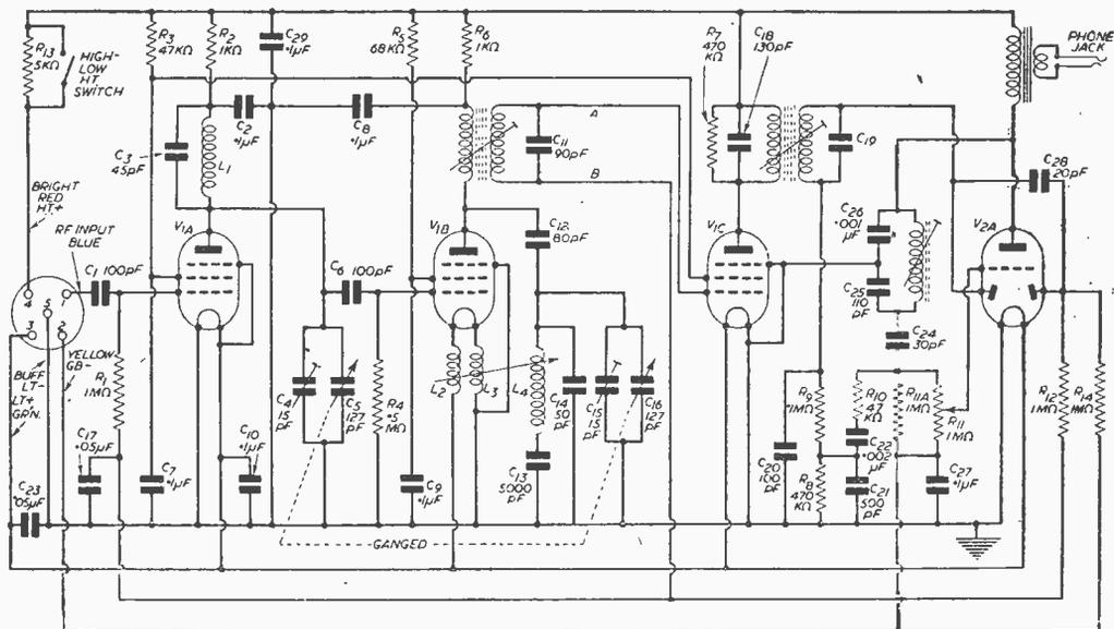
Fig. 1.—Circuit of the WS18 (popularly known as Type 18) receiver before modification.
