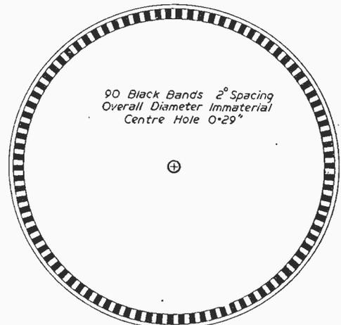
Fig. 1.—Laying out a Stroboscope for a turntable running at  $33\frac{1}{3}$  r.p.m. under lighting from 50 cycles mains.
