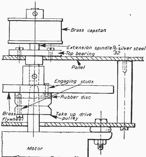
Fig. 6.—Method of fitting extension spindle and flywheel.
