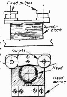
Fig. 4.—The recording head is mounted in a clamp made up from two strips of brass as shown in this plan and elevation.
