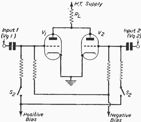
Fig. 1.—Basic Electronic Switch Circuit.
