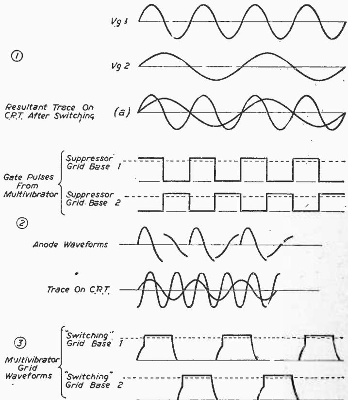
Fig. 2.—Waveforms associated with electronic switch circuits. (Not to scale.) (1) Simple circuit. (2) Gate circuit. (3) Triode-Hexode (anode wave-forms as in (2)).
