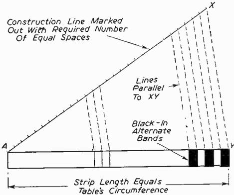
Fig. 2.—Diagram shows method of constructing a stroboscope for the rim of a turntable.
