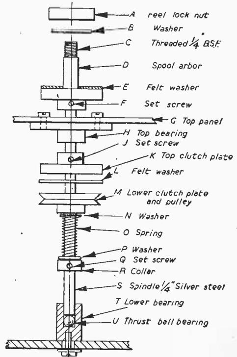
Fig. 7.—Full details of the take-up spindle.
