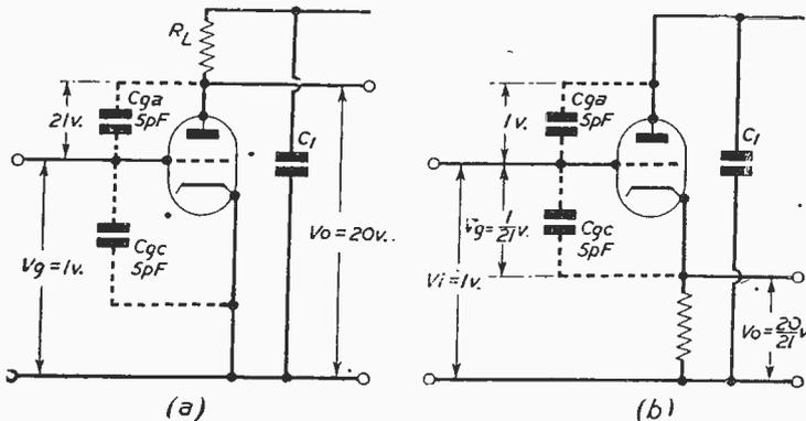
Fig. 9—A non-feed-back amplifier stage showing the stray capacities and their effect.
