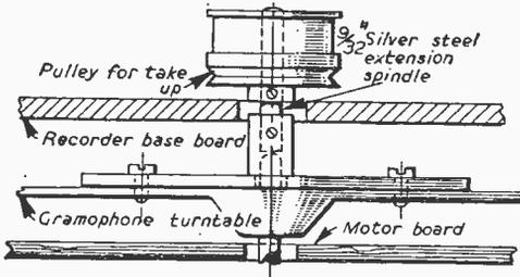
Fig. 1.—Method used to extend spindle of motor in the first recorder.
