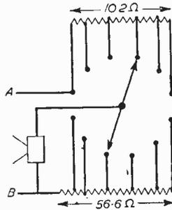
Fig. 3.—Wiring the resistances to a double-pole switch.
