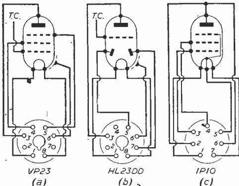
Fig. 4.—Base connections for the three valve types.
