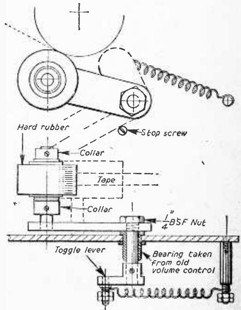
Fig. 2.—The pressure roller with toggle action.
