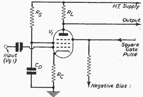
Fig. 3.—Basic "Gate" Circuit.
