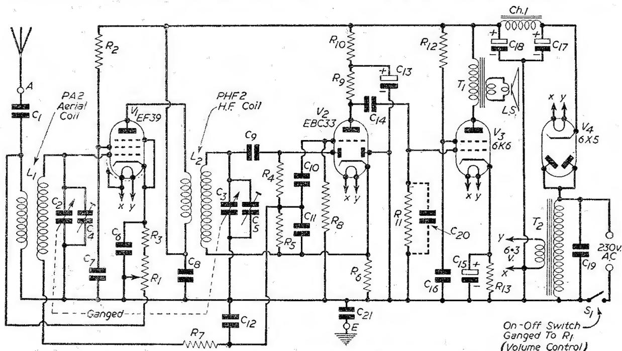
Fig. 1.—Theoretical circuit of the Quality Straight Three.
