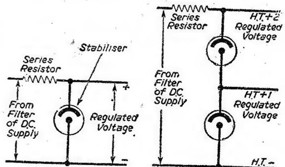
Fig. 1.—Circuit of straightforward stabiliser circuit.
