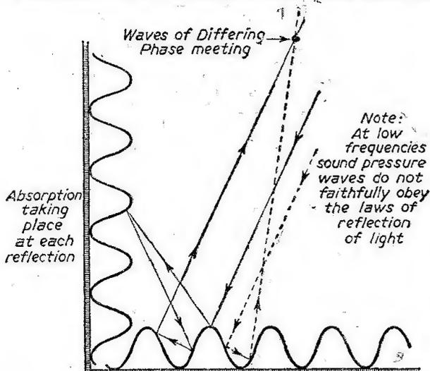
Fig. 2.—Part cross-section of lined cabinet showing possible paths of sound waves from loudspeaker.
