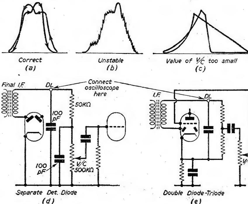
Fig. 6.—A.F. testing, showing typical oscillograms.
