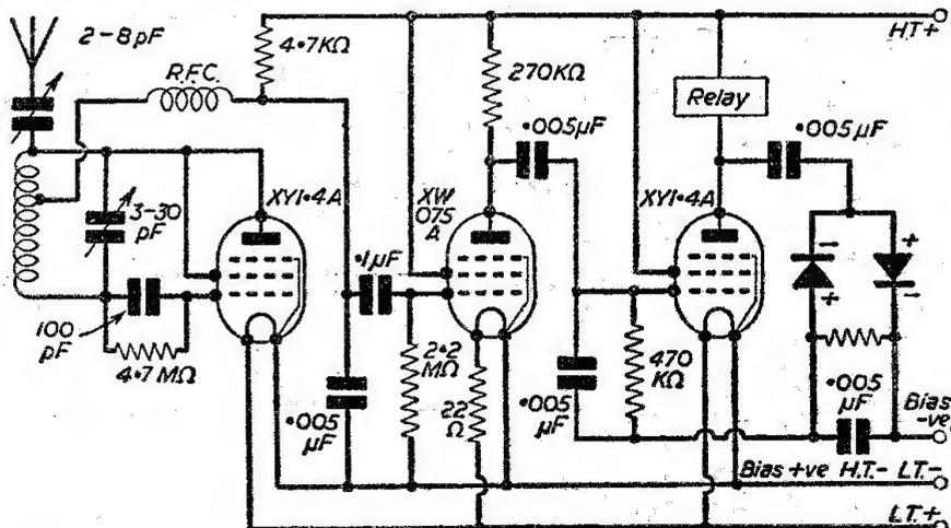
Fig. 3.—Three-valve receiver circuit with the tone-operated A.F. stage.
