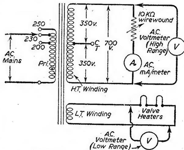
Circuit of a typical Mains Transformer and method of testing.
