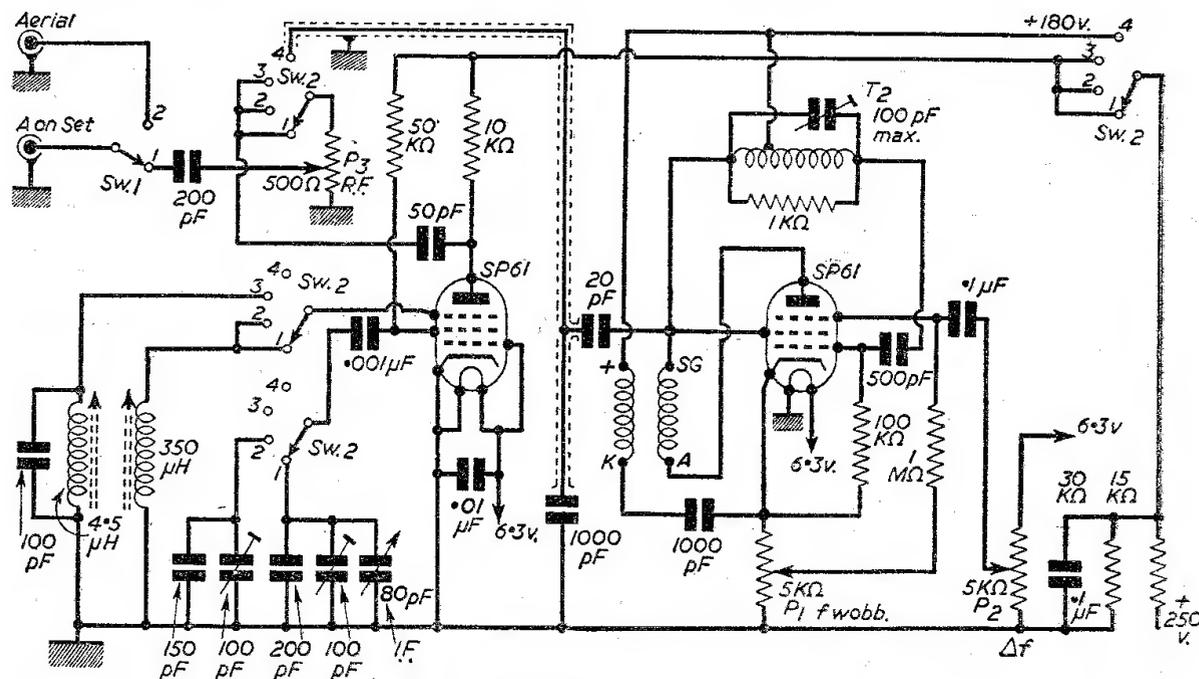
Fig. 1.—Circuit of the wobulator section.
