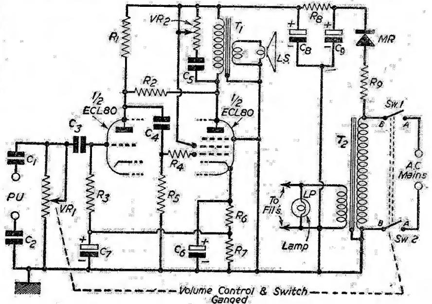
Fig. 1.—Theoretical circuit of the amplifier.
