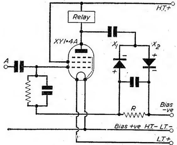
Fig. 2.—Final circuit of the A.F. stage.
