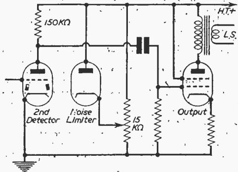
Fig. 2.—Simple clipper circuit.
