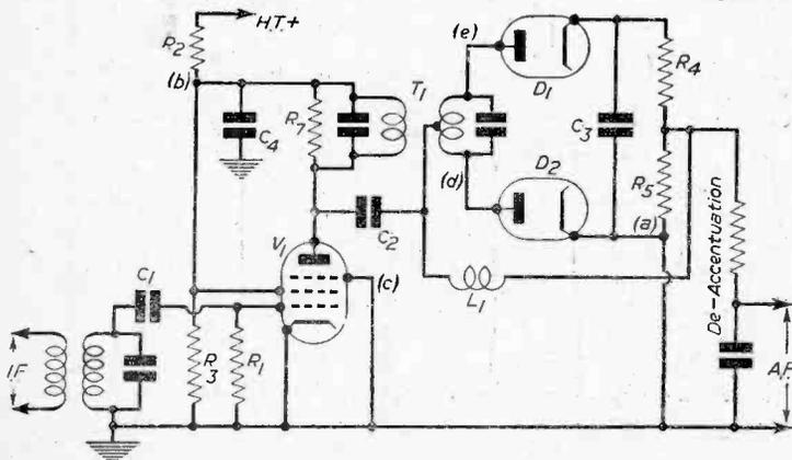
Fig. 17.—A frequency demodulator consisting of an amplitude limiter and a phase discriminator.
