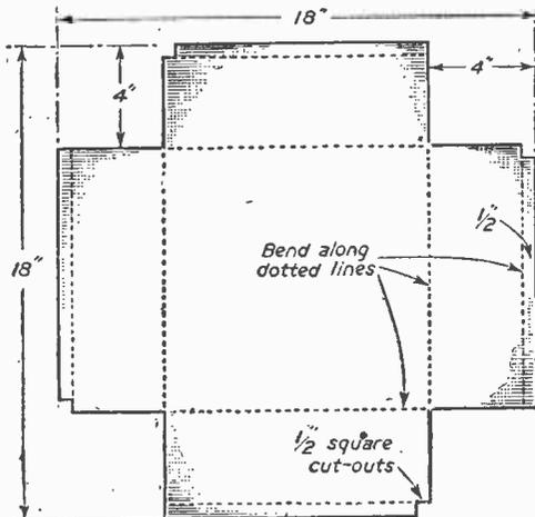
Fig. 2.—Details of the chassis.
