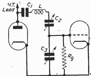
Fig. 14.—A series circuit as referred to on the following page.
