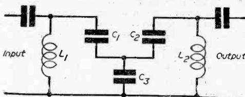
Fig. 16.—An I.F. transformer using mutual capacitance instead of mutual inductance coupling. The high frequency hump is tuned by means of C1 and C2 while the low frequency hump by means of C3.
