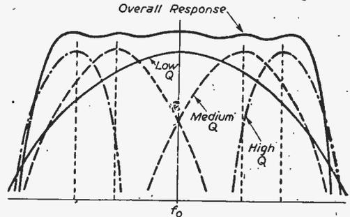
Fig. 15.—The combined effect of a number of stagger-tuned circuits.
