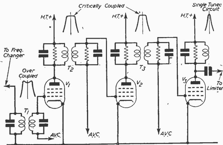
Fig. 15.—The functional circuit of a wide band I.F. amplifier for F.M. reception. An approximate shape of the frequency response curve is outlined above each stage of tuning.
