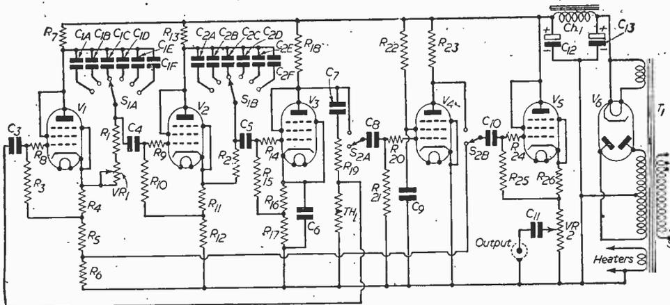
Fig. 1.—Theoretical circuit of the oscillator.
