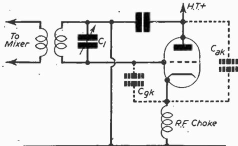
Fig. 14.—The modified Colpitts oscillator circuit—suitable for use as the local oscillator of a V.H.F. receiver. The anode is effectively earthing at R.F. so that  $C_1$  may form part of a two- or three-gang variable capacitor.
