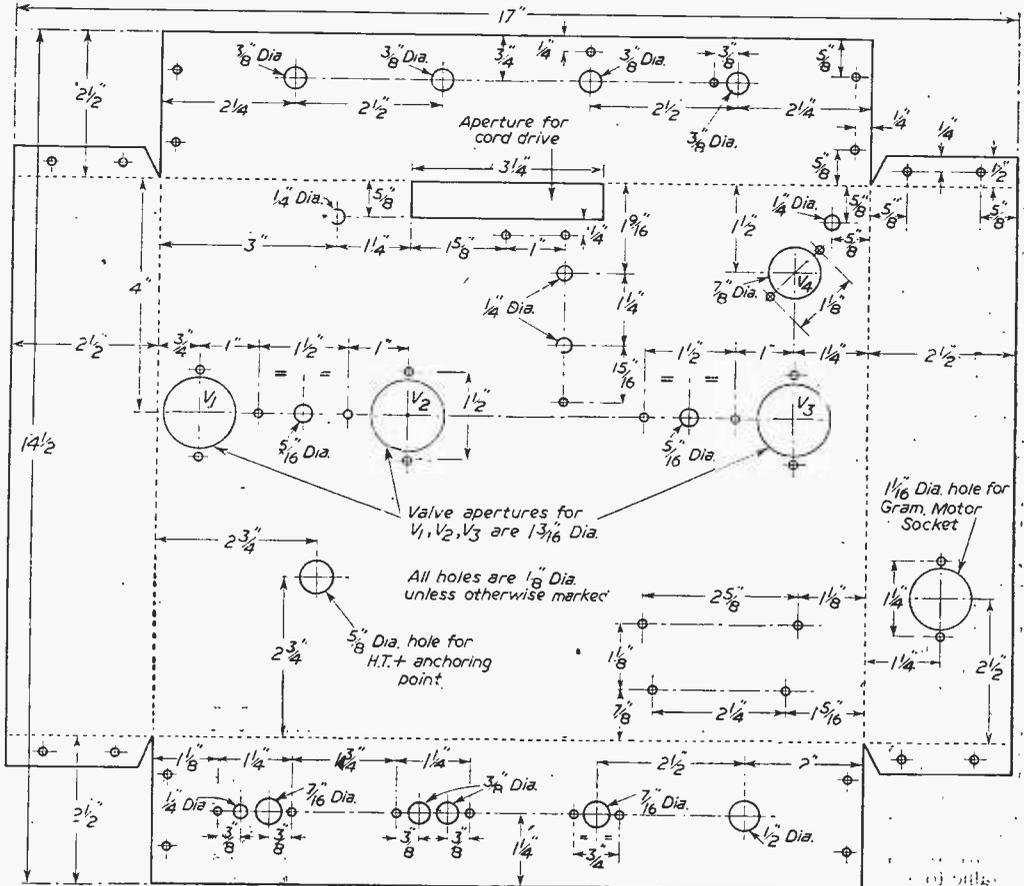
*Drilling details for the tuner and pre-amplifier chassis.*
