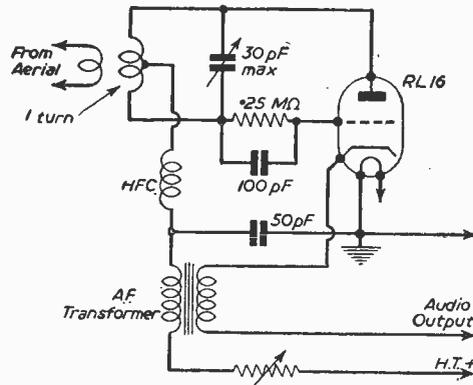
Fig. 53.—One form of super-regenerative circuit.
