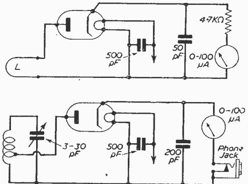
Fig. 56 (above).—V.H.F. valve voltmeter, and Fig. 57 (below).—A wavemeter for V.H.F. work.
