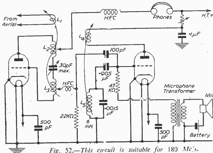
Fig. 52.—This circuit is suitable for 180 Mc/s.
