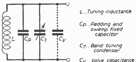
Fig 1.—V.F.O. tuned circuit.
