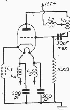
Fig. 46.— $L_2$ ,  $L_3$  and  $L_5$  are all H.F. chokes, consisting of 5-10 turns on a  $\frac{1}{2}$  in. former.
