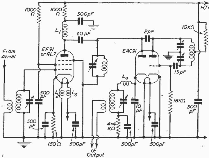
Fig. 54.—Another self-quenched super-regenerative arrangement.
