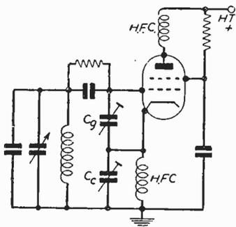
Fig. 7.—Condenser tap version of the "electron-coupled" oscillator. This is not to be confused with the similar Clapp circuit.  $C_2$  and  $C_3$  are cathode tapping condensers of, say, 100 pF. and 500 pF., respectively.
