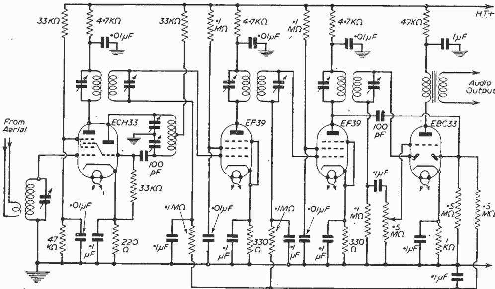
Fig. 48.—H.F. end of a complete receiver.
