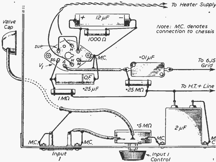
Fig. 2.—Wiring diagram of the 6J7 stage.
