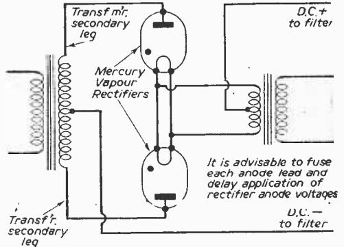
Fig. 1.—Basic circuit of a rectifier unit.
