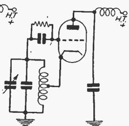
Fig. 4.—The grounded anode Hartley (so-called "electron-coupled" oscillator).
