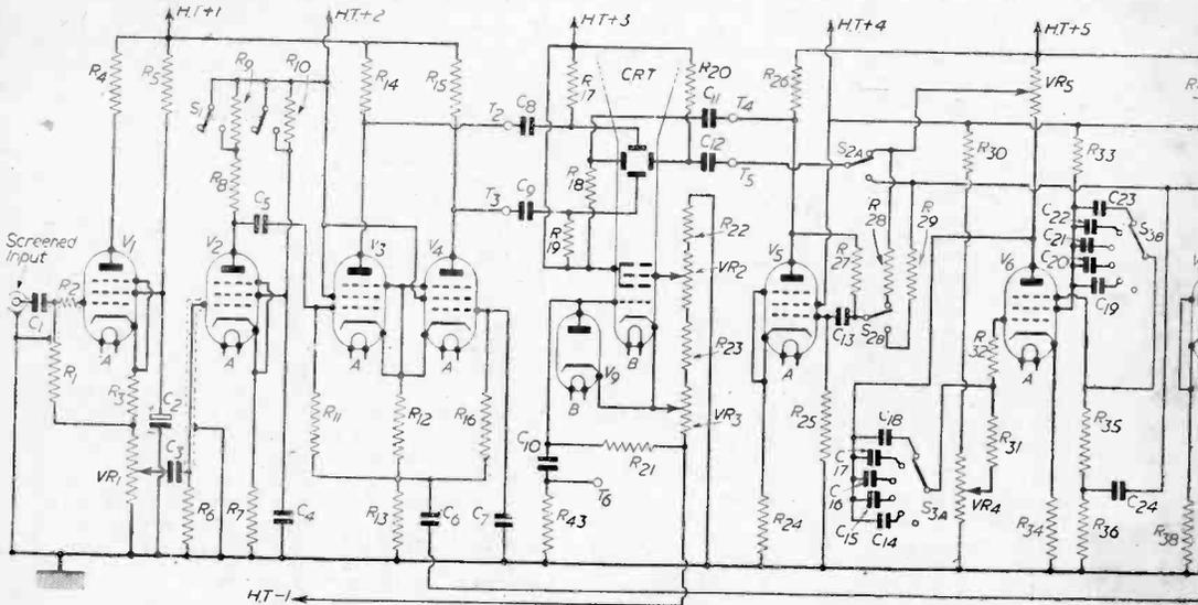
Fig. 1.—Theoretical circuit of the Versatile Oscilloscope.
