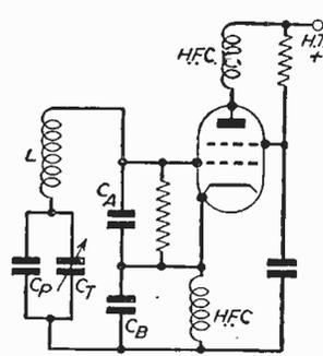
Fig. 9.—Clapp oscillator. Total effective tuning capacity is approximately  $C_T$  plus  $C_T$ , which may be, say, 35 pF or less.  $C_A = C_B$  which may be 500 pF. to 1,000 pF.
