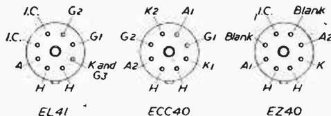
Note: I.C. is internal connection of valve. The tag can not be used for anchoring purposes
