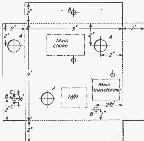
Fig. 12.—Drilling and cutting data for the amplifier chassis.
