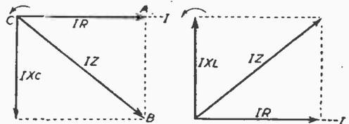
Fig. 2. (Left)—Showing how the voltage  $IX_c$  across a condenser lags the current by an angle of 90 deg.
