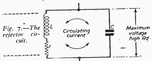
Fig. 7.—The rejector circuit.
