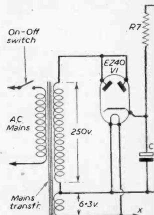
Fig. 1.—Theoretical circuit.
