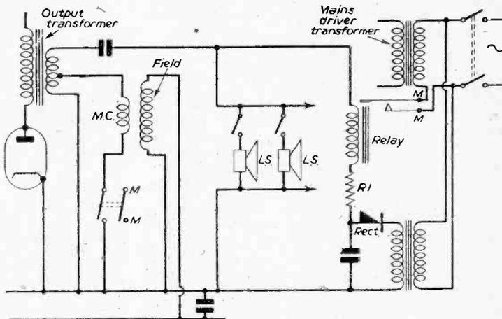
Circuit diagram of the remote control system.
