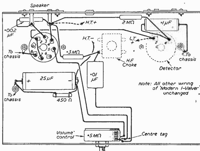
Components and wiring for the L.F. stage.
