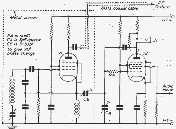
Fig. 1.—Basic N.B.F.M. V.F.O.-reactance modulator circuit.
