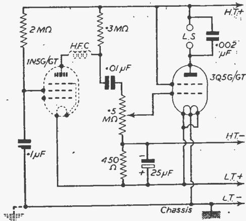
Theoretical circuit, showing additional wiring.
