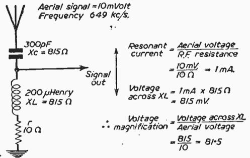
Fig. 6.—The acceptor circuit.
