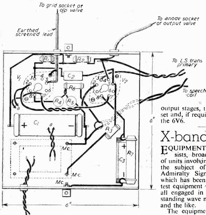
Fig. 3.—Practical wiring diagram.
