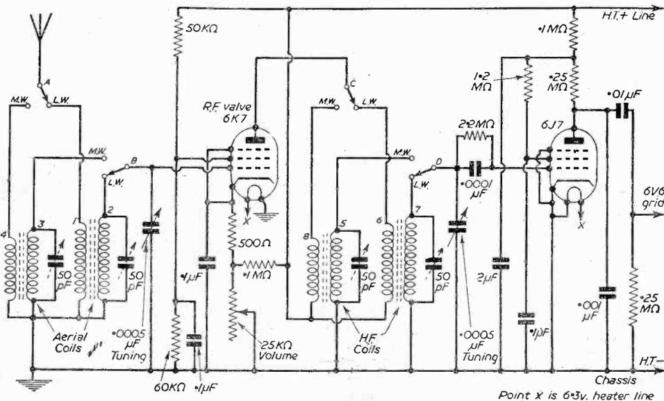
Theoretical circuit of the H.F. and Detector stages. Point x is 6.3v. heater line
