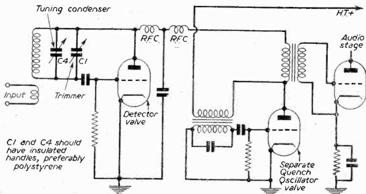
Fig. 3.—Basic externally quenched (capacitive) circuit.
