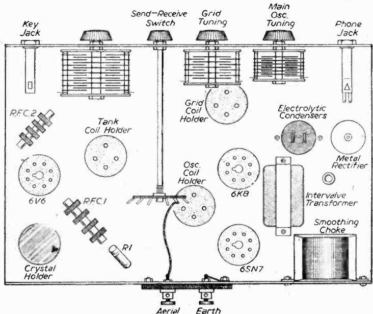
Fig. 4.—Below chassis layout.
