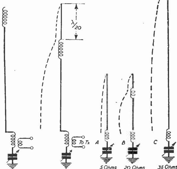
Fig. 1.—An extreme case of end-loading. Not recommended.
