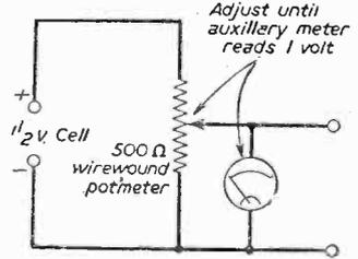
Fig. 3.—Temporary hook-up for calibrating the meter.
