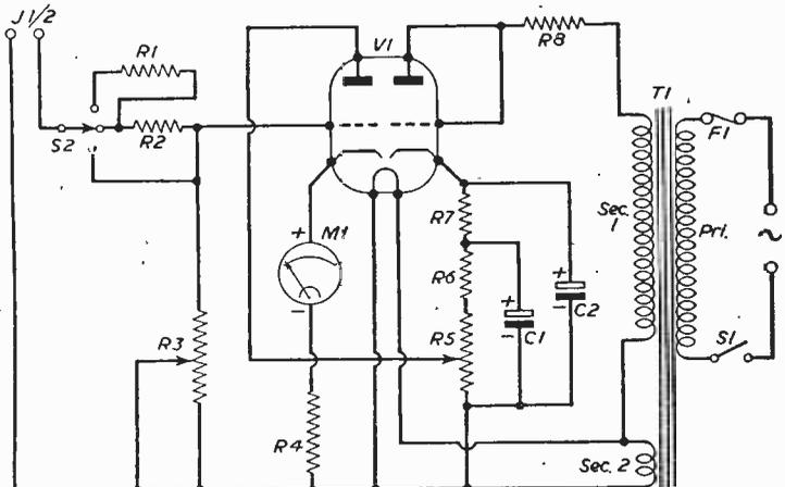
Fig. 1.—Theoretical circuit of the V.T.V.M.
