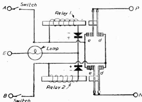
Fig. 2.—Modification for use with low-current relays.
