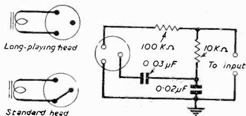
Fig. 5.—Automatic compensation system used in conjunction with Decca pick-ups.
