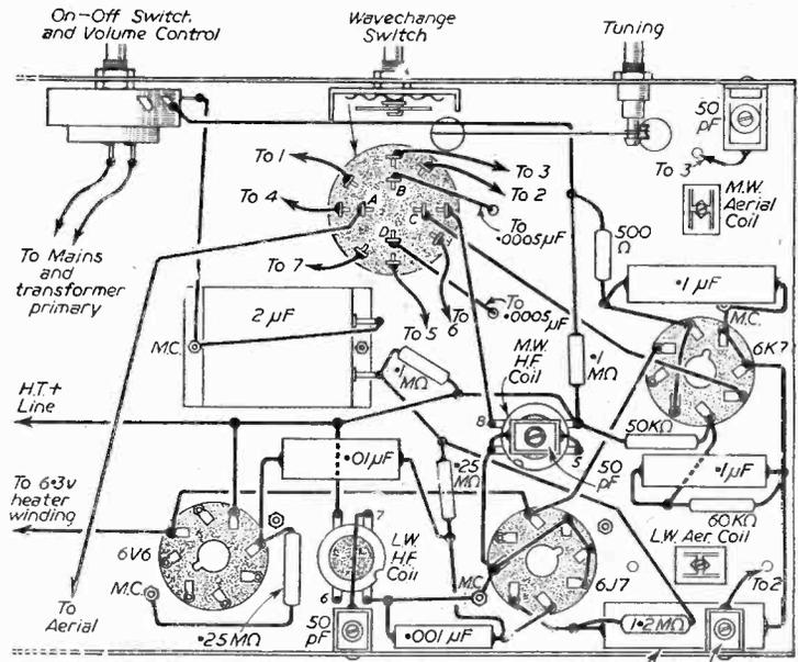
Note: Points marked MC, are connections to chassis
