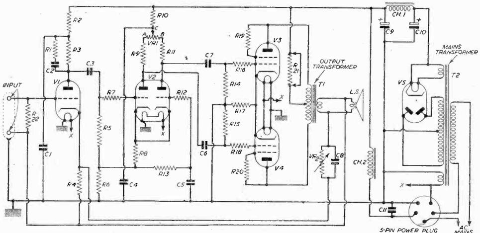
Fig. 1.—Theoretical circuit of the amplifier. A list of parts appears on page 124.
