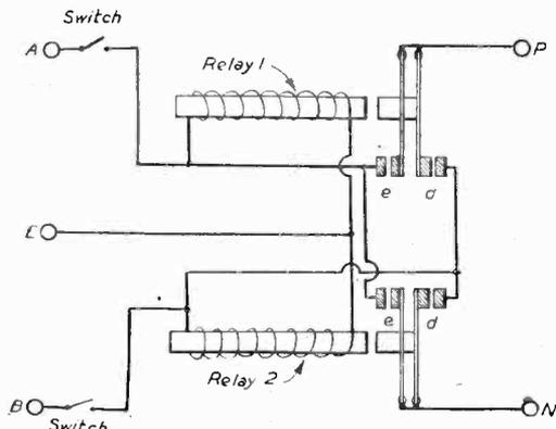
Fig. 1.—Standard circuit recommended by the author—e and d depict energised and de-energised positions respectively.
