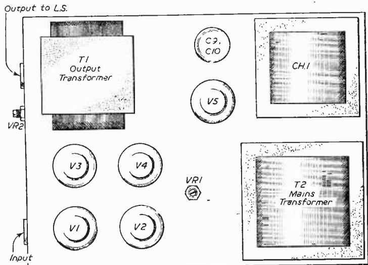
Fig. 2.—Suggested layout of the main components.
