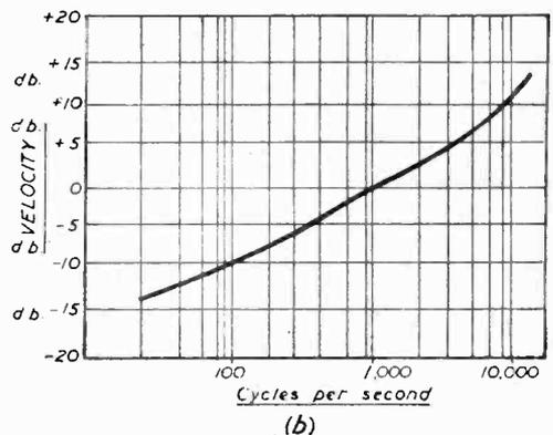
Fig. 1(a).—78 R.P.M. recording characteristic and (b).—Microgroove recording characteristic.
