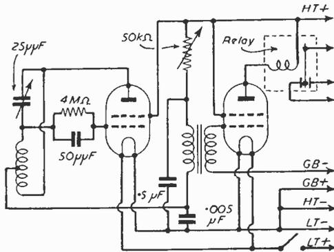
Fig. 1.—Circuit of a two-valve modulation controlled receiver.
