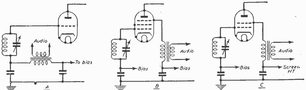
Fig. 1.—(A) Basic grid modulation circuit. (B) Basic suppressor modulation circuit. (C) Basic screen modulation circuit.
