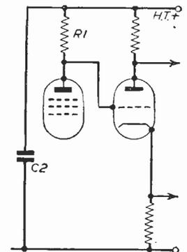
Fig. 4.—The coupling condenser has been eliminated here.
