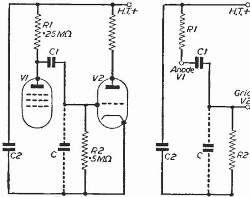
Fig. 1.—It can be seen that R2 forms part of a potentiometer R1 C1 which reduces the potential available at the grid of V2. Additionally at low frequencies the rising reactance of C1 and at high frequencies the stray capacitor C increases the loss.
