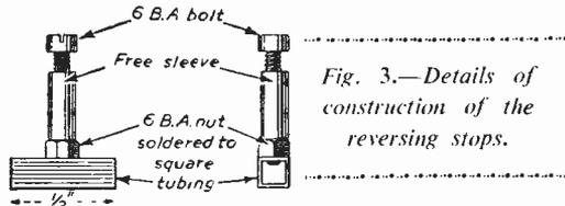
Fig. 3.—Details of construction of the reversing stops.
