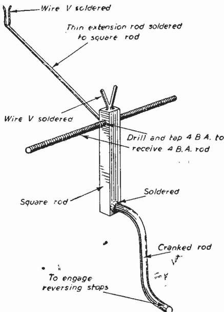
Fig. 4.—Constructional details of the wire guide.
