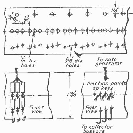
Fig. 6.—Details of construction of the main keyboard distribution board, seen at the rear of the keyboard in the illustration below. Dubilier type BTS resistors are wired as shown in the lower sketch.
