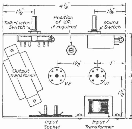
Fig. 6.—Amplifier dimensions and layout details.
