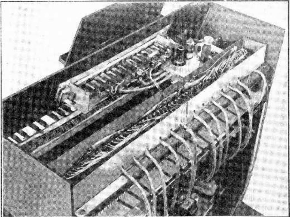
This illustration shows the keyboard with distribution board, main Fe. tabs and the small pre-amp, vibrato and tone-control valve chassis. Twelve screened five-way cables convey the outputs from the tone generators to the distribution board.
