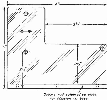
Fig. 2.—Shape and sizes of the sideplates. Two are required.
