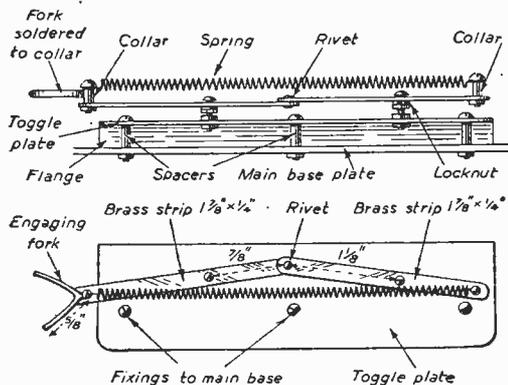
Fig. 5.—The first toggle seen in plan and elevation.
