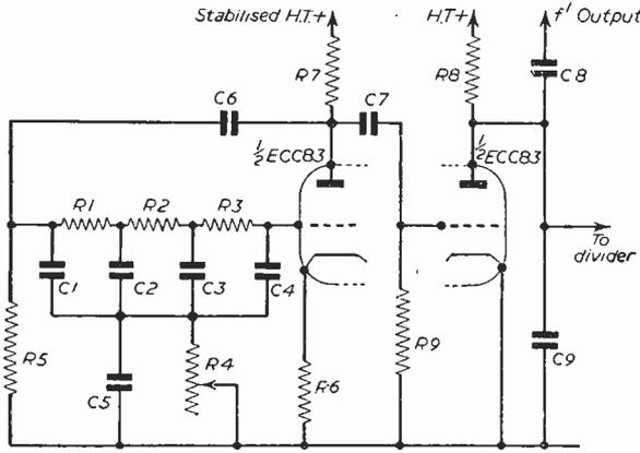
Fig. 3.—Theoretical circuit of the note generator and the buffer and saw-tooth converter. One of these is used for each of the 12 notes of the octave.
