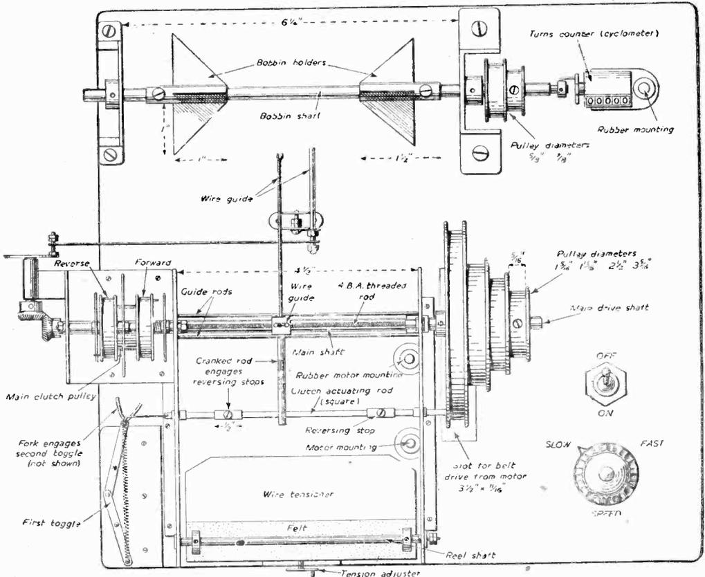
Fig. 1.—Plan of the complete machine with all parts identified.
