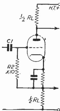
Fig. 2.—The "concertina" phase splitter circuit.
