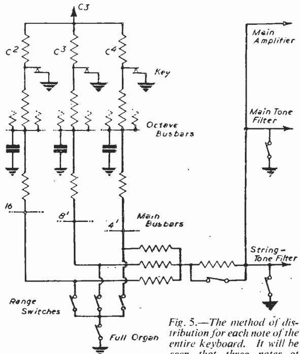
Fig. 5.—The method of distribution for each note of the entire keyboard. It will be seen that three notes in octave intervals are joined to each key which carries a three-contact switch.
