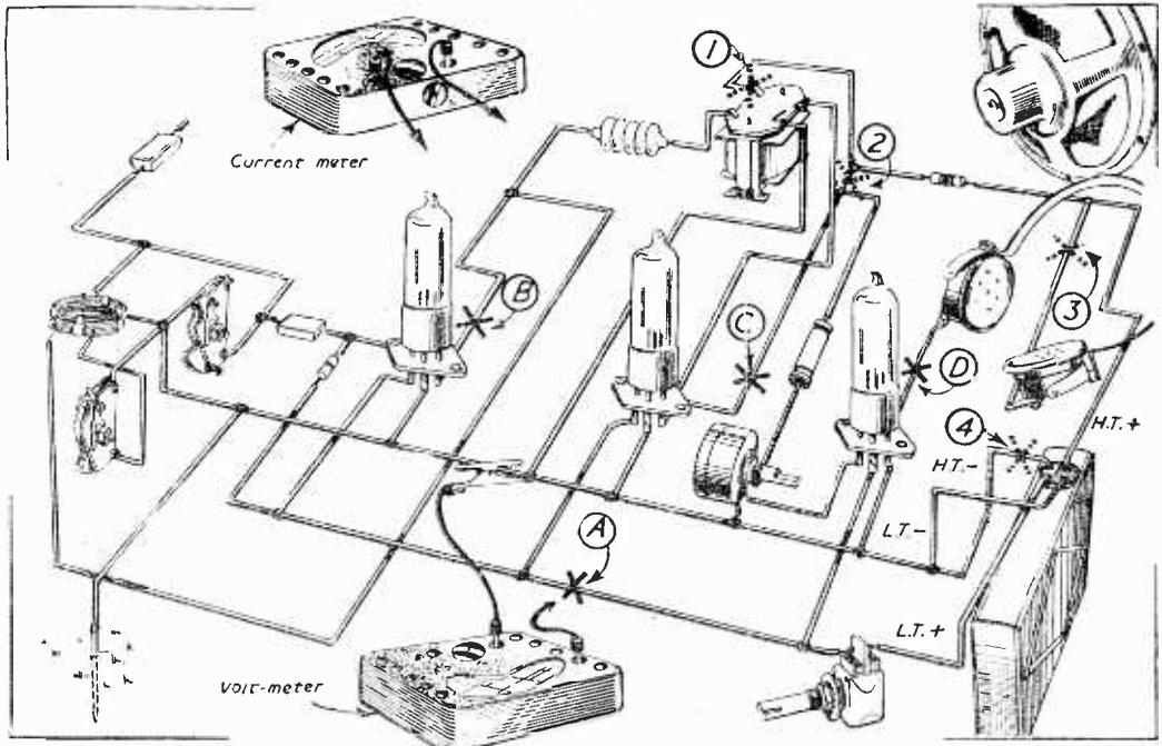
Fig. 31—The three-valve receiver circuit in pictorial form showing the points to which meters are joined for testing.
