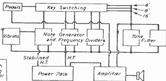
Fig. 1 (above).—Block diagram showing the essential arrangements of the design, and Fig. 2 (left) the manner in which the three double-diode triodes are employed for generating each note for five octaves. Twelve of these assemblies are used on four chassis.
