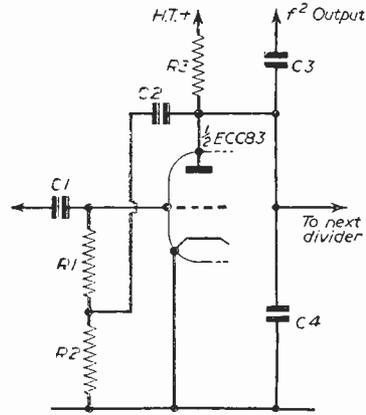
Fig. 4.—Theoretical circuit of the frequency divider. Four of these are used for each of the 12 notes of the octave, the only changes being in the values of condensers C1 and C4. Additional capacitors are used, as will be shown later, for coupling.
