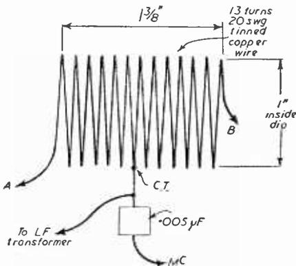
Fig. 4.—Details of the tuning coil.
