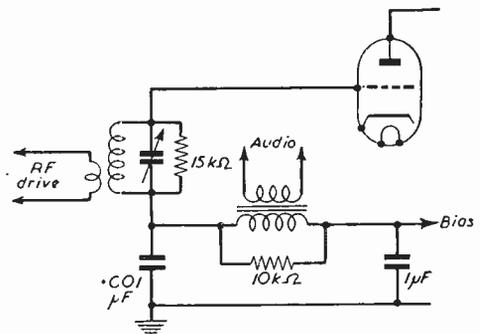
Fig. 2.—Typical values in a grid modulated system.
