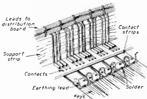
Fig. 8.—Details of the assembly of the key contact mechanism.
