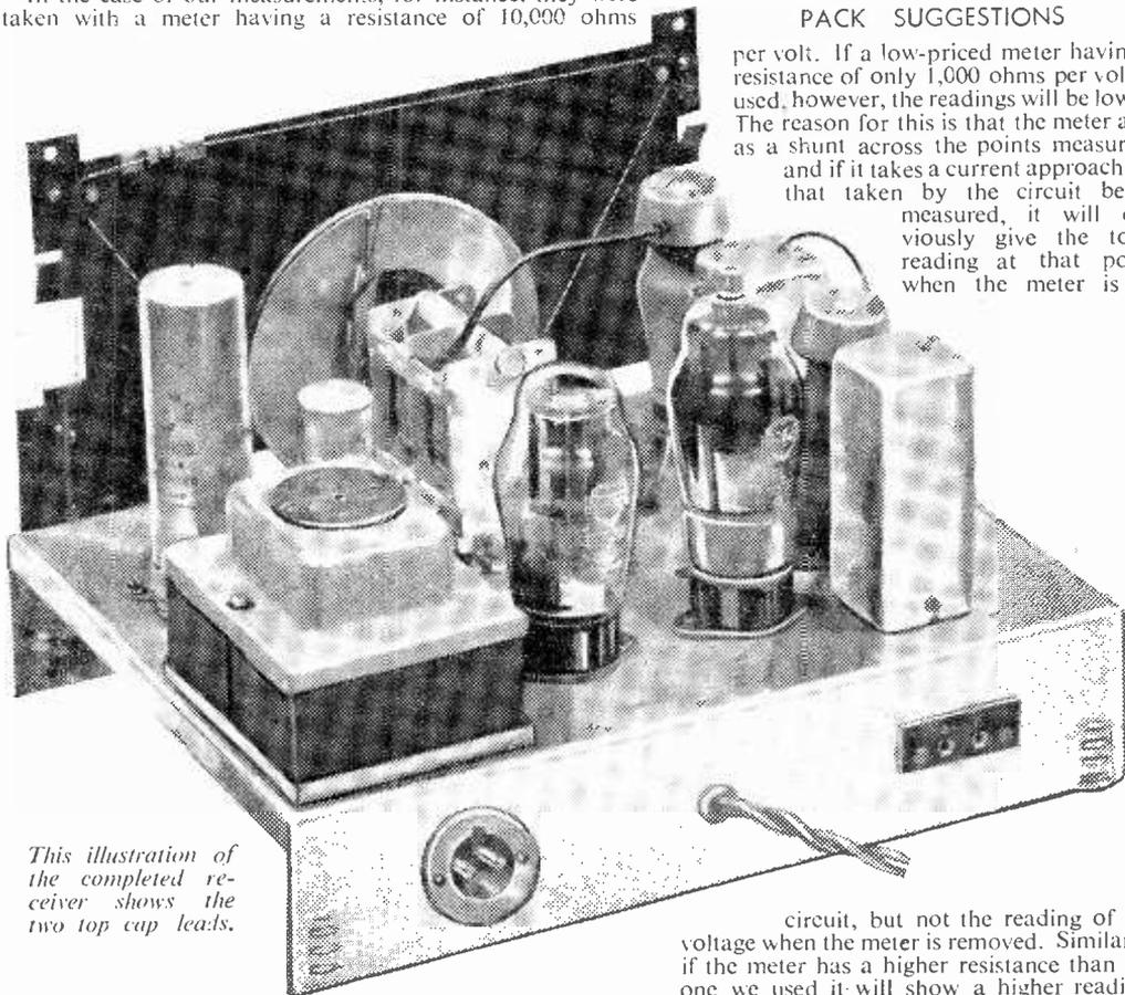
*This illustration of the completed receiver shows the two top cap leads.*
