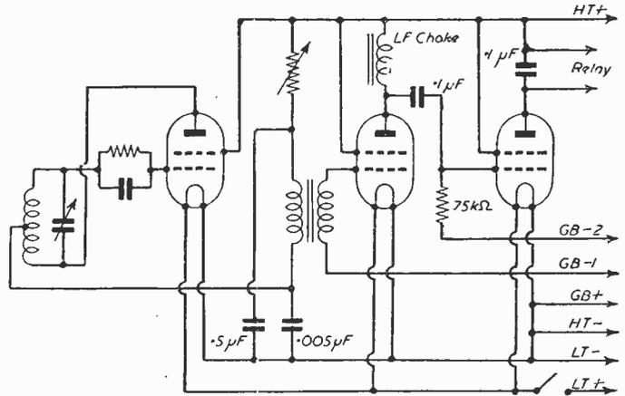
Fig. 2.—A three-valve circuit.
