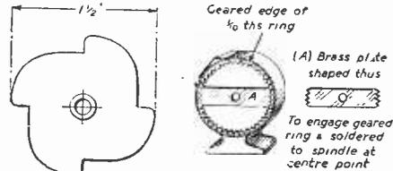
Fig. 10.—The modifications to the turns counter.
