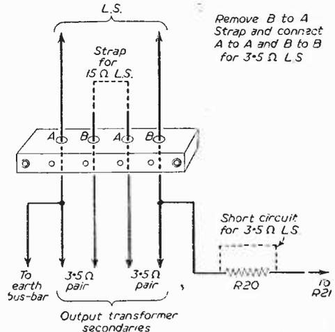
Fig. 9.—Loudspeaker output terminal block.
