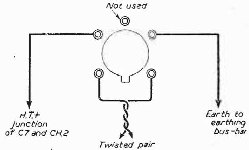
Fig. 6.—Wiring for the preamp. power socket connection.
