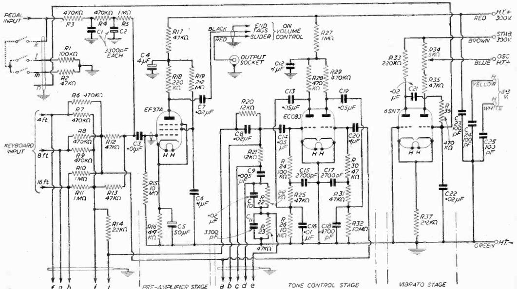
Fig. 13.—Circuit of the pre-amp unit, which includes the tone filter stage and the vibrato oscillator.
