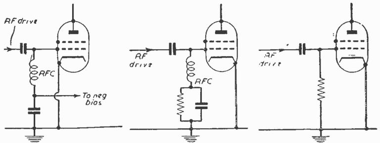
Fig. 1 (left).—Fixed bias circuit. Fig. 2 (centre).—By-passed grid-leak bias. Fig. 3 (right).—Un-by-passed grid-leak bias.
