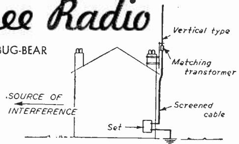
Fig. 1.—Aerial arrays for minimising interference.
