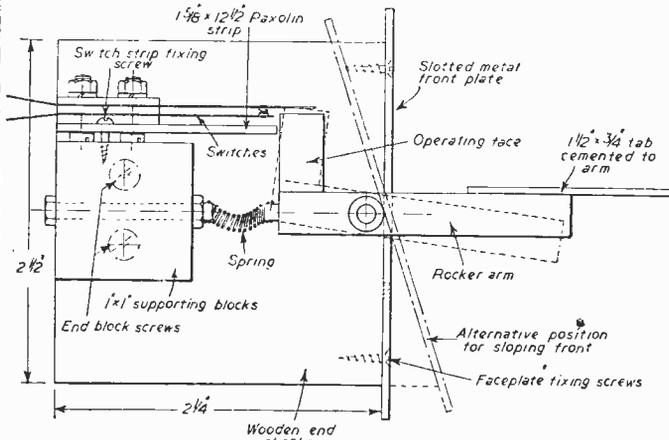
Fig. 9.—Details of the tab switches.
