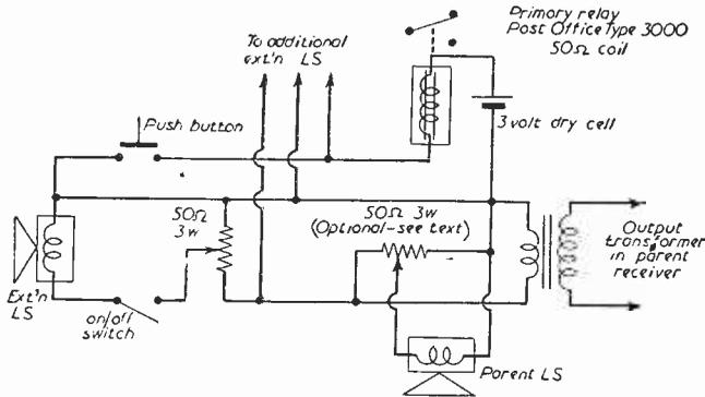
Fig. 1.—Primary operating circuit.
