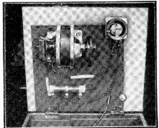
Fig. 9.—View of the underside of base plate showing felt surrounding the motor, and speed control.
