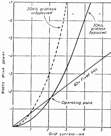
Fig. 4.—807 grid drive power requirements for the cases of 60 volts fixed bias, by-passed 30,000 ohm grid-leak, and for a 30,000 ohm grid-leak un-by-passed.
