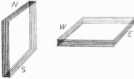
Fig. 2.—How a frame aerial may be used to locate the direction from which interference is coming.
