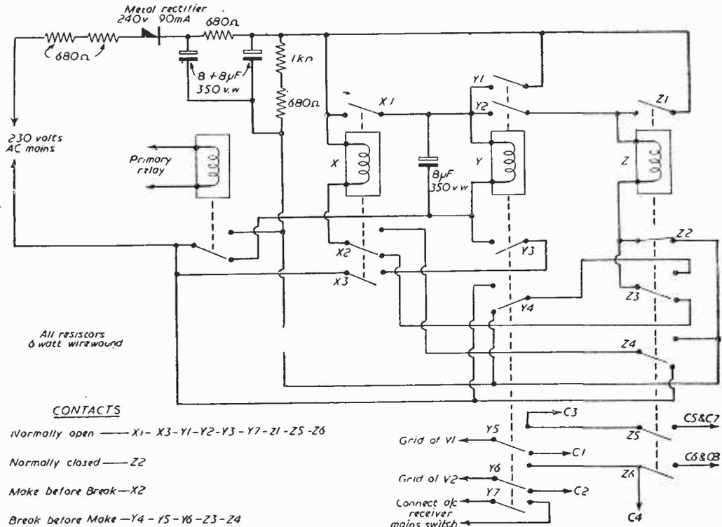
Fig. 3.—Cycling sequence circuit.
