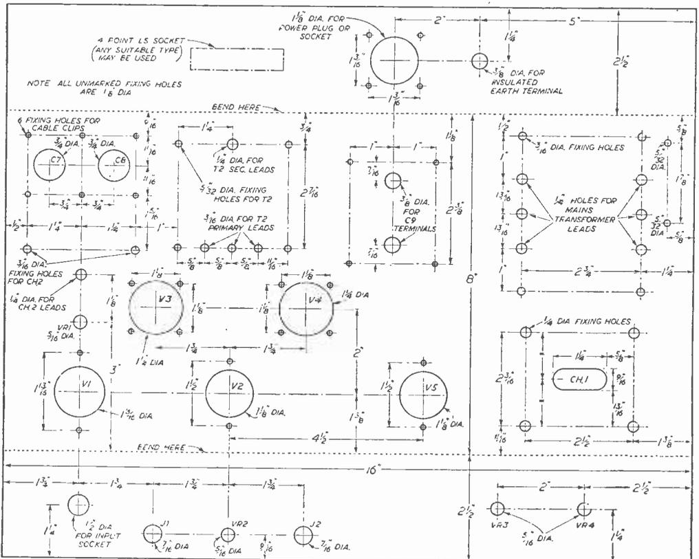
Fig. 10.—Chassis drilling data.
