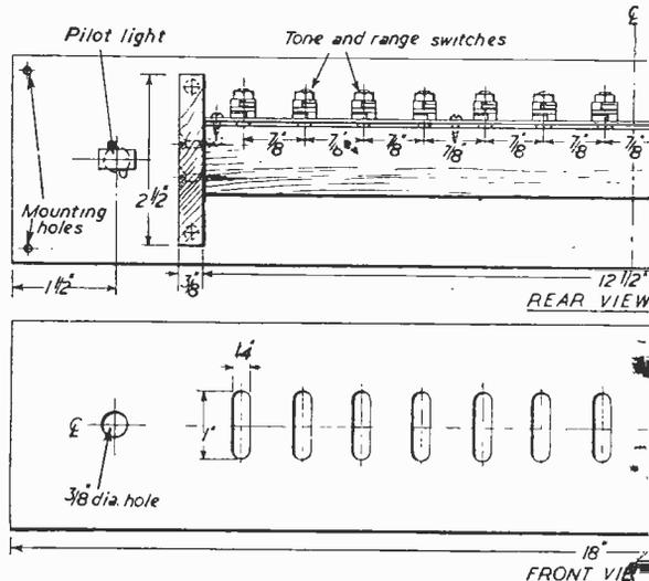
Fig. 10.—Details of the assembly
