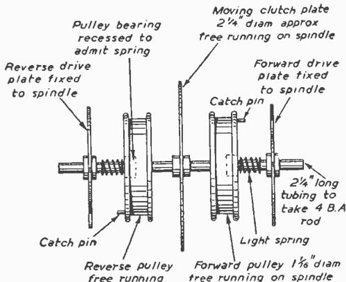
Fig. 8.—Detailed layout of part of the clutch mechanism. The parts have been spaced for clarity.
