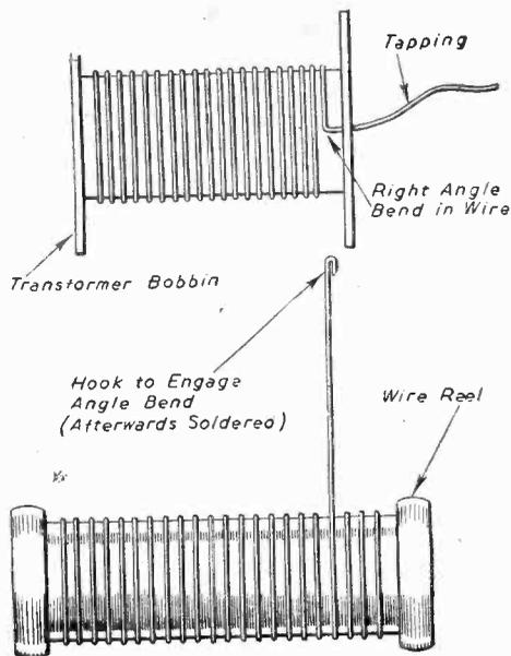
Fig. 13.—Method of making a tapping when using a heavy gauge of wire.
