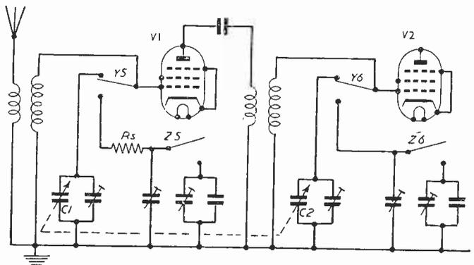
Fig. 5.—Showing how the relays Y and Z are used to alter tuning from manual (using C<sub>1</sub> and C<sub>2</sub>) to pre-set, for Light and Home programmes.
