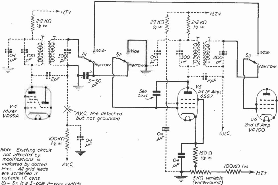
Fig. 1.—General details of the modification.
