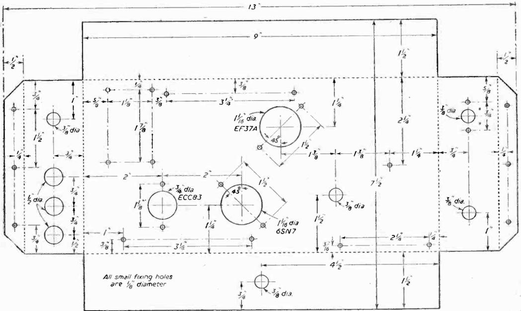
Fig. 12.—Chassis cutting and drilling details for the pre-amp.
