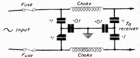
Fig. 3.—Typical mains interference suppressor circuit.
