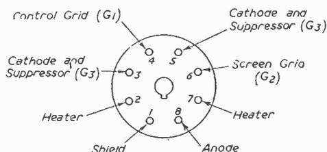
Fig. 2.—Details of the base connections of the 6SG7.
