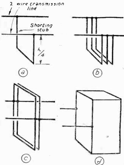
Fig. 3(a).—This stub has no effect on the line since the open end is of high impedance. (b) More stubs added to line. (c) More added edge to edge. (d) If the number of stubs is increased indefinitely and placed into contact, a metal tube,  $\lambda/2$  high results.
