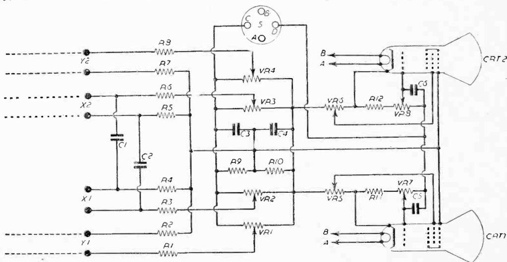
Fig. 3.—The cathode-ray tube unit.
