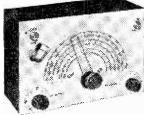
case 10 x 6 1/2 x 4 1/2 in., size of scale 6 1/2 x 3 1/2 in., 2 valves and rectifier, A.C. mains 230 250 V. Internal modulation 400 c.p.s. to a depth of 30%. Frequency calibration accuracy plus or minus 1%. Modulated or unmodulated R.F. output continuously variable 100 millivolts. Post and packing 4/-, £4/5/0.
