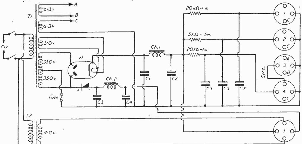
Fig. 2.—The power pack—C1 to C7 inclusive are 8μF 450 v.w. electrolytics.
