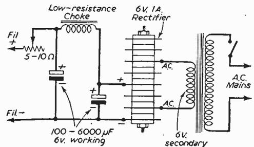
Fig. 3.—L.T. circuit for 1.4-2.0 volts.
