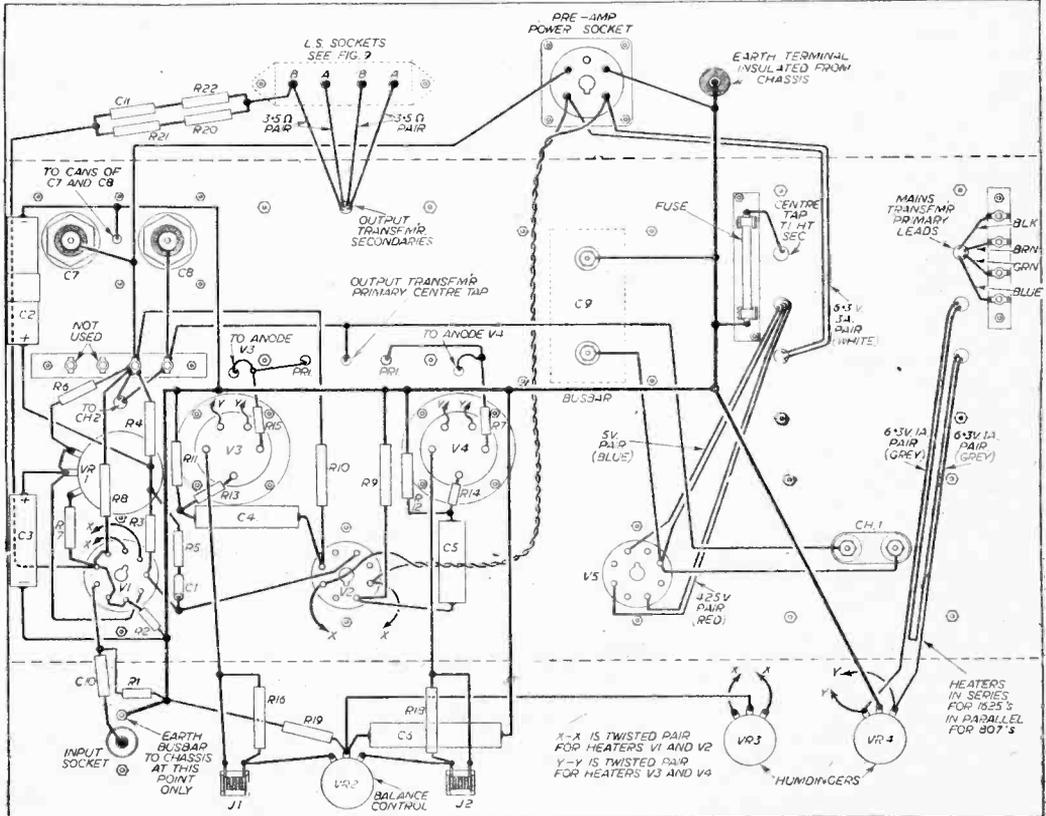
Fig. 12.—Wiring details for the amplifier.
