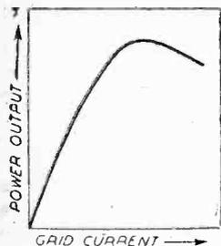
Fig. 2.—"Overdriving" a tetrode P.A. stage.
