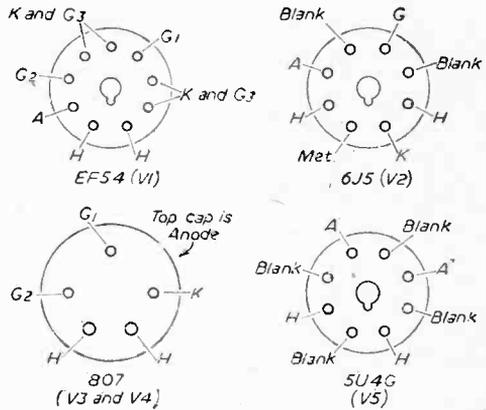
Fig. 11.—Valve base data for the valves used in the amplifier.
