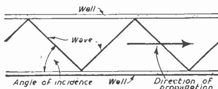
Fig. 2.—Showing how a wave is reflected from the walls of the wave-guide.
