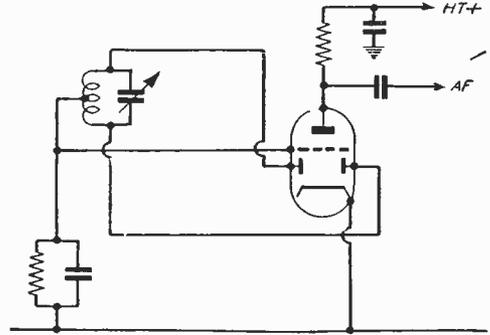
Fig. 2.—A full-wave detector circuit—this is actually a modified form of Fig. 1.
