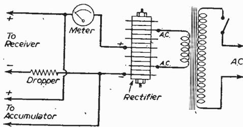
Fig. 6.—Trickle charger with dropper for 1.4v.
