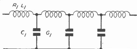
Fig. 1.—In this circuit the inductances have resistance  $R_1$ , and self inductance  $L_1$ , and the capacitors have capacity  $C_1$  and conductance  $G_1$ .
