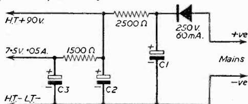
Fig. 4.—Simple "All-Dry" receiver power circuit.
