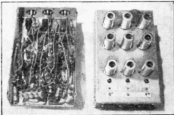
Two views of the note generator chassis. Four of these units are required.
