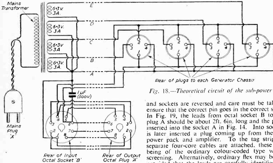
Fig. 18.—Theoretical circuit of the sub-power unit.
