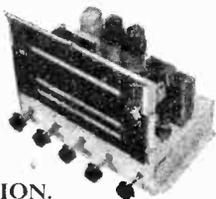
**FC.38** 8 valve Superheterodyne chassis, giving 8 watts push-pull output with negative feedback and separate BASS and TREBLE lift controls. WAVE RANGE: 16-50 metres, 190-550 metres and 1,000-2,000 metres. PRICE: £23 13s. including tax.
