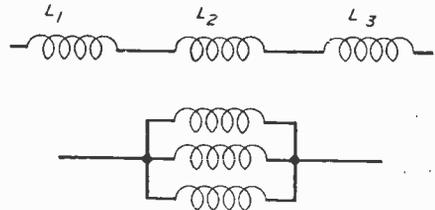
Fig. 36.—Top, inductances in series. Below, inductances in parallel.
