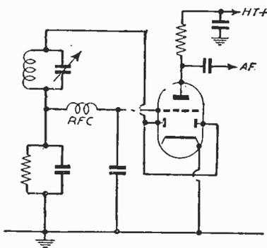
Fig. 1.—Typical half-wave detector—Diode anodes strapped together.
