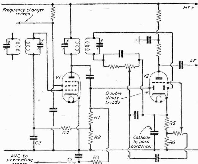
Fig. 3.—Typical circuit using a D.D.T. valve.
