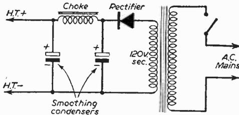
Fig. 1.—H.T. section of eliminator circuit.
