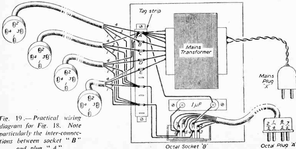
Fig. 19.—Practical wiring diagram for Fig. 18. Note particularly the inter-connections between socket "B" and plug "A."
