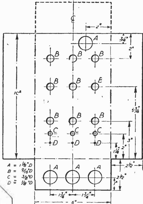
Fig. 17.—Chassis cutting and drilling data for the units shown on page 31.
