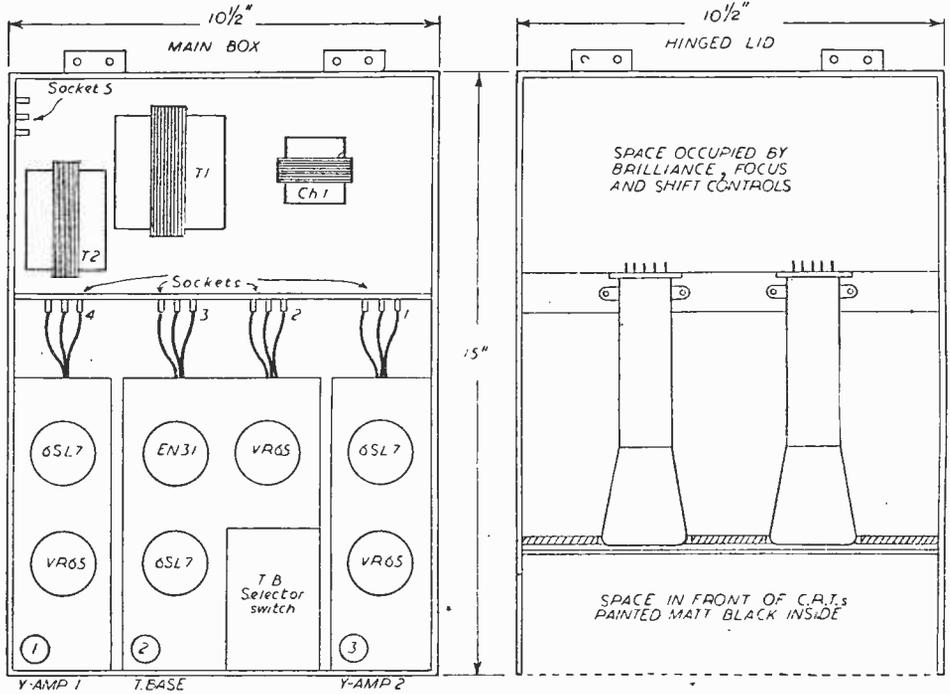
Fig. 1.—General layout of main components.
