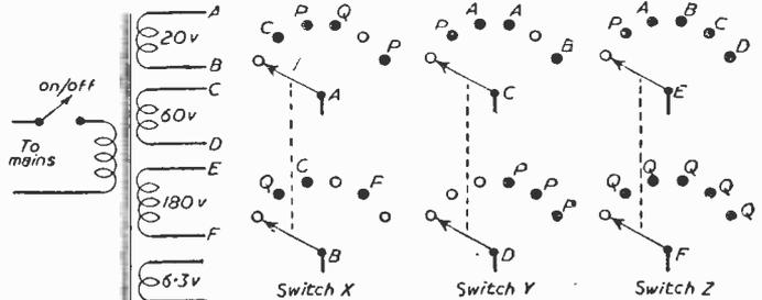
Fig. 1.—Connections between mains transformer and the three two-pole, six-way switches. Points marked P, Q are joined to the same points on Fig. 2.
