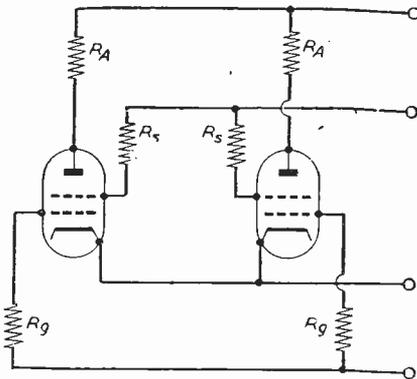
Fig. 6.—Method of paralleling 6L6s or 807s for greater output.  $R_A$ —10 ohms.  $R_S$ —47 ohms.  $R_g$ —220 ohms.
