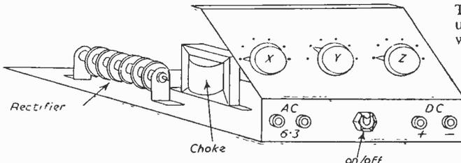
Fig. 3.—Showing layout and the control panel.
