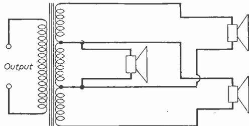
Fig. 2.—One form of rough matching using a single multi-section output transformer.
