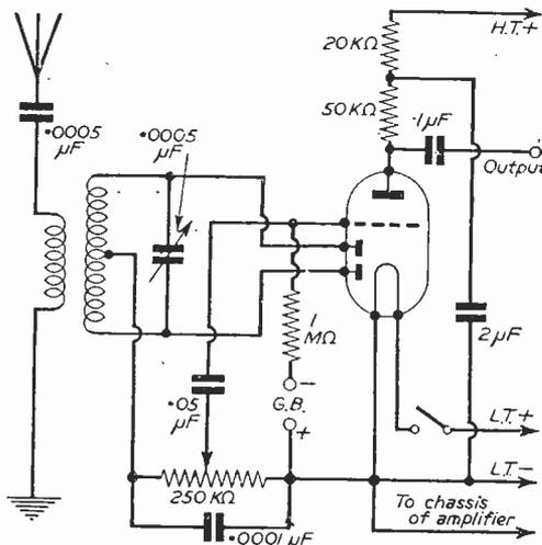
Fig. 2.—An attachment for either a mains or battery amplifier is provided by this circuit.
