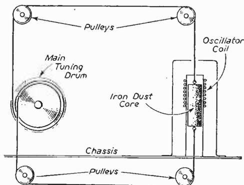
Fig. 8.—One method of mechanical tuning.
