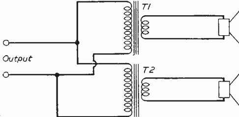
Fig. 3.—Using separate matching transformers.
