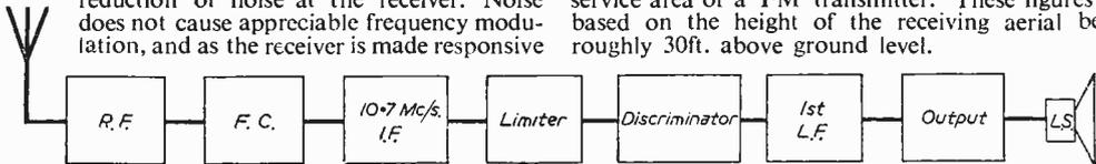
Fig. 3.—Block diagram of a FM receiver.
