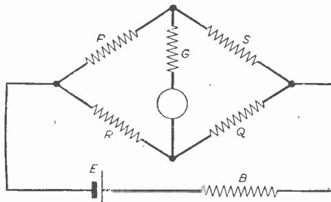
Fig. 1.—Basic bridge circuit.
