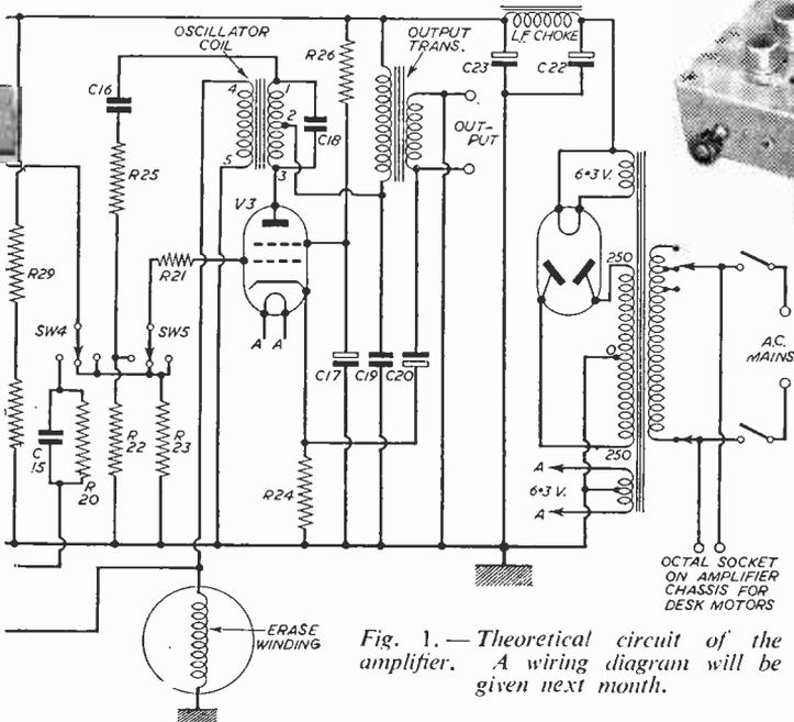
Fig. 1.—Theoretical circuit of the amplifier. A wiring diagram will be given next month.
