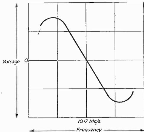
Fig. 7.—Graph showing discriminator output *V* frequency characteristic.
