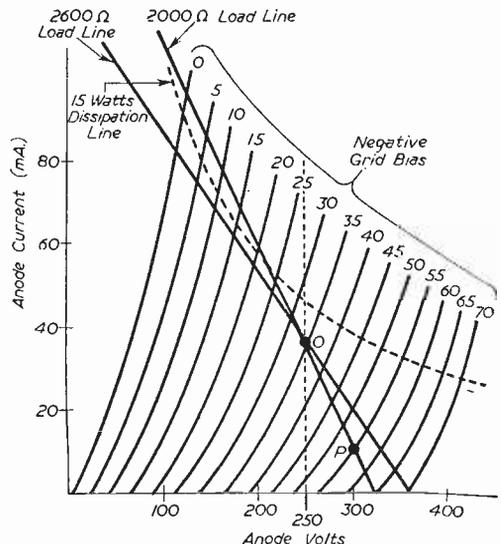
Fig. 31.—Triode output valve characteristic with load lines.
