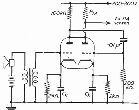
Fig. 4.—A "clamp-tube" version of the 6SN7 modulator for screen modulation of tetrode stages. No modulation transformer is needed.  $C_K$ —25  $\mu$ F, 2v.w. electrolytics.  $R_M$ —Value depends on P.A. valve and operating conditions.
