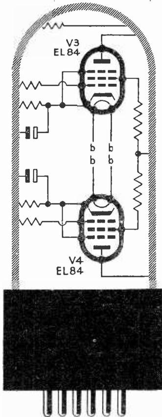
*These are the valves for the Mullard 5 valve 10 watt High Quality Amplifier.*
