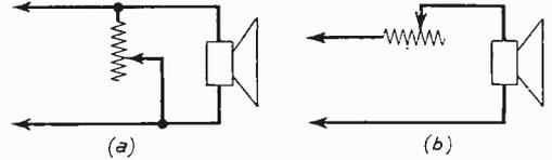
Fig. 4.—Methods of using a volume-control on an extension speaker.
