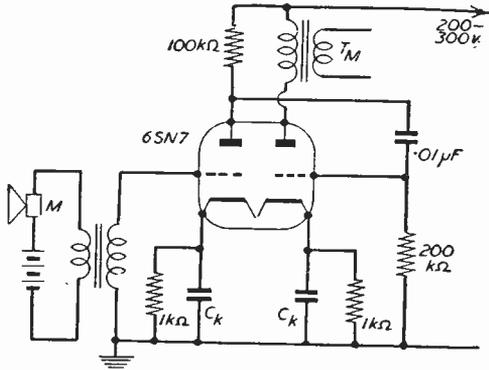
Fig. 3.—A modulator suitable for "efficiency" modulation. An easily obtainable double triode gives a two-stage modulator.  $C_K$ —25  $\mu$ F 25 v. electrolytics.  $T_M$ —"Intervalve" L.F. transformer.  $M$ —Carbon microphone.
