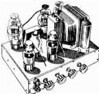
LOOPS with 15 db in the main loop from output transformer to voltage amplifier. Frequency response +3 db. 50-20,000 c.p.s. HUM and DISTORTION LESS THAN 5%
