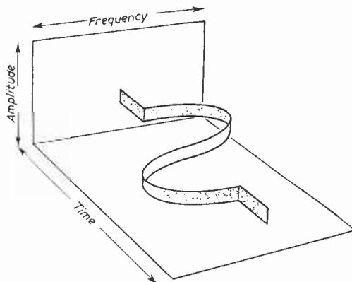
Fig. 2.—Diagram illustrating frequency modulation.
