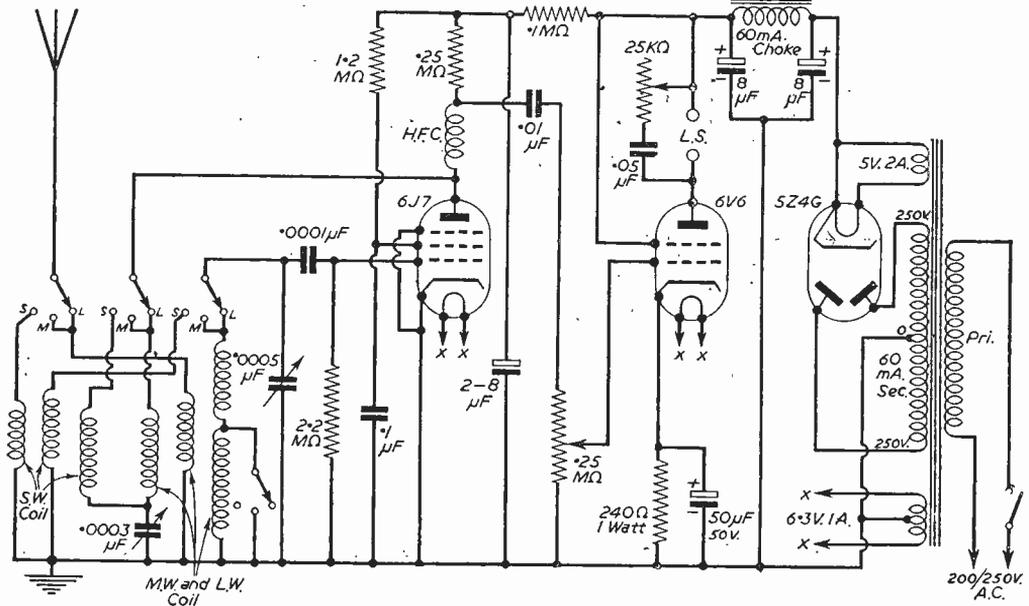
Fig. 5.—A complete All-wave A.C.2:
