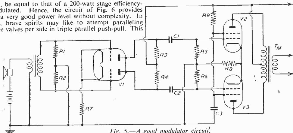
Fig. 5.—A good modulator circuit.
