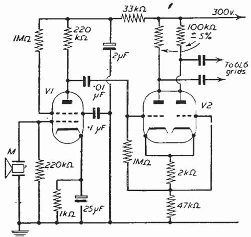
Fig. 7.—Method of modifying the circuit of Fig. 5 to allow a pre-amplifier to be used with a low-level microphone.  $V_1$ —6J7,  $V_2$ —6SN7.  $M$ —Crystal Microphone.
