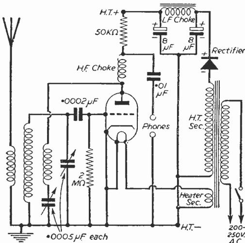
Fig. 1.—A 1-valver for A.C. mains.
