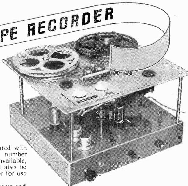
diagram, Fig. 1) is the fact that only three valves are used in the complete record and playback amplifiers (four valve stages) and these give more than adequate volume with a first rate standard of reproduction. The valves used are an EF37A for the high-gain low-noise input stage, a 6SN7 double triode for the two intermediate stages and a 6L6GT for the oscillator and output stage, the respective functions being switched in a similar manner to that originated in the "SoundMaster."
