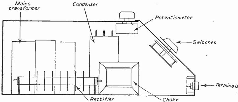
Fig. 5.—An elevation view of the H.T. unit.
