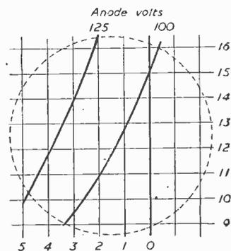
Figs. 84 and 85.—(Left) The grid-volts anode curve. (Right) An enlarged view of the circled section.
