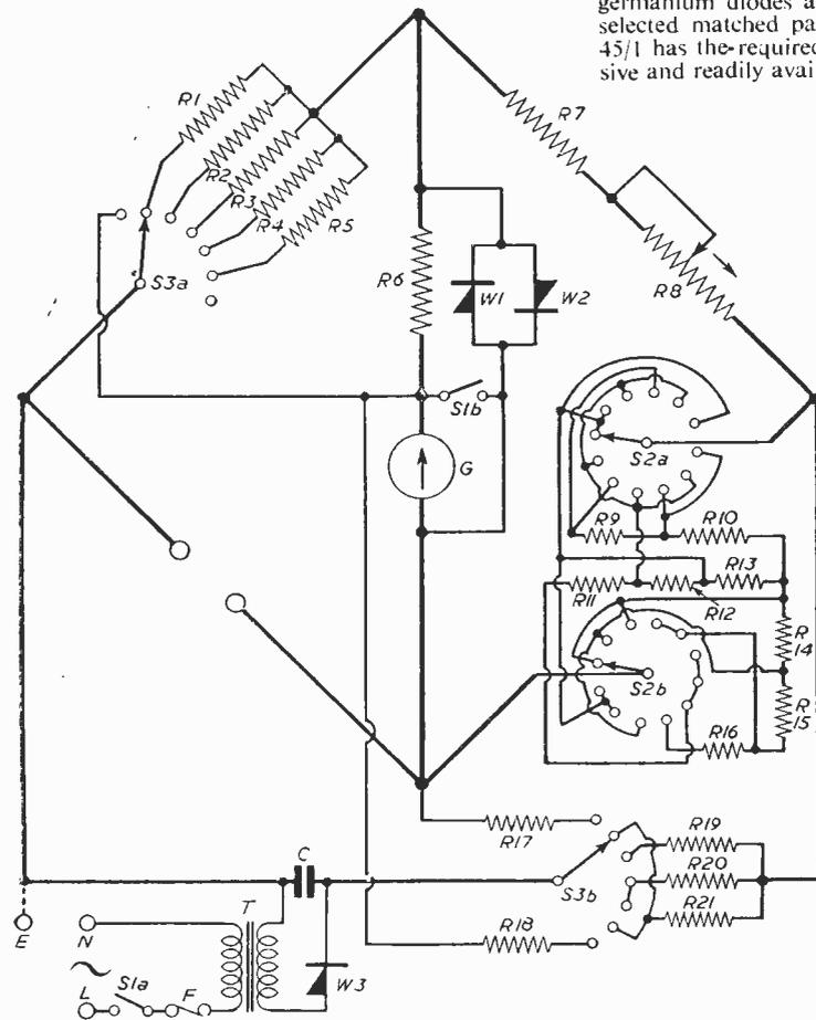
Fig. 2.—Circuit of the bridge described here.
