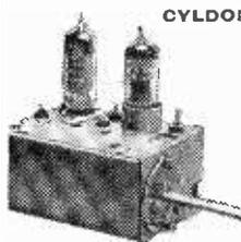
Instant and positive selection of any one of the 5 B.B.C. television channels, by a single control knob. Uses EF80 RF pentode and EC331 or 12AT7 Double Diode Triode as frequency changer. Tuning is obtained by switching incremental inductances. Size : 4 1/2 x 2 1/2 x 2 1/2 ins. Spindle 2 1/2 in. long, 1 in. diameter. I.F. Output 9.5-14 Mc/s., noise figure on all channels better than 10.5dB. I.F. rejection better than 45dB. **LASKY'S PRICE,** less valves, 12/6. Post Free.
