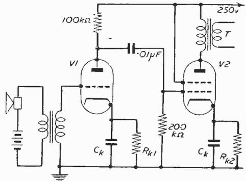
Fig. 2.—A simple two-stage modulator.
