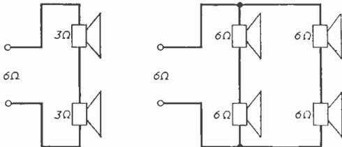
Fig. 1.—Matching the output when using more than one speaker.
