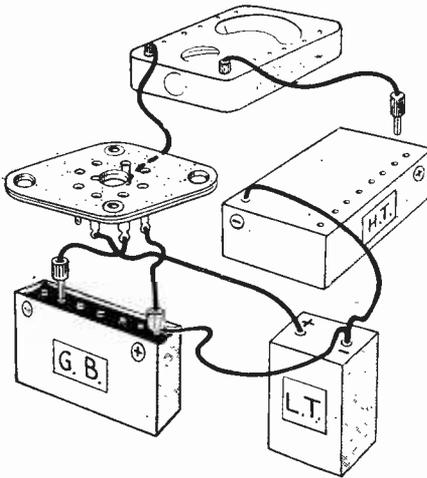
Fig. 86.—Set-up for taking valve measurements.
