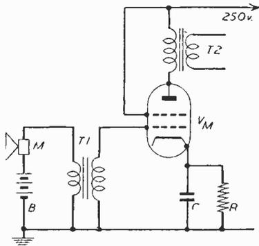
Fig. 1.—The simplest modulator.
