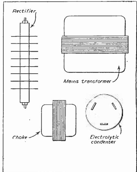
Fig. 4.—Showing layout of components on the base.
