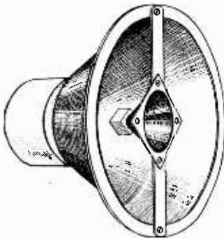
Fig. 5.—A suggestion for making up a concentric loudspeaker.
