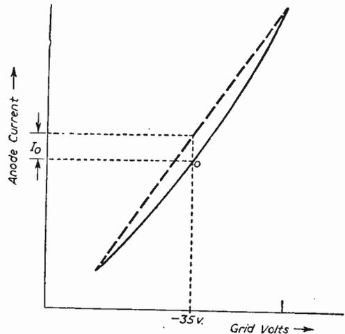
Fig. 32.—Distortion curve for triode showing second harmonic distortion. The divergence of  $I_0$  indicated by O indicates the degree of distortion.
