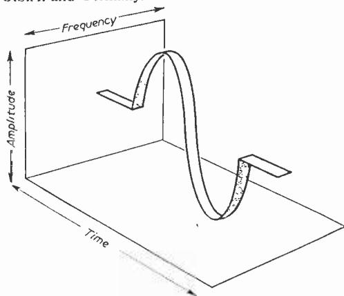
Fig. 1.—Diagram illustrating amplitude modulation.
