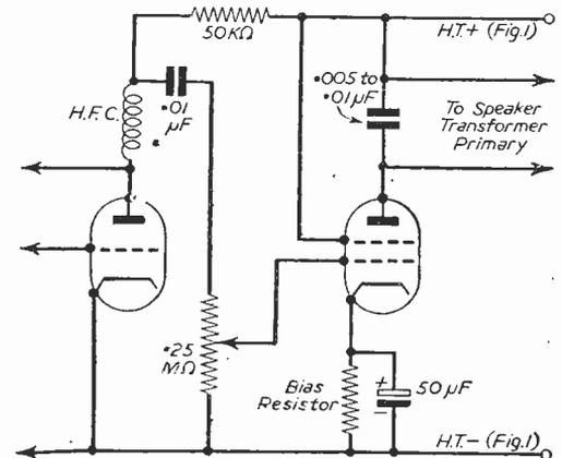
Fig. 2.—An output stage for speaker operation.
