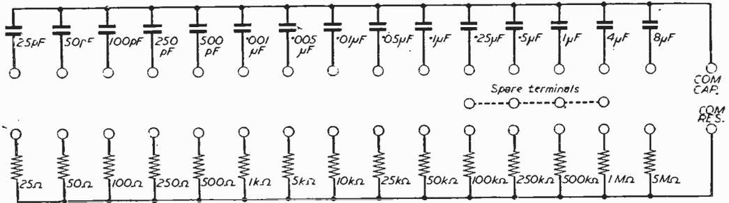
Fig. 6.—Capacitors and resistors are available in this box.
