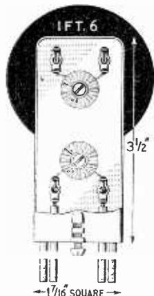
**IFT.6/465 kc/s or 1.6 Mc/s.**—A superior I.F. transformer for use in high quality receivers and tuners. Permeability tuned, Litz wound coils, using Neosid iron dust cores, and high quality silver mica condensers housed in an extruded aluminium can. Termination is made by four coloured leads. Coupling is optimum at 465 kc/s and slightly sub-optimum for increased selectivity at 1.6 Mc/s.
