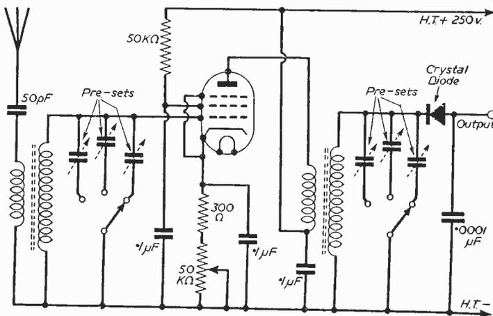
Fig. 3.—An R.F. detector Pre-set tuner.
