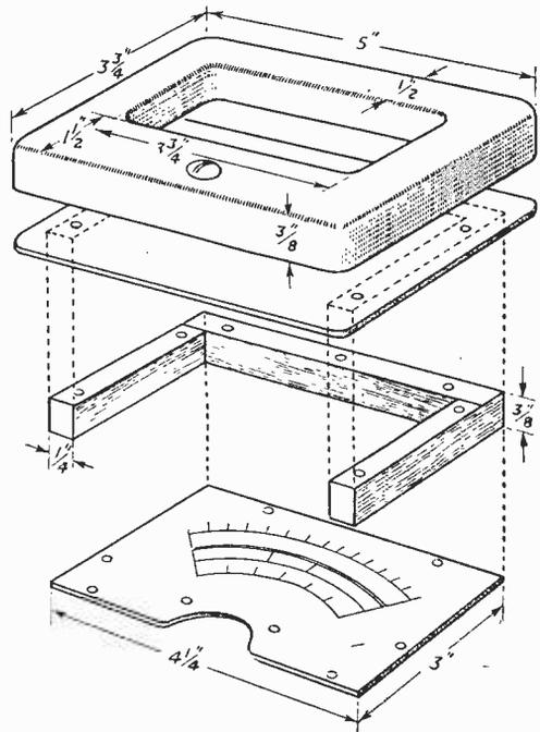
Fig. 5.—Details of the dial mounting.
