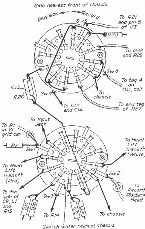
Fig. 3.—Details of the switch connections.
