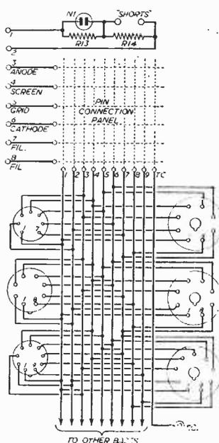
Fig. 2.—Wiring to the valholders.
