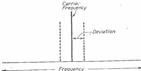
Fig. 9. — Diagram illustrating the deviation obtained in F.M.
