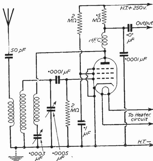
Fig. 2.—A simple one-valve tuner.
