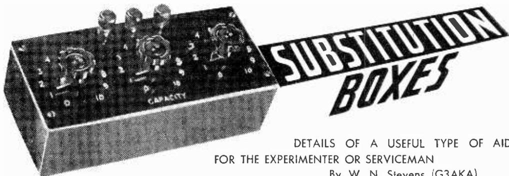
IT often happens that a certain component (or combination of components) in a receiver or other piece of equipment being constructed or serviced needs checking to ascertain if it is in good order. Also, and especially in experimental hook-ups, various components may be critical as to value, so that trial and error procedure is adopted until the best all-round practical values have been found. The components concerned are, of course, largely resistors and capacitors.
