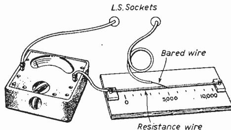
Fig. 91.—A simple output measuring device. The resistance may be made up by using bare resistance wire wound over a thin former.
