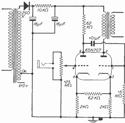
Fig. 1.—Basic theoretical circuit.
