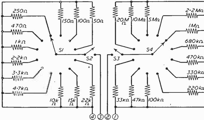
Fig. 3.—Low and high values are selected in this arrangement.
