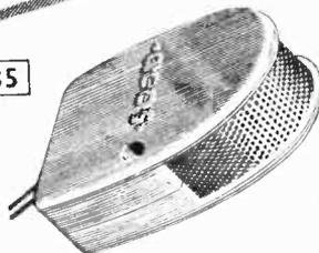
A general purpose hand microphone of robust construction with substantially flat response from 50 to 5,000 c/s. Suitable for recording apparatus. Public Address equipment etc. RETAIL PRICE £1-5-0d.
