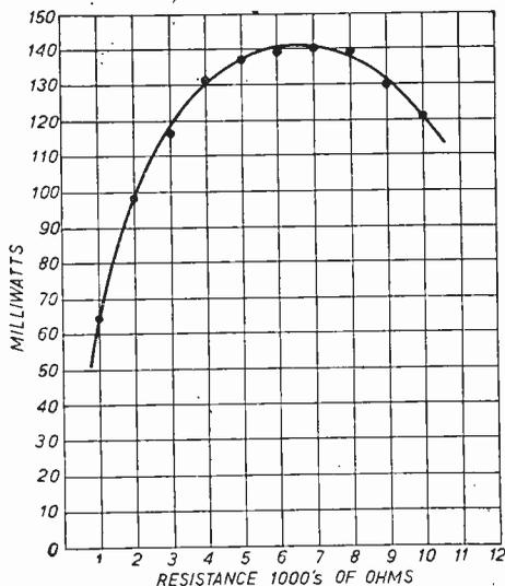
Fig. 92.—Plotting a graph for the output stage.
