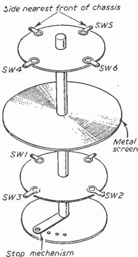
Fig. 6.—How the switch assembly is made up.
