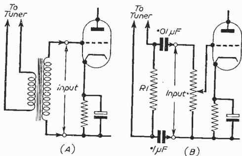
Fig. 4.—Two types of input circuit.
