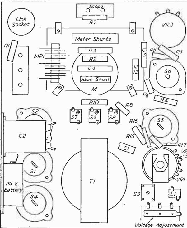
Fig. 6.—General view of the layout of main components.
