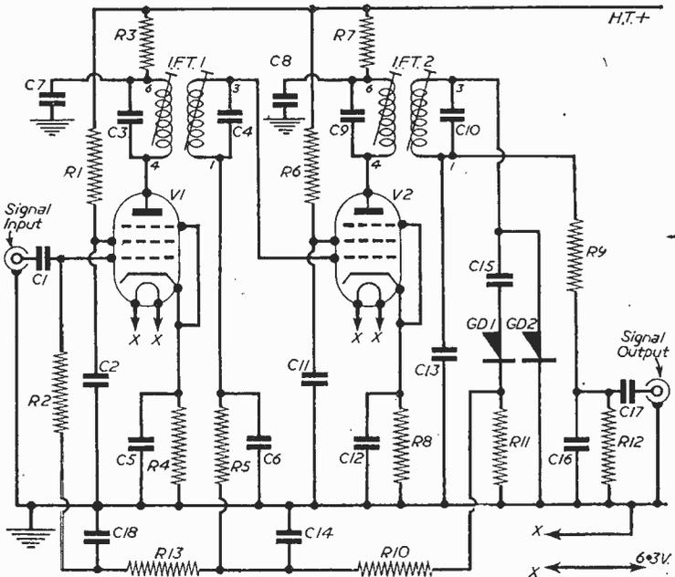
Fig. 14.—I.F. circuit diagram.
