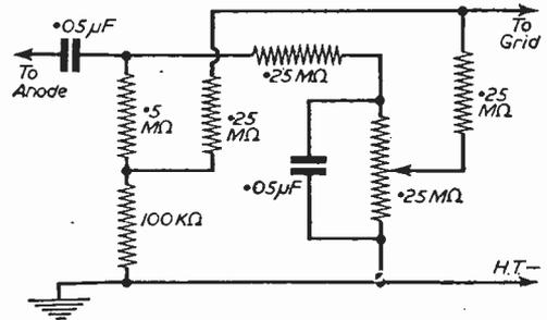
Fig. 4.—A continuously variable bass boost circuit.
