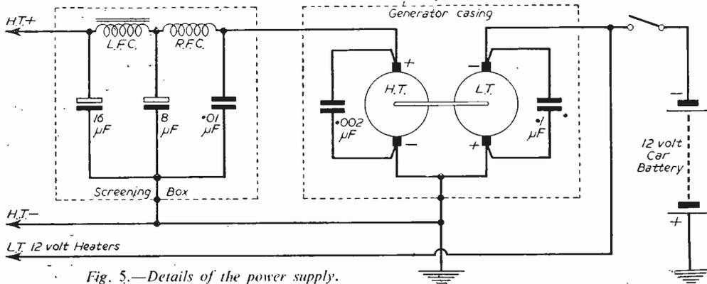
Fig. 5.—Details of the power supply.
