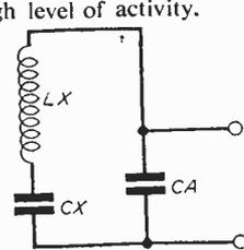
Fig. 1.—The equivalent circuit of a Quartz crystal.  $L_x$  may be several Henries, while  $C_x$  may be as little as .01 pF.  $C_A$  includes the effect of the holder plate capacity and is several pF.
