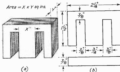
Fig. 6.—Core area and suitable laminations.
