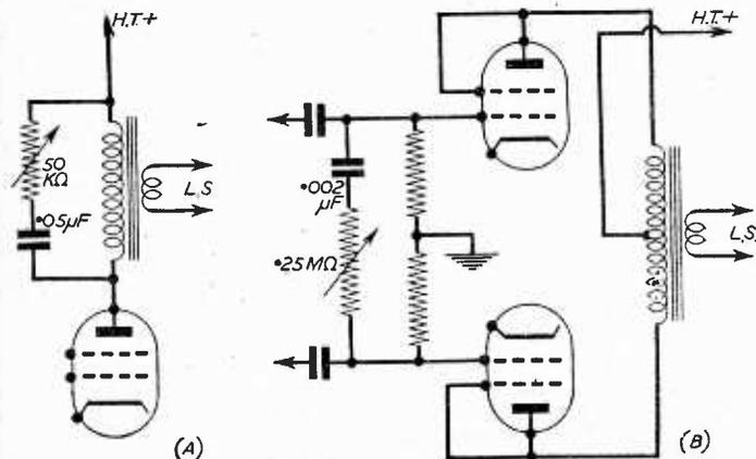
Fig. 1.—Two simple top-cut controls.
