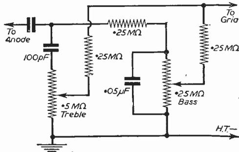
Fig. 5.—Separate controls for treble and bass.
