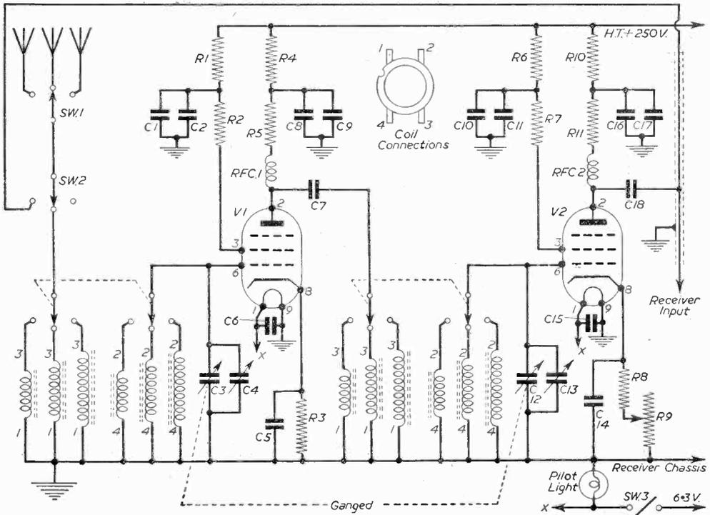
Fig. 1.—Theoretical circuit of the pre-selector.
