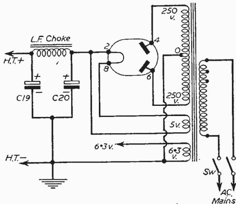
Fig. 2.—Details of a suitable power pack.
