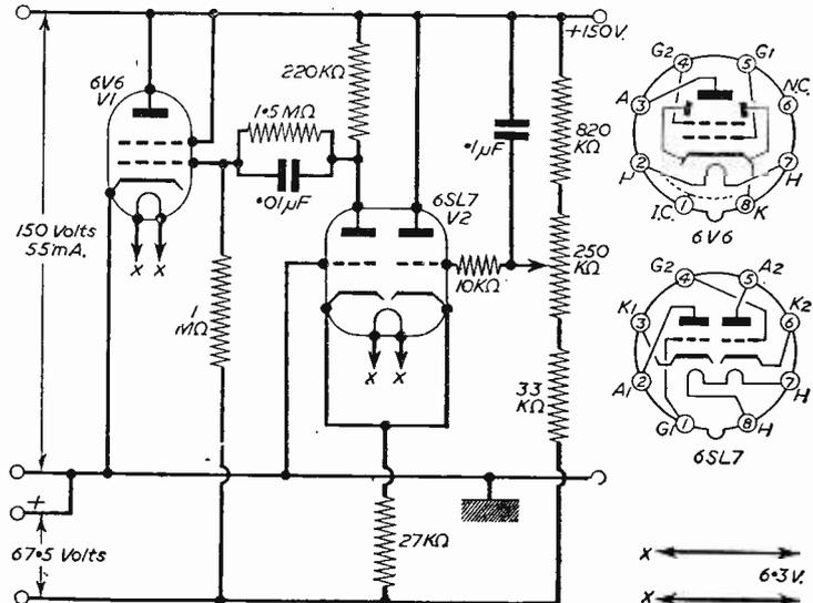
Fig. 5.—The circuit of a practical stabiliser.
