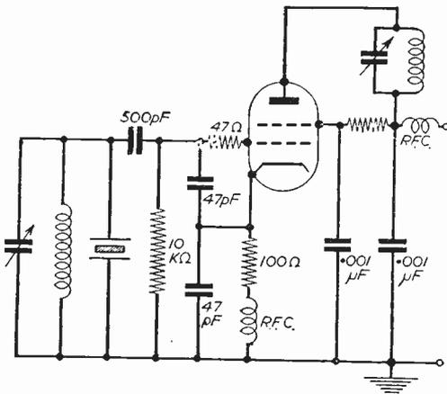
Fig. 6.—A cathode tap variation upon the basic circuit of Fig. 5.
