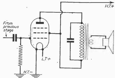
Fig. 4.—Basic output stage.
