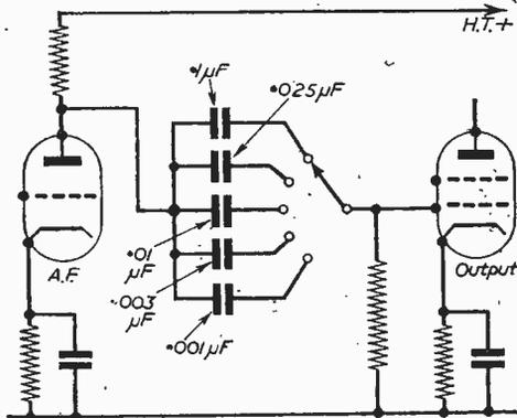
Fig. 2.—Bass cut by coupling capacity selection.
