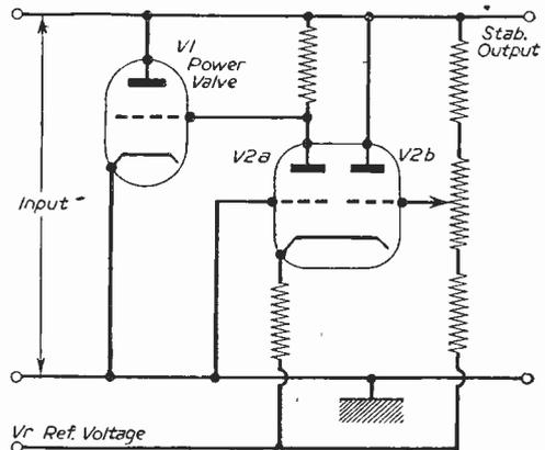
Fig. 3.—Simplified shunt regulator.
