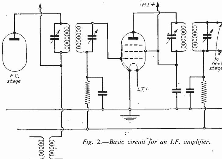
Fig. 2.—Basic circuit for an I.F. amplifier.
