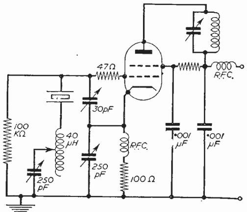
Fig. 7.—An elaborate and flexible circuit enabling circuit parameters to be separately adjusted for optimum performance. This is recommended as the circuit enabling a good degree of frequency shift to be obtained from miscellaneous crystals.
