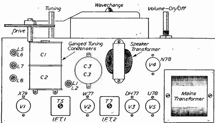
Figs. 2 and 3.—Above and below chassis layout with main components identified.
