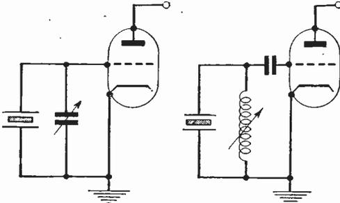
Figs. 3 and 4.—The oscillation frequency of a crystal may be shifted slightly by the above methods.
