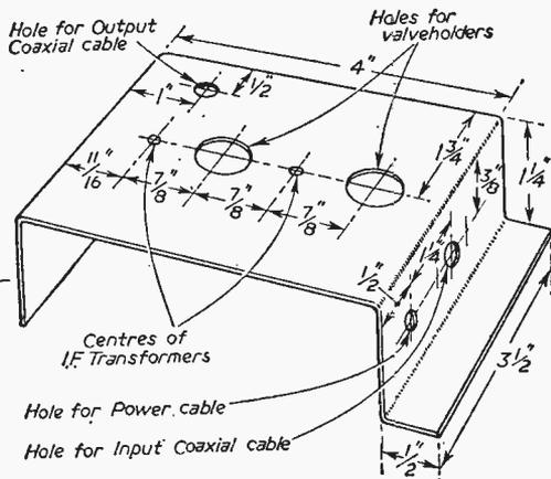
Fig. 15.—Details of chassis.
