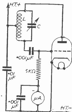
Fig. 74. — A grid-dip oscillator using a Hartley oscillator.
