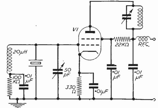
Fig. 5.—A more elaborate circuit for "rubberising" a crystal.
