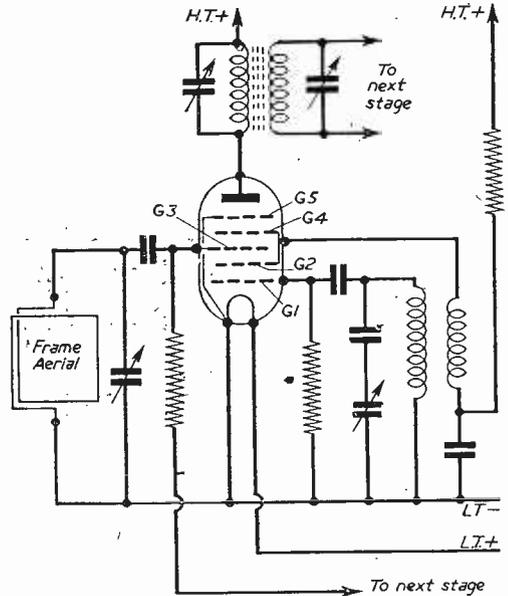
Fig. 1.—Basic circuit of frequency changer for battery miniature valves.
