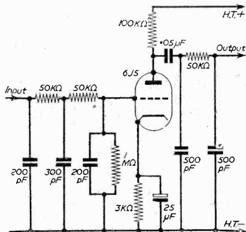
Fig. 7.—Steep cutting H.F. filter.
