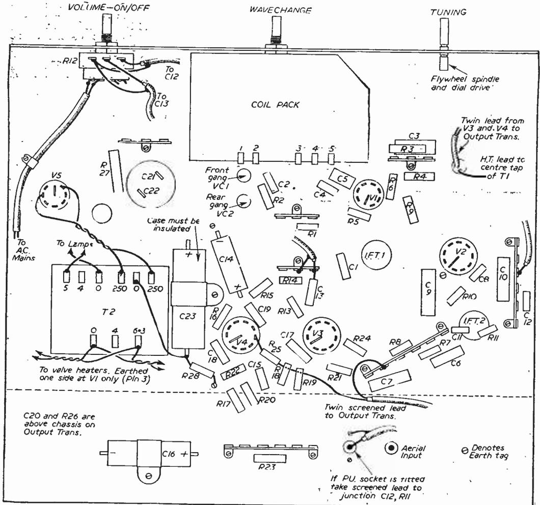
Fig. 4.—Wiring details and main component layout.
