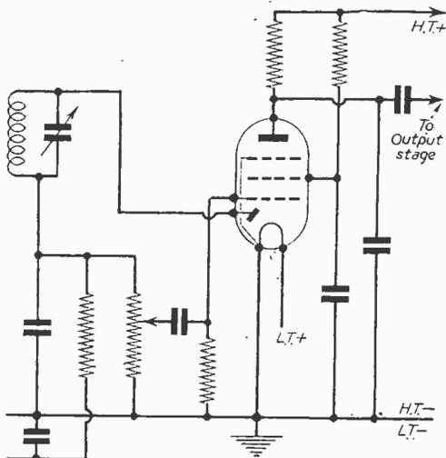
Fig. 3.—Basic circuit of diode detector and audio amplifier.
