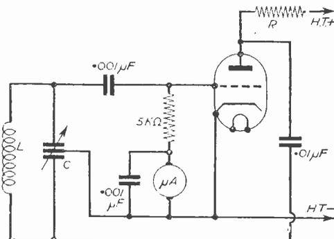
Fig. 75—A grid-dip oscillator using a Colpitts oscillator.
