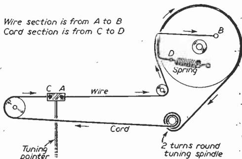
Fig. 4.—Details of the Cord Drive for the Tuning Dial.
