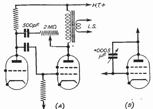
Fig. 6.—Using negative feedback to reduce top.
