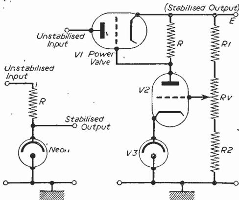
Fig. 1.—Neon stabiliser. Fig. 2.—Simplified series regulator.
