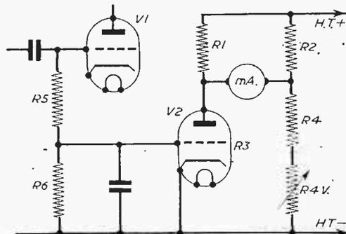
Fig. 77.—Amplifying a change in oscillator grid current by means of a valve bridge circuit.
