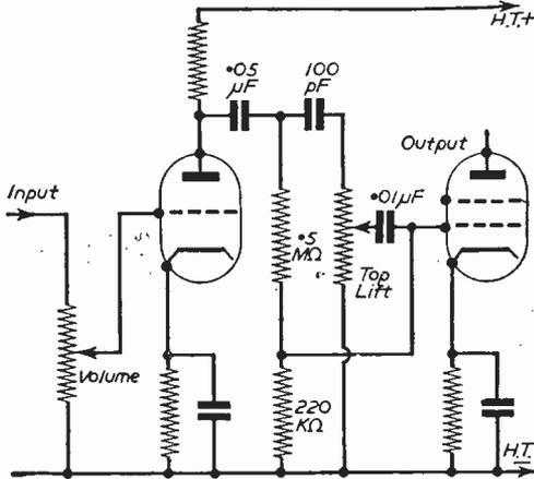
Fig. 3.—Circuit for top lift.
