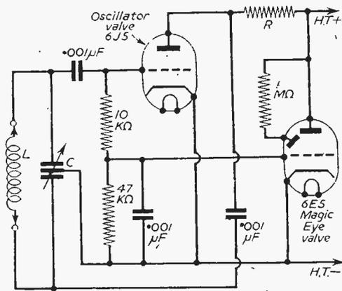
Fig. 76.—A method of using a "magic eye" valve to indicate a change in oscillator grid current.
