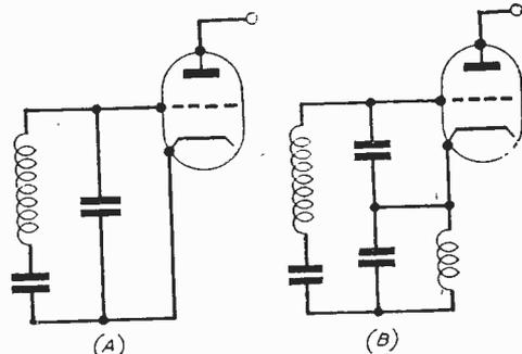
Fig. 2.—The similarity of the equivalent crystal circuit (a) to the Clapp-Harries oscillator circuit (b) is clearly shown.
