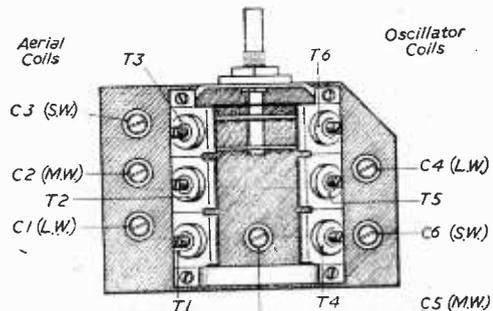
Fig. 5.—Details of the coils and trimmers.
