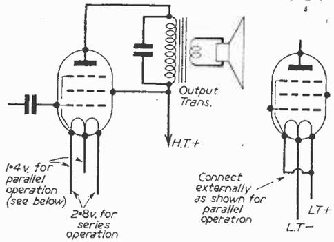
Fig. 5.—Basic circuit for output, using 2.8 volt filament valves.
