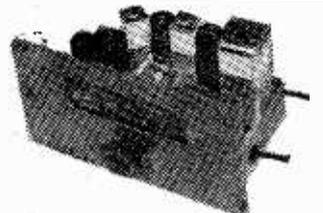
**P.M. TUNER-UNIT (87 mc/s—105 mc/s), by Jason.**
