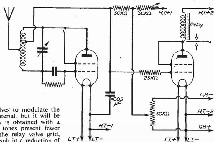
Fig. 4.—Direct-coupled amplifier.
