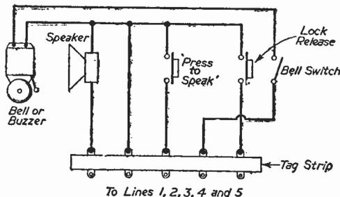
Fig. 4 (a)—Flat unit wiring.
