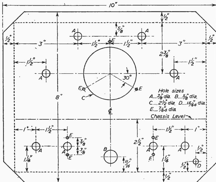
Fig. 2.—Panel drilling and bending data.
