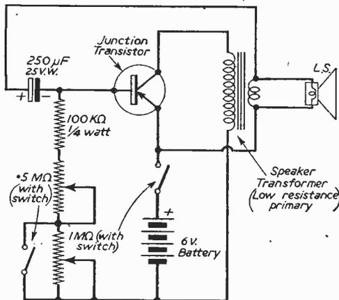
Fig. 1.—Theoretical circuit of the Metronome.
