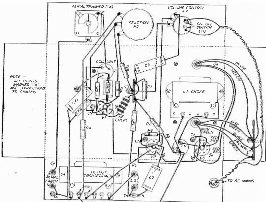
Fig. 6.—Below chassis wiring details.
