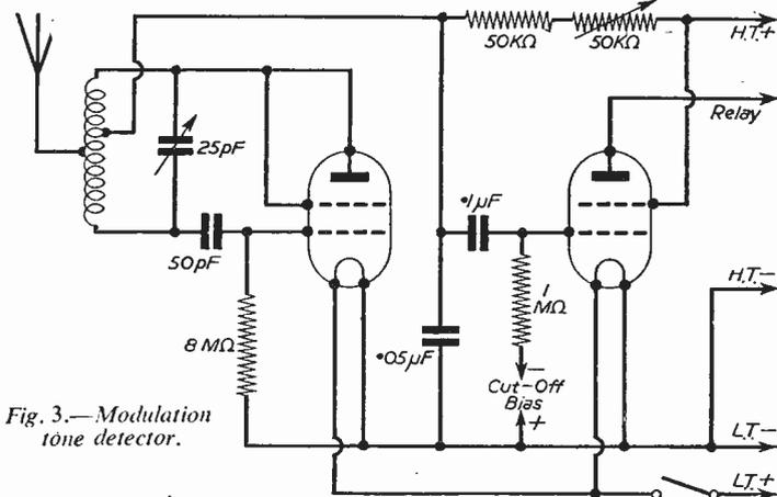
Fig. 3.—Modulation tone detector.
