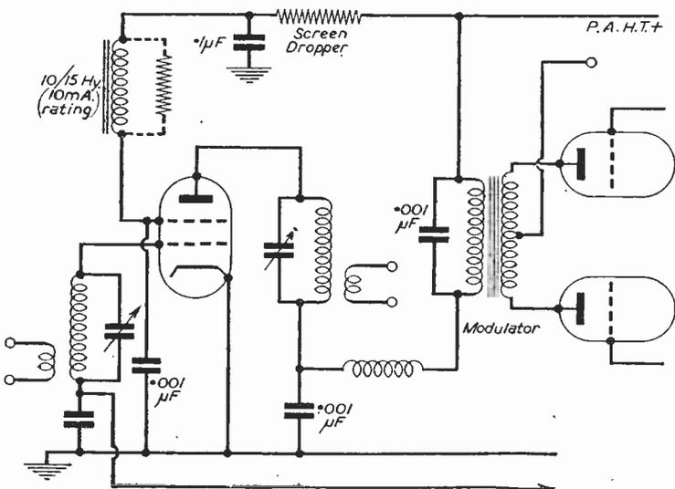
Fig. 4.—The self screen modulator circuit reproduced from last month's issue.
