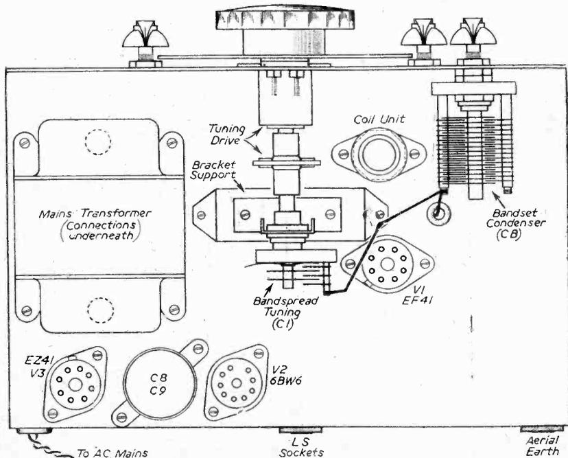
Fig. 5.—Above chassis wiring and layout details.
