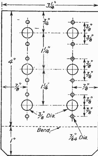
Fig. 7.—Drilling and bending details of the potentiometer bracket.
