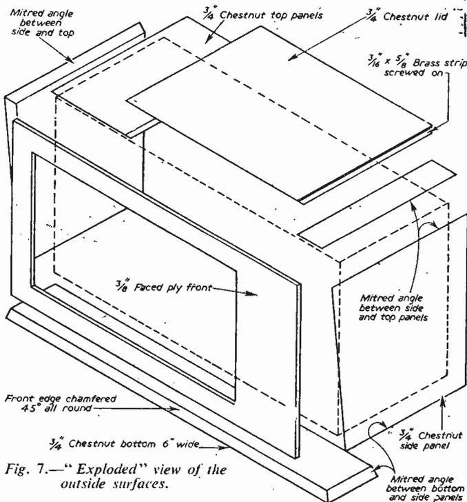
Fig. 7.—“Exploded” view of the outside surfaces.
