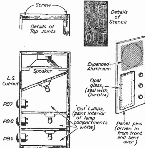
Fig. 3.—Constructional details of the front door unit.
