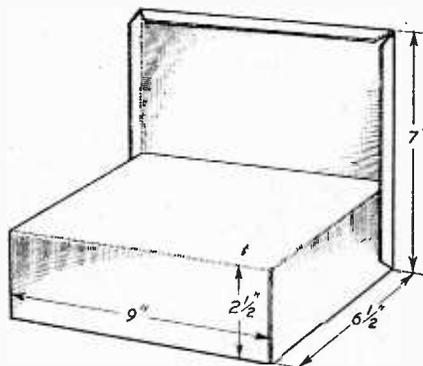
Fig. 4.—How the chassis is made up.
