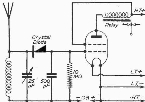
Fig. 2.—A diode-valve circuit.
