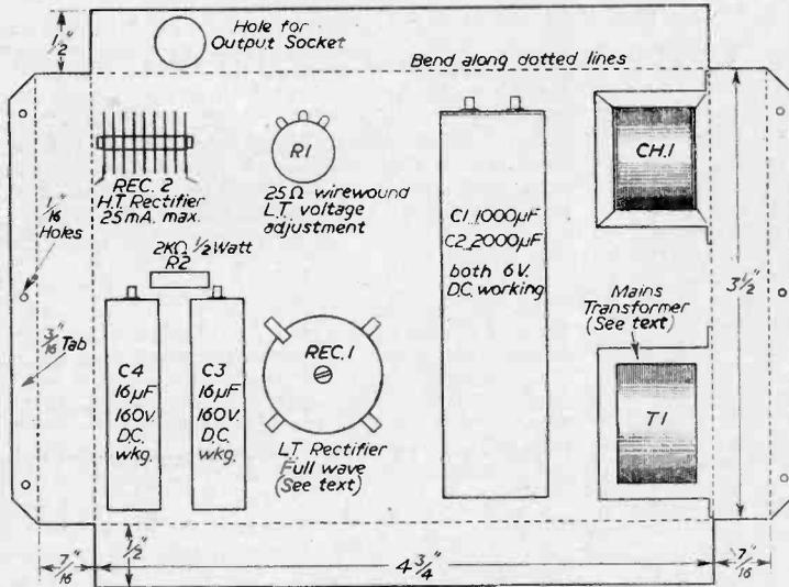
Fig. 2.—Layout and component values.
