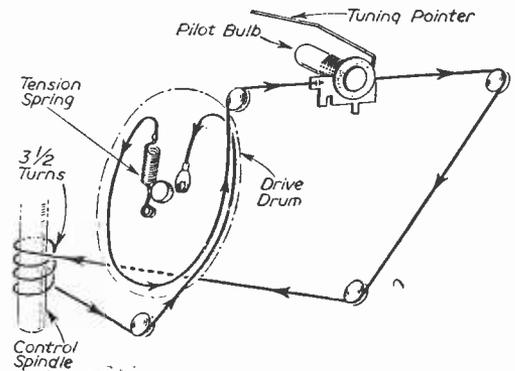
Fig. 4.—Details of the dial drive.
