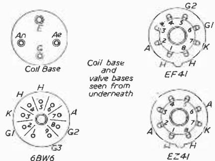
Fig. 7.—Details of valve base connections.
