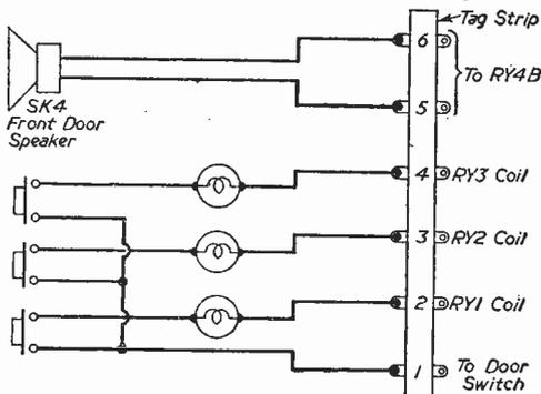
Fig. 4 (b)—Door unit wiring.
