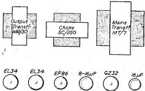
Fig. 17.—Diagram of the layout.
