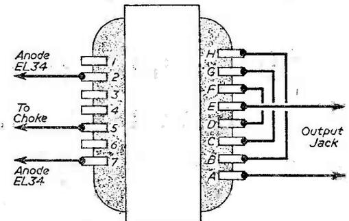
Fig. 14.—Output transformer details.
