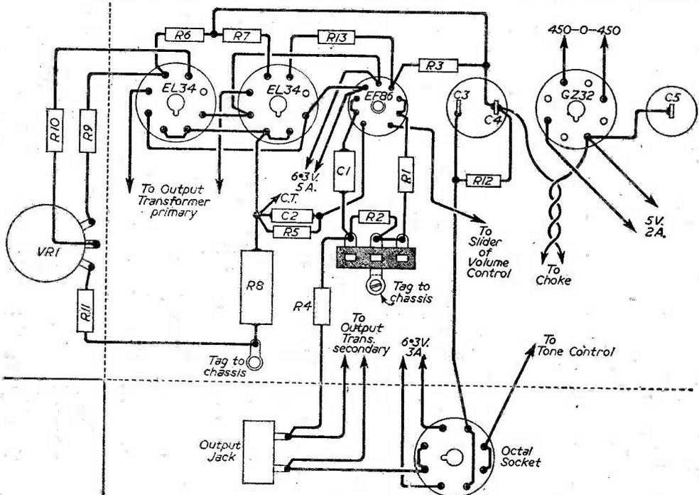
Fig. 16.—Wiring diagram of the 20-watt model.
