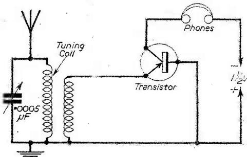
Fig. 1.—Transistor as detector-amplifier.
