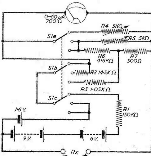
Fig. 3.—Circuit of an ohmmeter covering 100Ω to 5 MΩ in three ranges with a common scale.
