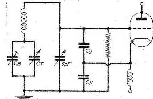
Fig. 9.—A 5 pF condenser connected as shown gives a "velvet vernier" control of a few Kc/s frequency shift in the Clapp V.F.O. circuit. CB is the "band-setter." CT is the usual tuning control.
