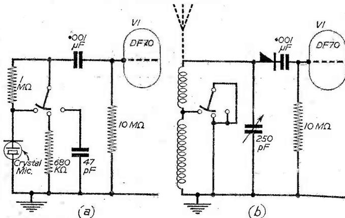
Fig. 1.—(a) The original input circuit; and (b) after conversion.
