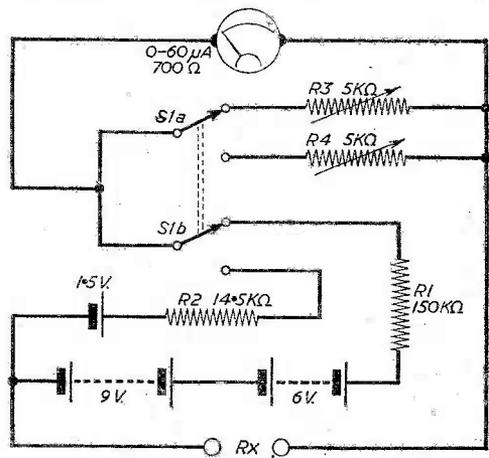
Fig. 2.—A simple circuit which measures from 1 KΩ to 5 MΩ in two ranges. Maximum current approximately 100μA. A single scale serves for both ranges.
