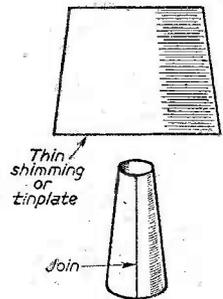
Fig. 10.—Gramophone spindle cone (if required).
