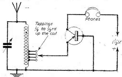
Fig. 2.—Using a tapped coil.
