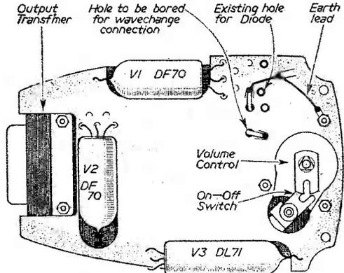
Fig. 3.—Rear of chassis after conversion.
