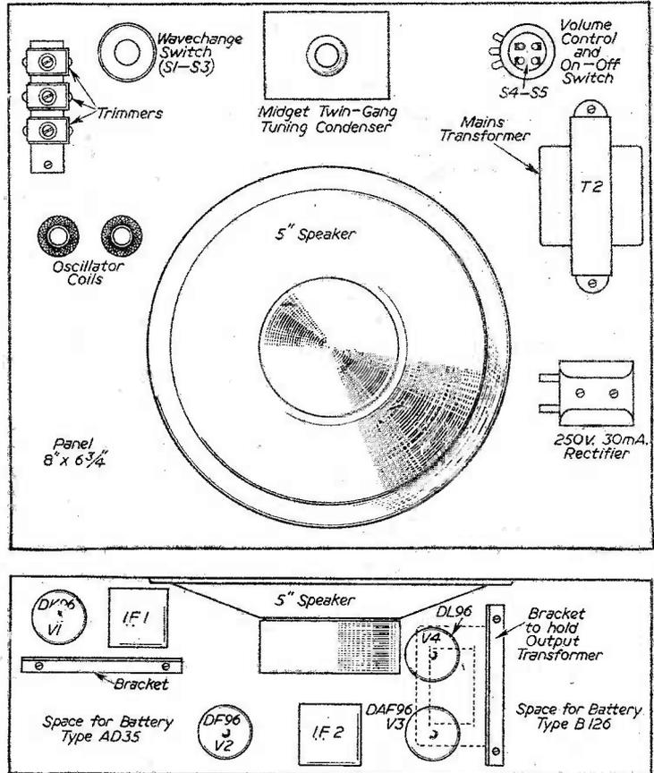
Fig. 3.—Main layout and plan view.
