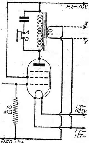
Fig. 5.—The output circuit. XY provides low impedance, and AB high-impedance outputs.
