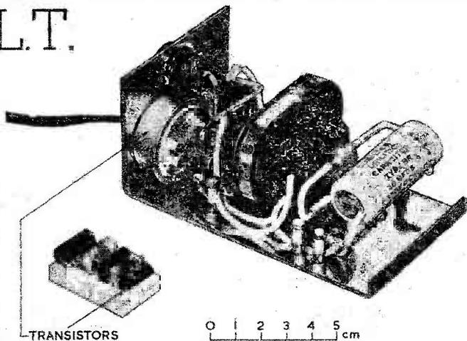
Converters with 2mW and 4 to 6W output.
