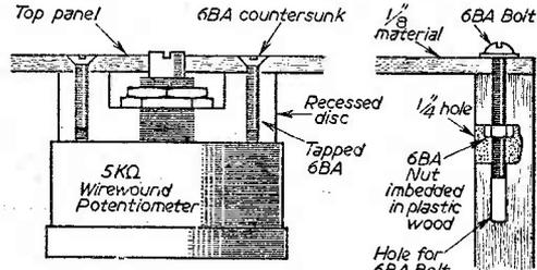
Fig. 8.—An unobtrusive method of mounting the pre-set potentiometers.
