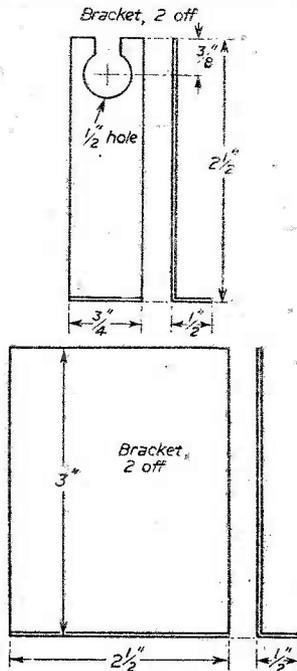
Fig. 2.—Details of the Ferrite Rod mount and bracket for output transformer.
