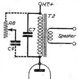
Fig. 8.—Fitting a tone control.
