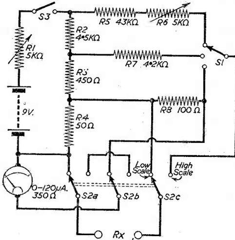
Fig. 10.—An ohmmeter circuit with four ranges which provides measurement between 1Ω and 2 MΩ. The lowest range has a separate scale.
