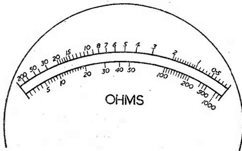
Fig. 12.—The two scales of the ohmmeter of Fig. 10. Mid-scale readings 5 (x 100, etc.) and 45Ω. The upper scale is for the three series ranges; the lower scale is for the lowest range, which uses the shunt method.
