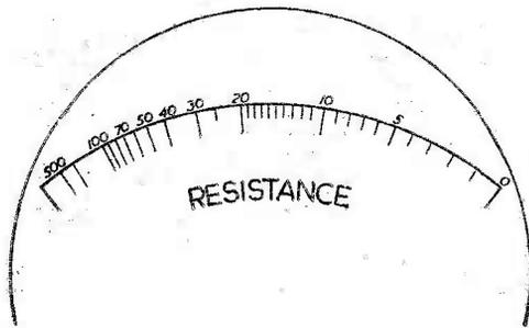
Fig. 4.—Scale of the ohmmeters of Figs. 2 and 3. Mid-scale value=15. On the different ranges are to be multiplied by factors of 100, 1,000 and 10,000 respectively to give ohms values.
