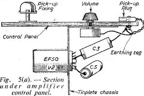
Fig. 5(a).—Section under amplifier control panel.
