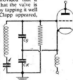
Fig. 1.—The Clapp oscillator.
