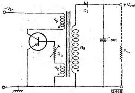
Basic circuit of ringing choke converter.
