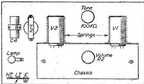
Fig. 5.—View of the underside of control panel.
