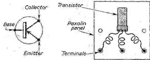
Fig. 7.—Transistor mounting.
