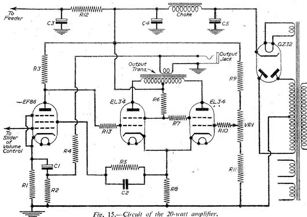
Fig. 15.—Circuit of the 20-watt amplifier.
