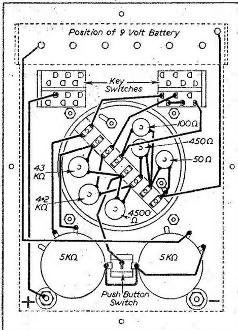
Fig. 7.—The reverse of the top panel, showing the components and some of the wiring.
