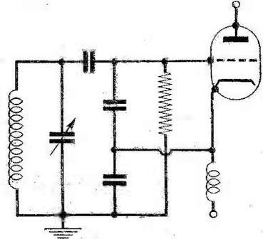
Fig. 2.—The "capacity tap" E.C.O.
