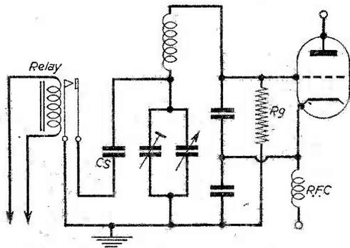
Fig. 10.—Between transmissions V.F.O. drift may be minimised by using a relay to switch in a detuning capacitor (CS). This shifts the V.F.O. frequency outside the band, but the V.F.O. valve still oscillates and therefore does not cool off during stand-by periods. After initial warming up the V.F.O. frequency during transmission becomes stable.
