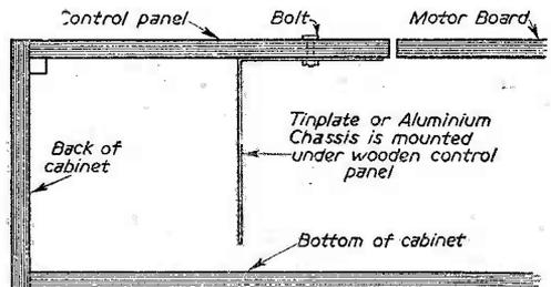
Fig. 4.—Details of the chassis—tinplate or aluminium.
