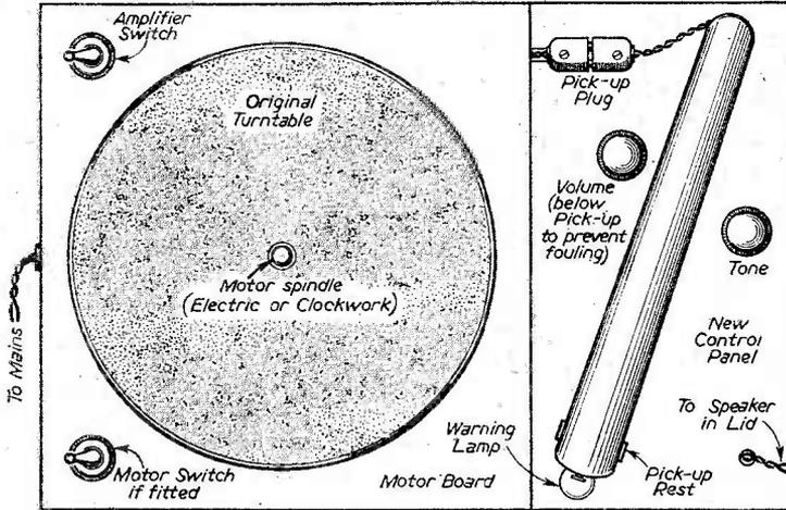
Fig. 3.—Plan of layout.
