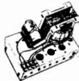
**POWER PACK** for F.M., etc. 40/- (2/- p. & p.). 220 v. at 50 mA. 6.3 v. at 2½ amps. Ditto with two valve amplifier, £5 (carr. paid). Ample volume. Separate top and bass controls.
