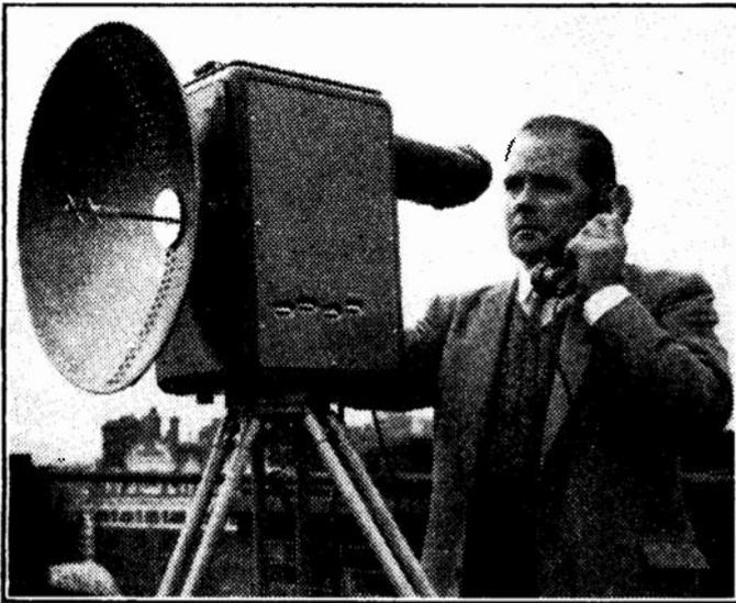
Testing the "Tellurimeter"—a micro-wave measuring instrument. It is claimed that this has an accuracy of 2in. to 6in. over distances ranging from 10 to 30 miles.
