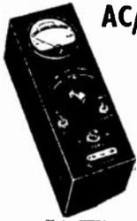
Complete 250 moving coil meter, scale graduated in A.C. P.C. volts, ohms and milliamperes. Voltage range A.C. D.C. 10, 0.1, 1, 10, 100, 1,000, 10,000. From panel, range switch, wire-wound potentiometer (zero setting) two toggle switches, resistors and meter resistor. In grey hammer-finish case.
