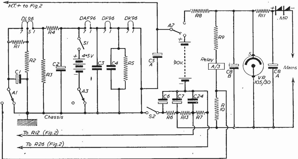
Fig. 1.—The power supply circuit.
