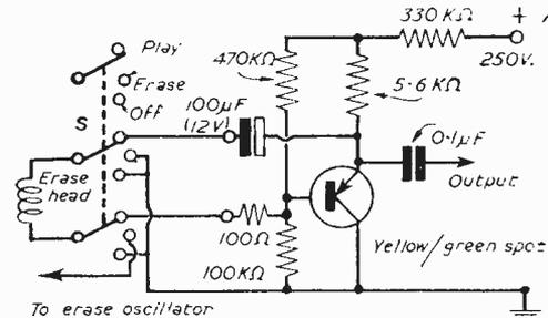
The tape recorder switching arrangement described by Mr. Dobson.
