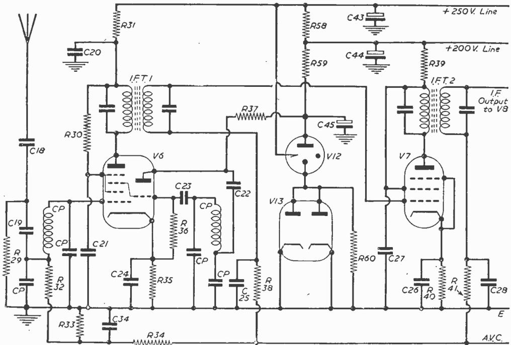
Fig. 1(a).—Circuit of the feeder section.
