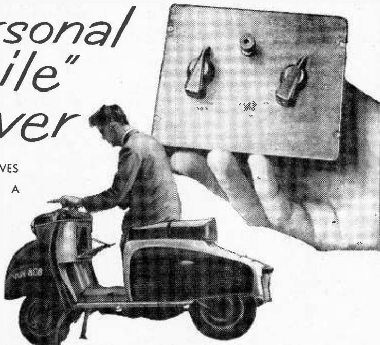
lead can be taken to scooter or car accumulator circuit to obtain current.
