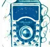
2,500 o.p.v. Multi range 6/30 120 300 1,200 v. A.C. ditto D.C. 0-1 K. 0-1 megohm 400 MicroA. 12 mA., 300 mA. -0 to +64 D.B. 5 ranges: 3in. x 4 1/2in. x 1 1/2in. Large clear dial. Leads supplied.
