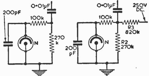
Fig. 3—A simple indicator circuit using a neon.
