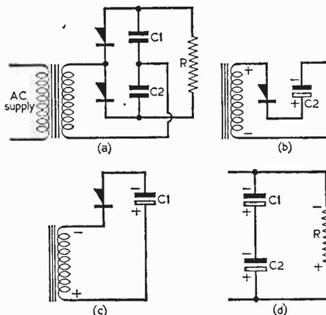
Fig. 14 (a)—The complete voltage doubler circuit. (b)—When the supply voltage is as shown in the diagram, C2 is charged. (c)—When the supply is reversed, C1 is charged as shown. (d)—This shows that the charges on C1 and C2 are in series and discharge through the load resistor R.
