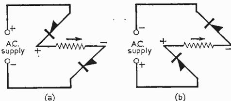
Fig. 13 (above)—These diagrams represent the actions of the bridge circuit of Fig. 12. Whatever the supply polarity, the load current is always in the same direction.
