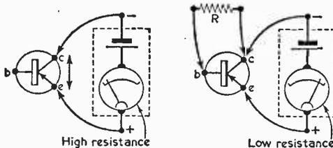
Fig. 8 (left)—Transistor leakage test.
