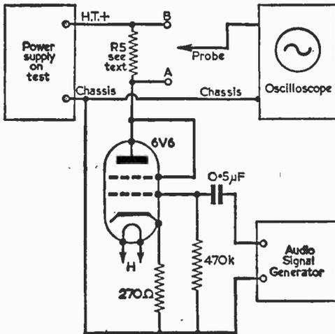
Fig. 5—Method of measuring dynamic internal impedance.
