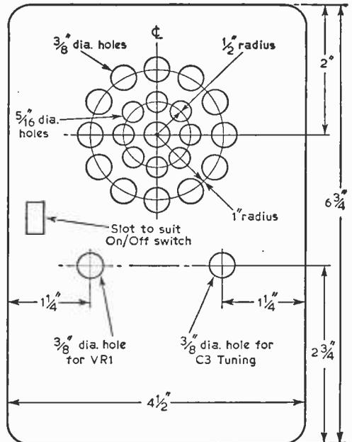
Fig. 3 (right)—The drilling details of the case.
