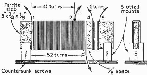
All coils wound with 28swg. D.C.C. copper wire
