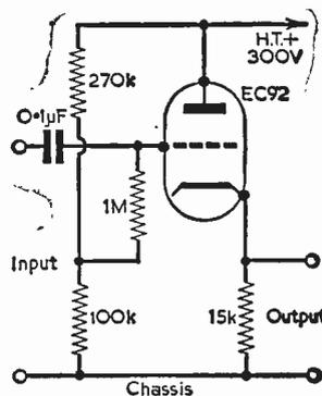
Fig. 6—A cathode-follower circuit, capable of handling peak 75V signals (positive or negative).
