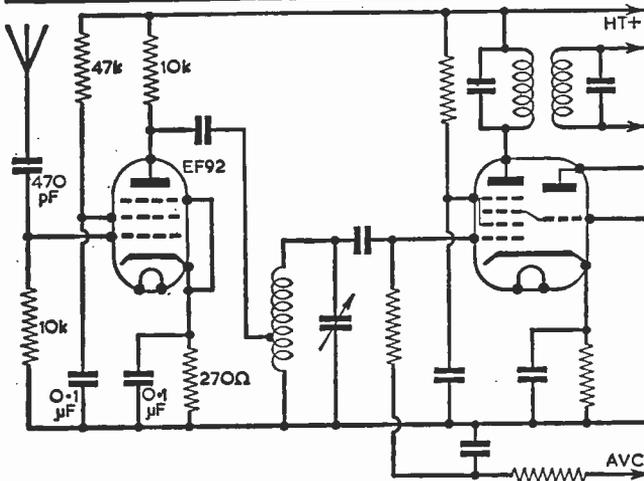
Fig. 5 (left)—A suitable improvement for the circuit of Fig. 4.
