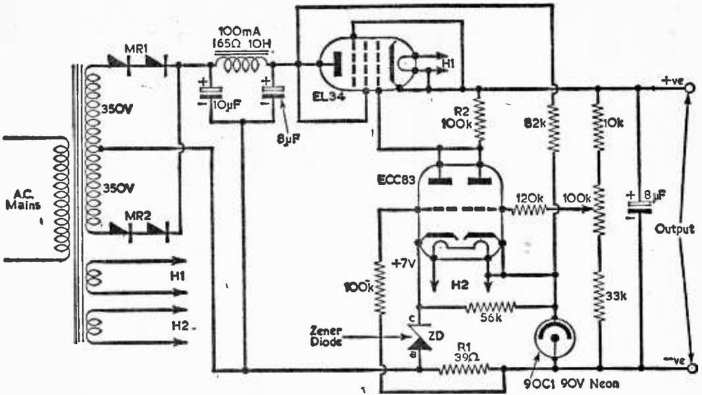
Fig. 2—The basic circuit with the addition of a current limiting device (which proved unsuccessful—see text).
