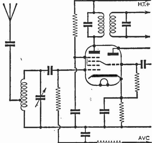
Fig. 4 (above)—A typical receiver input circuit which does not employ an aerial coupling coil.
