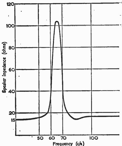
Fig. 1—A typical resonance curve for a 15Ω speaker with a 65c/s resonance.
