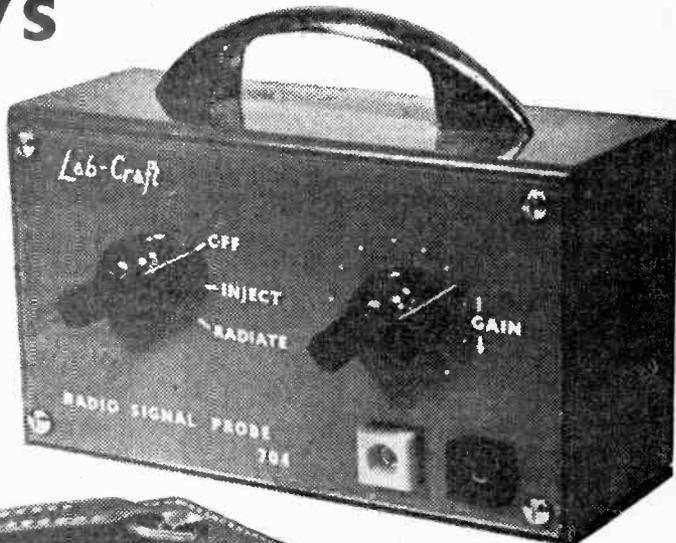
(Above)—The Lab-Craft radio signal probe—Model 704.
