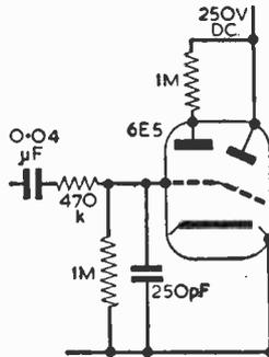
Fig. 1—In this circuit, the grid of the magic eye is connected to an audio connection in the recorder.
