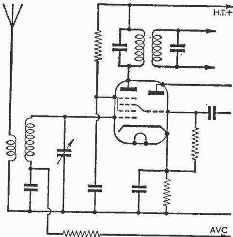
[Fig. 1—A typical receiver input circuit.
