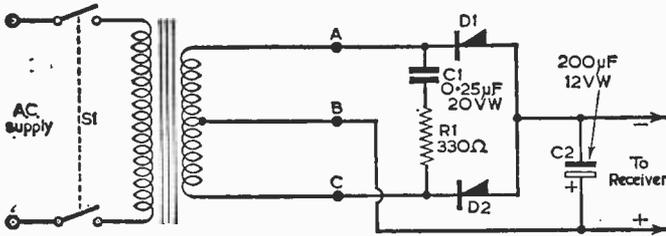
Fig. 1—This circuit is suitable for running a transistor portable receiver from the mains supply (see text).
