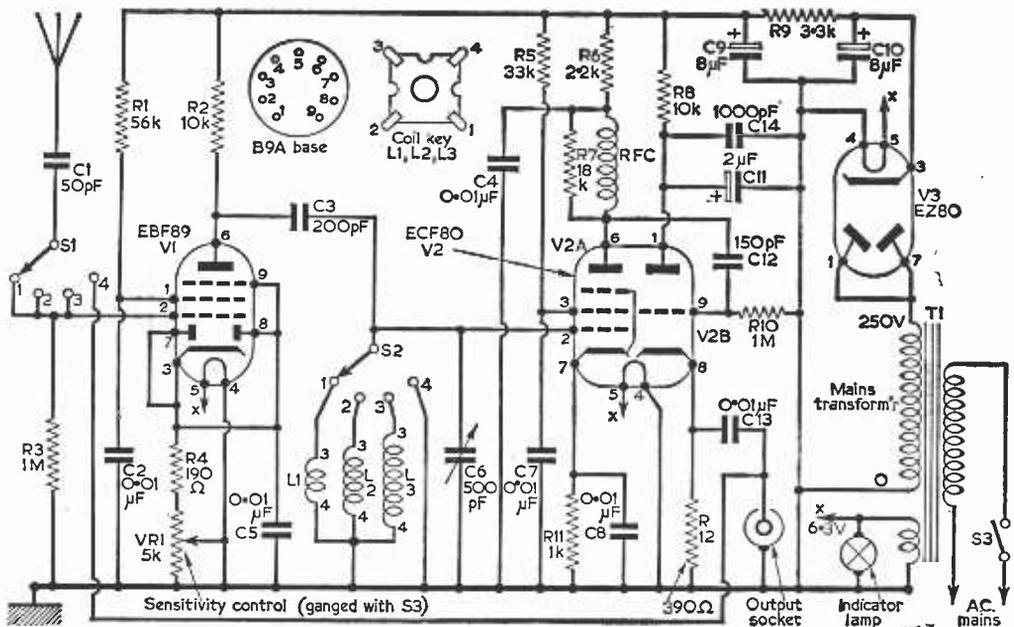
Fig. 1—The complete circuit.
