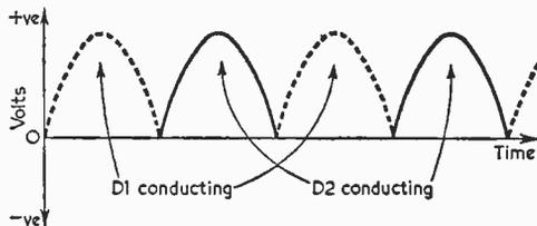
Fig. 10—This represents the output voltage from a full-wave supply, without a reservoir capacitor or smoothing components.
