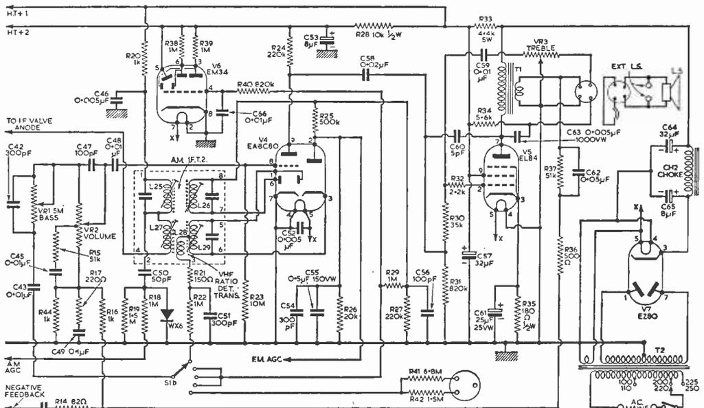
Fig. 9—The circuit diagram of the detector, AGC, A.F., output and rectifier stages of a combined A.M./F.M. receiver.
