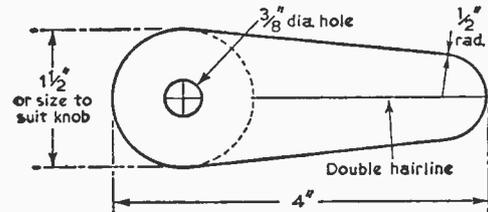
Fig. 6—The dimensions of the cursor.
