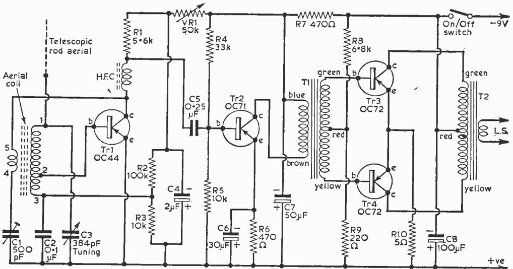
Fig. 1—The circuit of the receiver.
