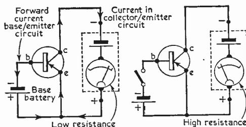
Fig. 5 (left)—The action of forward current in the base-emitter circuit gives a reduction in the apparent resistance between the collector and emitter.
