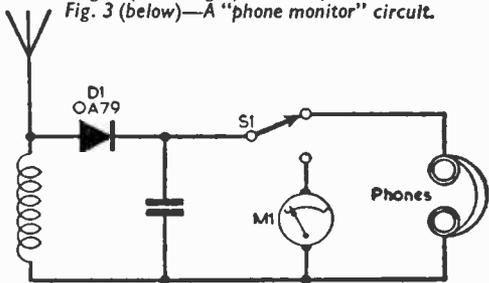
Note: The "Loop" is joined to the circuit by a length of coaxial cable
