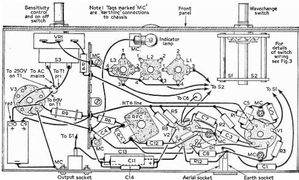
Fig. 2b—The under-chassis layout and wiring diagram.
