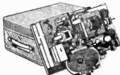
**SELF-POWERED VHF TUNER CHASSIS.** Covering 88-95 Mc/s. Mullard permeability tuner. Dims. 10 1/2 x 4 1/2 x 5 1/2 in. high ECC85, EF91, EF91 and 2 diodes. Metal Rectifier. Mains transformer. Fully wired and tested. Only £7.14.0 (carr. pd.). Room dipole 10'—300 ohm twin feeder. 6d. yd. Tuner without power pack £6.14.0 (carr. paid).
