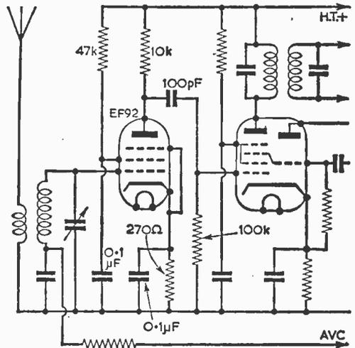
Fig. 2—The circuit of Fig. 1 with an R.F. stage added.
