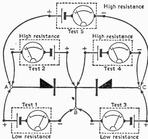
Fig. 1—How a series of ohmmeter tests indicates that a transistor contains two diodes connected in series opposition. (Test 6 is the same as Test 5, but with the ohmmeter leads transposed.)
