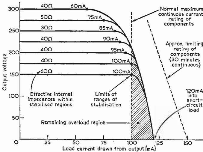
Fig. 4—Performance graph of the circuit of Fig. 3 with R1 having a value of 185Ω. (When R1 was made 150Ω, merely the overload region was increased, so that the short circuit current was 147mA; when R1 was made 200Ω, the overload region was entirely removed, and the short circuit current was only 110mA, or less. However, cut-off then encroaches on the available stabilised region. It may thus be seen that R1 is critical and that 185Ω is the optimum value.)
