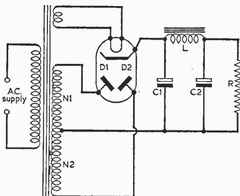
Fig. 9—A complete H.T. full-wave rectifier circuit.
