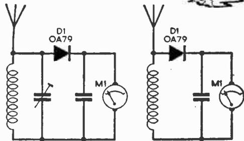
Fig. 1 (above left)—A field strength indicator circuit. Fig. 2 (above right)—A modified circuit. Fig. 3 (below)—A "phone monitor" circuit.
