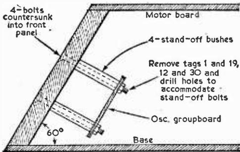
Fig. 22—The method of mounting the oscillator group board on the front panel of the cabinet.
