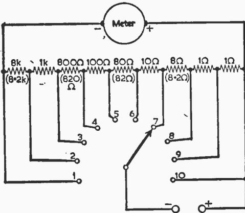
Fig. 1—A circuit of a switched universal shunt. The figures in brackets are preferred values of components which may be used if extreme accuracy is not essential.
