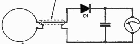
Loop...3 turns 2" diam. of PVC. covered wire
