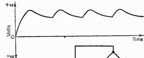
Fig. 11 (above)—The output voltage from a full-wave circuit with a reservoir capacitor.
