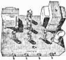
A kit designed to meet the exacting requirements of the audio enthusiast, yet remain within the price range of the average constructor. A stylishly finished monaural amplifier with an output of 14 Watts from 2 EL84's in push pull. Super reproduction of both music and speech
