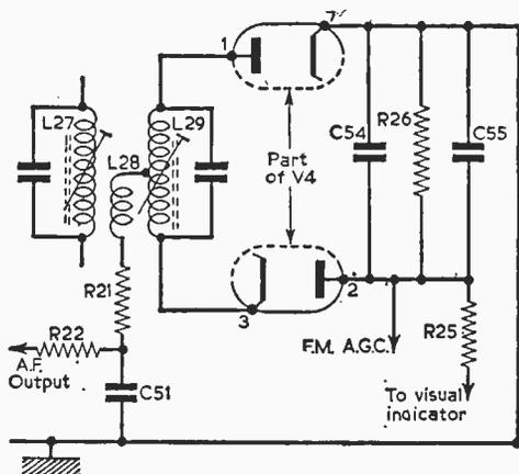
Fig. 10—The ratio detector section from the receiver shown in Fig. 9 with the same component references.
