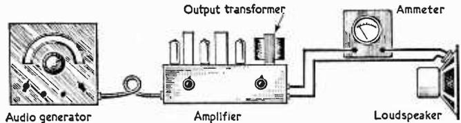
Fig. 3—Determining the fundamental resonant frequency of a loudspeaker.
