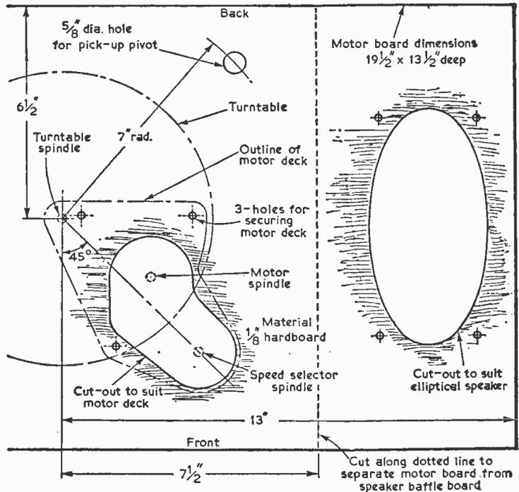
Fig. 23—Dimensions of the motor board and its cut-outs.
