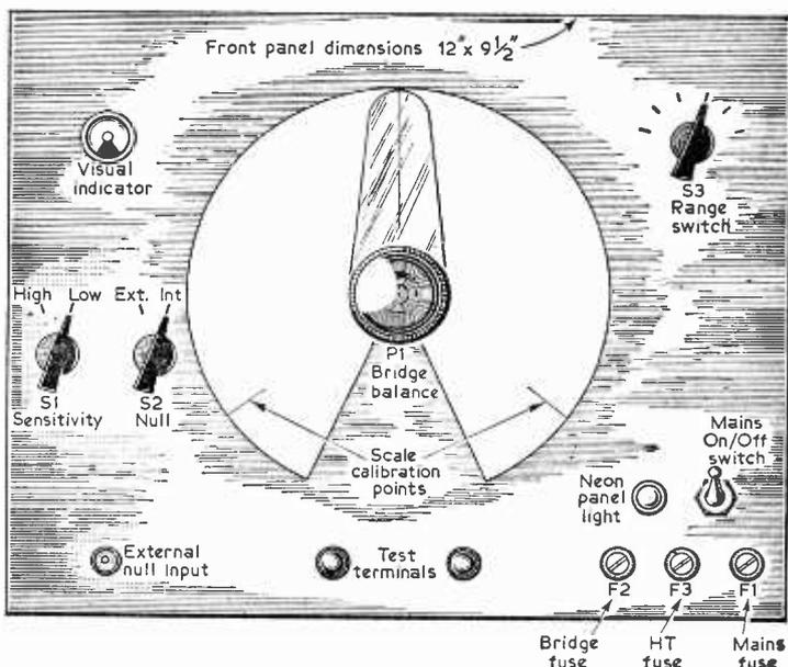
Fig. 5—The layout of the front panel.
