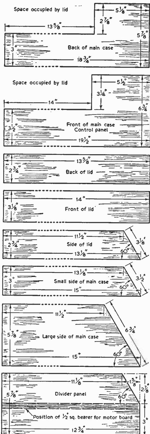
Fig. 21—Dimensions of the softwood sections of the cabinet. (Note: the lid requires only three sides—see Fig. 20.)
