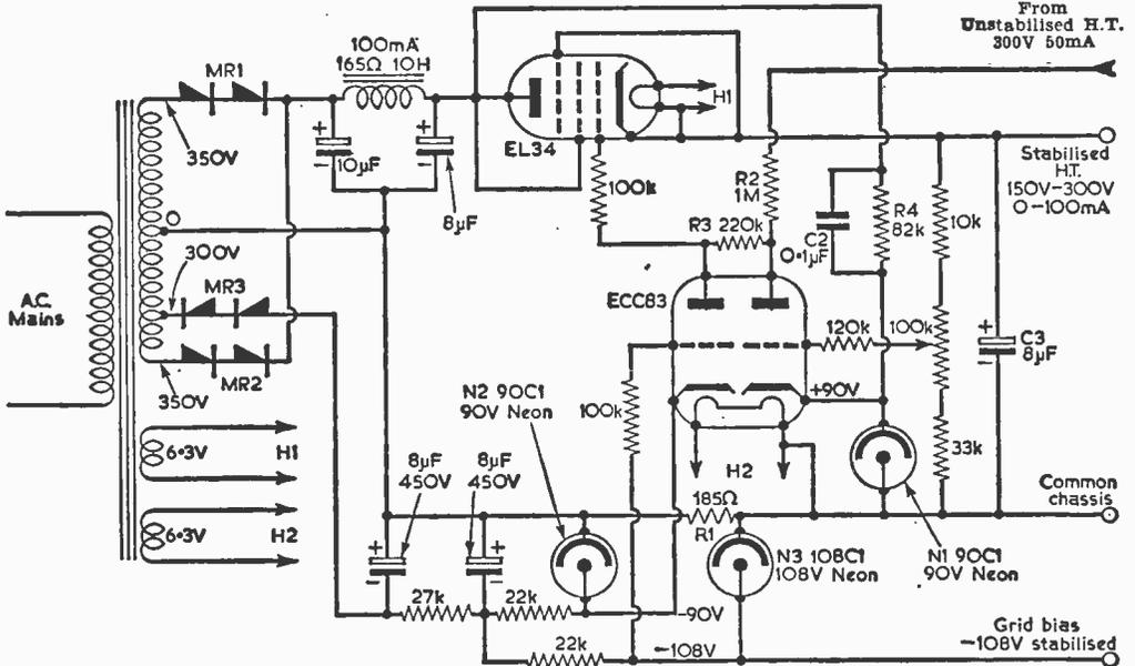
Fig. 3—The advanced stabilising circuit with the addition of an effective current limiting circuit.
