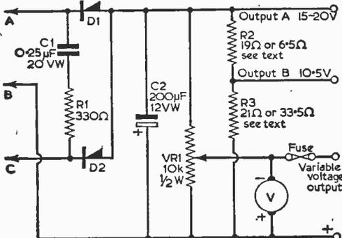
Fig. 2—A workshop supply unit with variable outputs.
