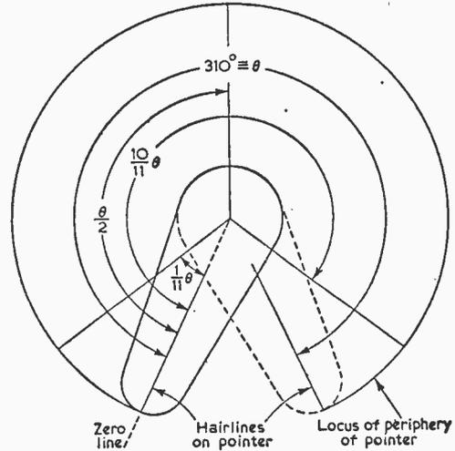
Fig. 7—The method of marking the scale.
