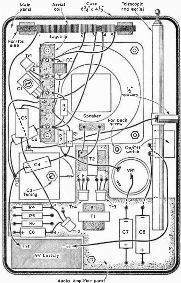
Fig. 4—The internal layout of components.
