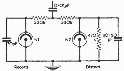
Fig. 5—A circuit using two neons; one for record and one for over-record.
