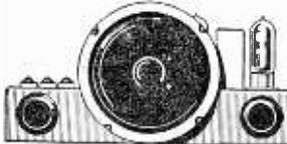
4 Mullard valves, 5in. speaker, frame aerial, 4 pre-set stations, 1 long, 3 med. wave, superhet circuit. BRAND NEW. Size 9 x 6 x 5 1/2 in. high. Tested by us ready for use. 200/250 v. A.C.-D.C. Mains.
