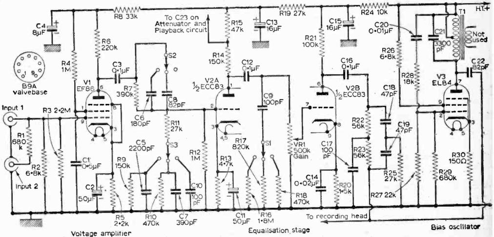
Fig. 13: The main amplifier circuit.
