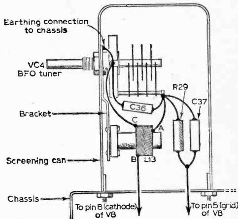
Fig. 5 (above)—The beat frequency oscillator.
