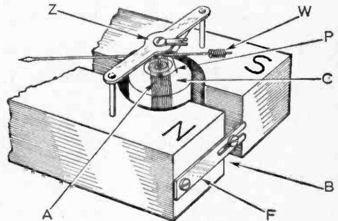
Fig. 1—A typical meter movement.
