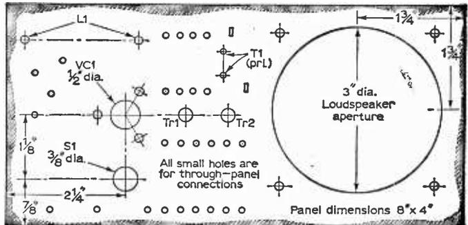
Fig. 2—Drilling details of the panel.
