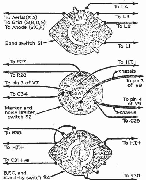
Fig. 4—Details of the switch wiring.
