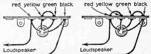
Fig. 4 (left): Loudspeaker/output transformer connections for 15Ω speaker.
