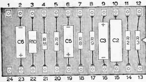
Fig. 2: The front of the group board wiring.
