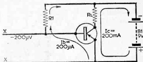
Fig. 3: The battery, B2, of Fig. 2 is replaced here by a resistor.
