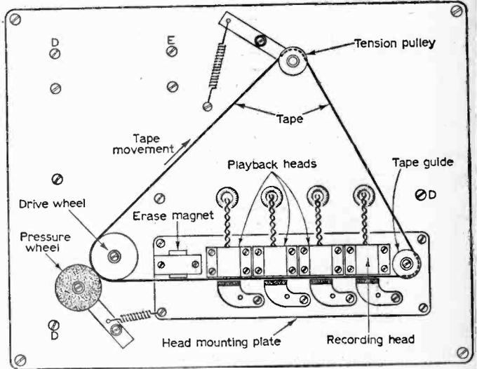
Fig. 12: The completed deck.
