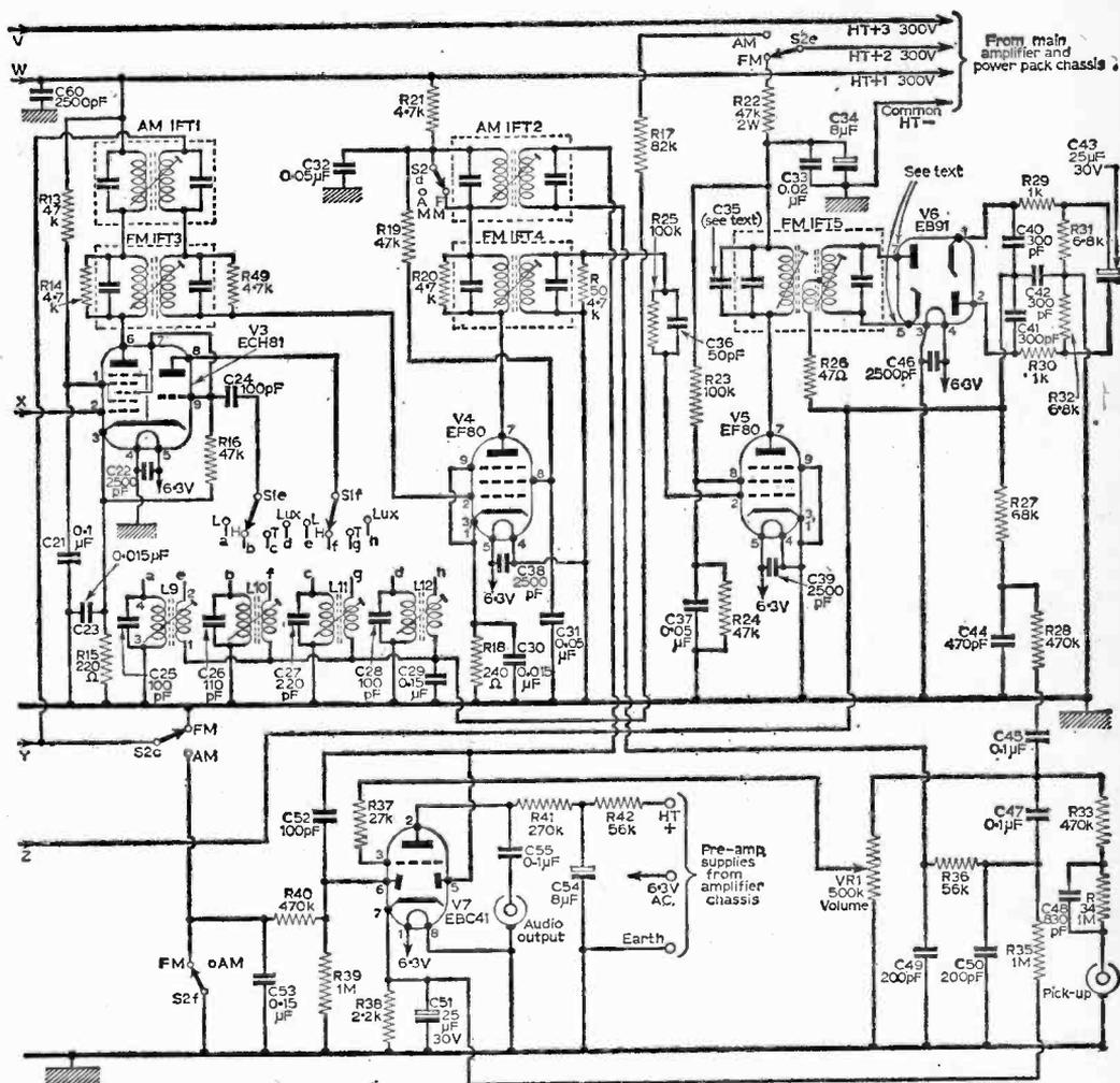
Fig. 9b: The i.f., detector and audio stages of the circuit.
