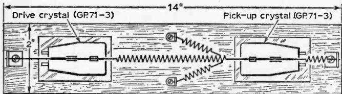
Fig. 5 (above): Top view of delay unit.
