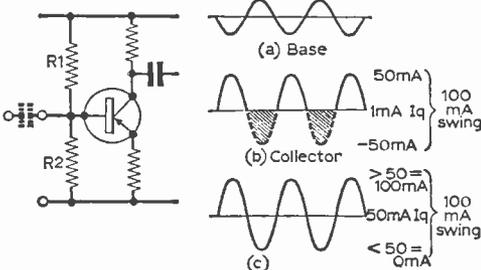
Fig. 1: Common-emitter amplifier.
