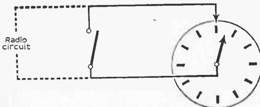
Fig. 1—Showing how the on-off switch of the radio is replaced by the hour hand of the clock. The bottom lead does not need to be connected to the spindle as metallic contact through any part of the frame suffices.
