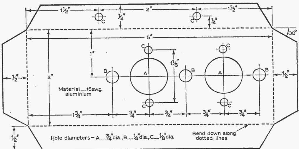
Fig. 3: Chassis drilling details for the receiver unit.
