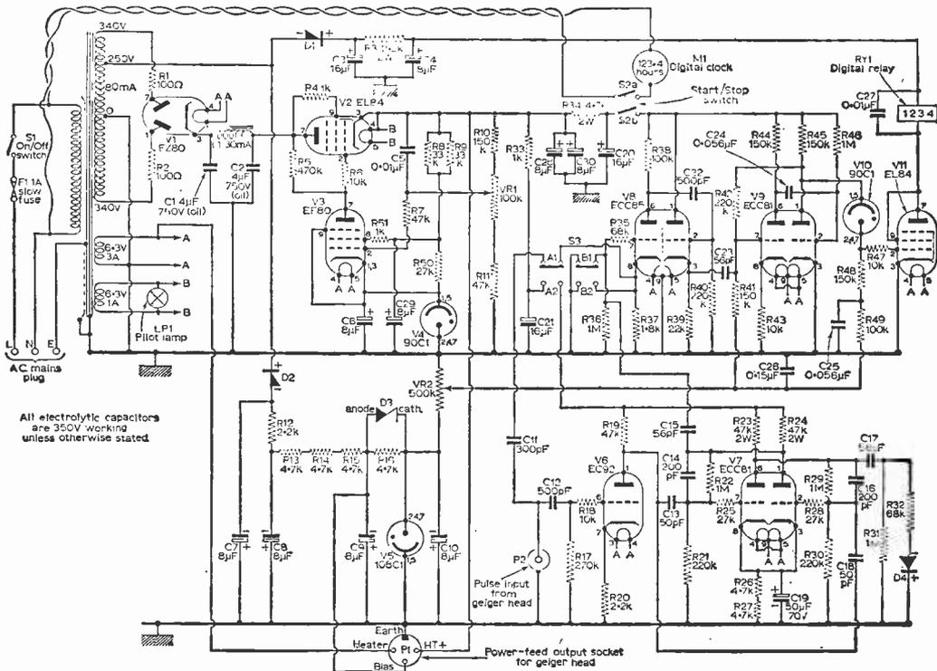
Fig. 1: The complete theoretical circuit of the digital register.
