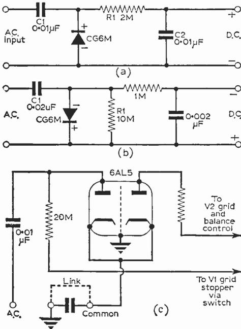
Fig. 14: Typical examples of crystal and valve probes.
