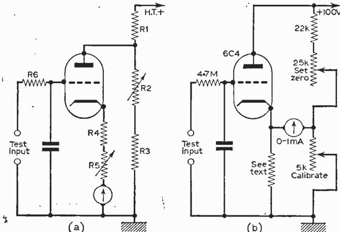
Fig. 12: The use of a valve to amplify an applied voltage and give a meter indication.
