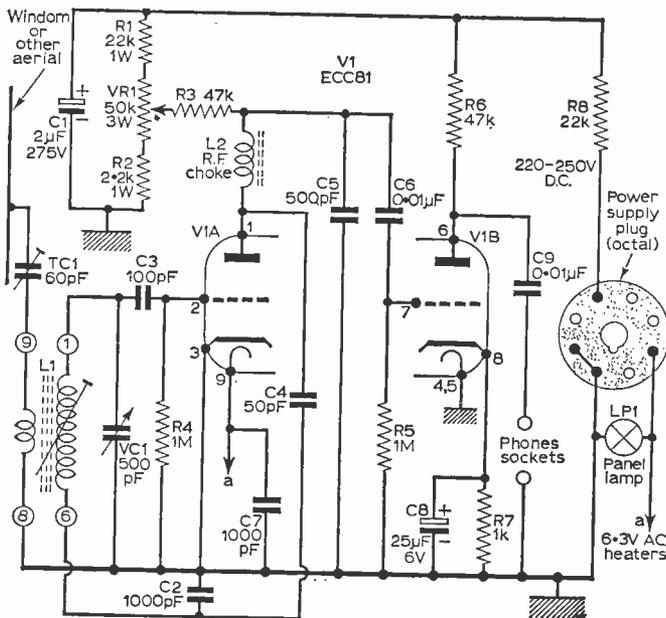
Fig. 1: The circuit diagram of the receiver unit.
