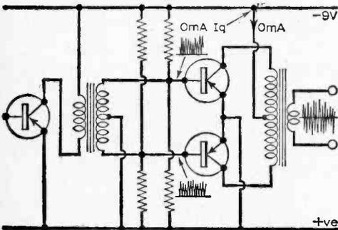
Fig. 8: Transformer phase-splitter.
