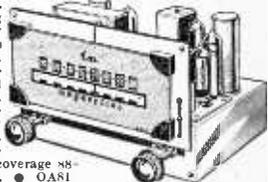
**6 TRANSISTOR AND DIODE SUPERHET**
