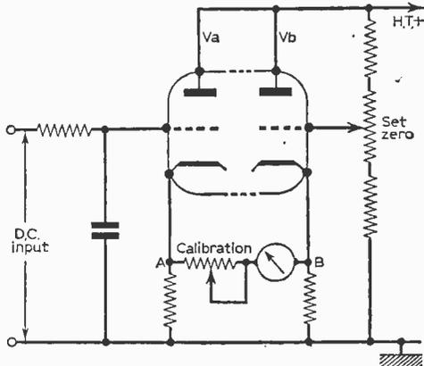
Fig. 10: Basic circuit of a valve voltmeter.
