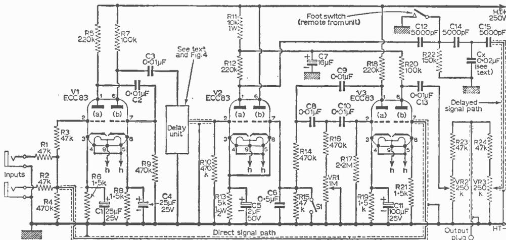
Fig. 2: The circuit diagram of the Echo Unit
