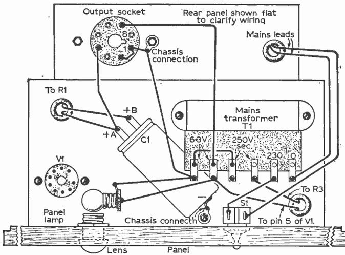
Fig. 9: The above-chassis layout of the power-pack
