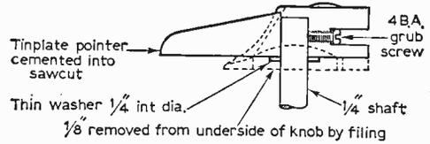
Fig. 7: Section through modified pointer knob.
