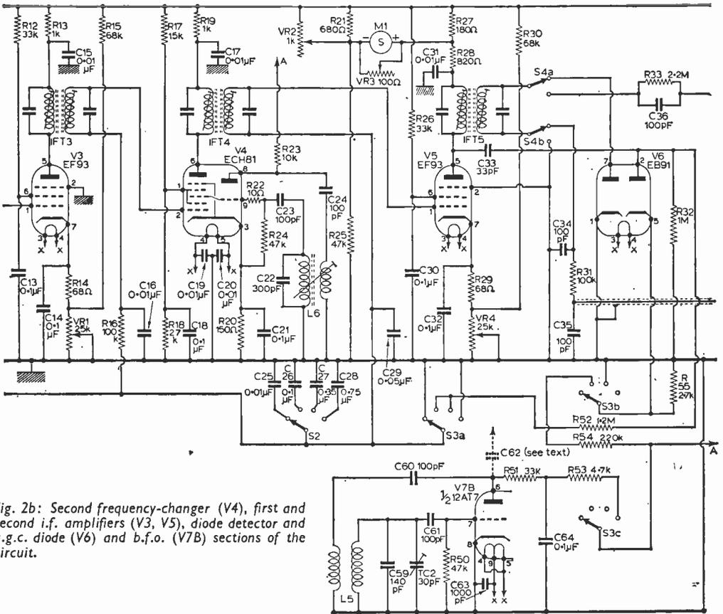
Fig. 2b: Second frequency-changer (V4), first and second i.f. amplifiers (V3, V5), diode detector and a.g.c. diode (V6) and b.f.o. (V7B) sections of the circuit.
