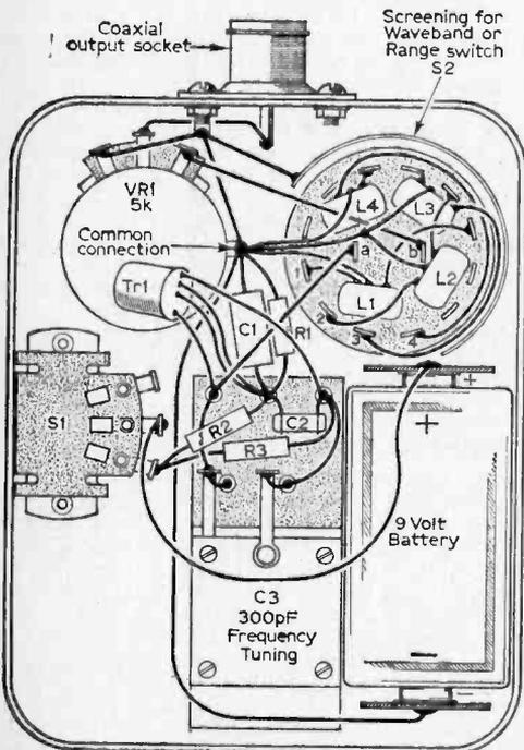
Fig. 2: Interior view showing layout and wiring.
