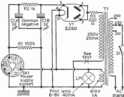
Fig. 7: The circuit of the power unit.
