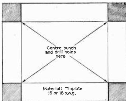
Fig. 1: Cutting the chassis.
