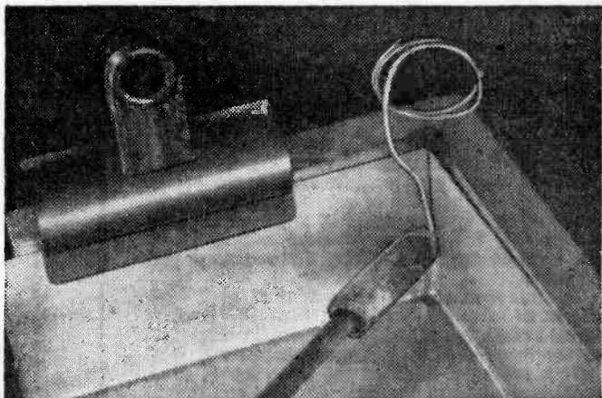
Fig. 3: Soldering the corner joints.
