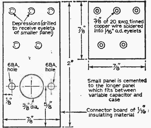
Fig. 5: Connector board, made up of 1/16 in. insulating material.
