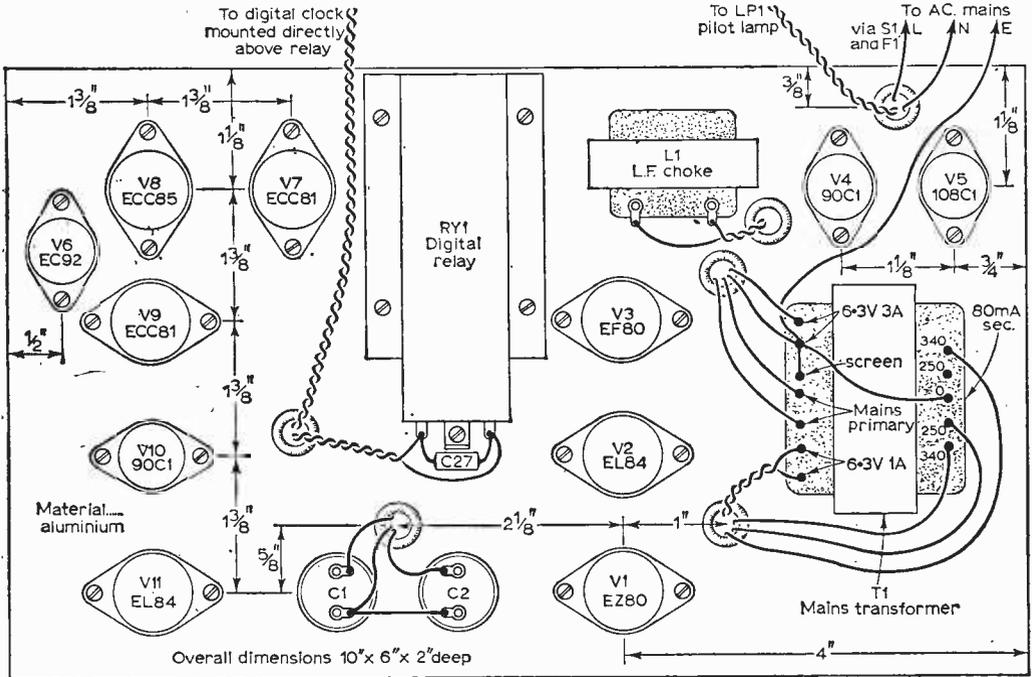
Fig. 3: Above-chassis layout and wiring, showing main drilling dimensions.
