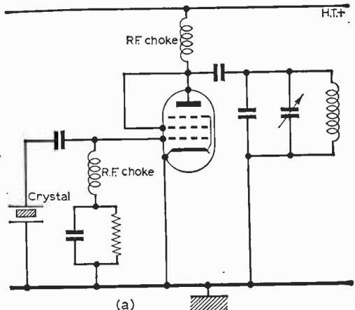
Fig. 19a (above): A simple crystal oscillator circuit.
