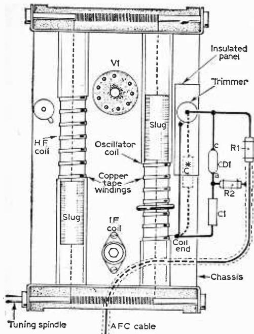
Fig. 13: The connections of the a.f.c.-components on the f.m.-head.
