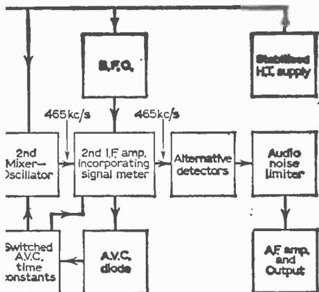
Another EF95 strapped as a triode serves as the first oscillator, giving the high output needed for optimum conversion efficiency, this factor being maintained over the whole frequency band by the loading of the oscillator anode with an r.f. choke, L4. The output to the mixer is taken from the top of the anode circuit, this once again reducing any tendency towards "pulling", although in some cases it might be necessary to take the output from the oscillator anode (see paragraph on alignment).
