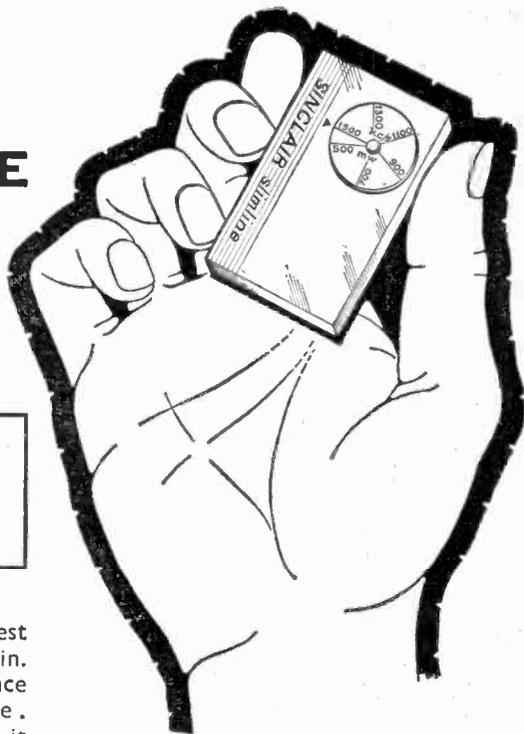
The **Sinclair Slimline** is the smallest receiver of them all, only  $2\frac{3}{4} \times 1\frac{5}{8} \times \frac{5}{8}$  in. Yet it far surpasses in performance sets many times as large. Using only its internal ferrite rod aerial, it will receive all stations on the medium wave band including **Home, Light, Third, Luxembourg** and dozens of continental transmissions.
