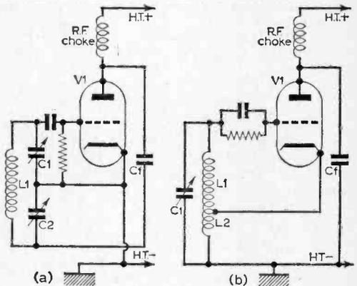
Fig. 17a: Colpitt's oscillator; b: the Hartley oscillator.
