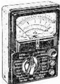
20,000 O.P.V. MODEL TP-5S. Reads voltage up to 1,000 D.C. at 20,000 ohms per volt and A.C. at 10,000 o.p.v.; D.C. Current to 500mA; Resistance to 10 Megs.; Capacitance to 0.1µF; Decibels from -20 to +36. Size 3 1/4 in. x 5 1/4 in. £5.19.6.
