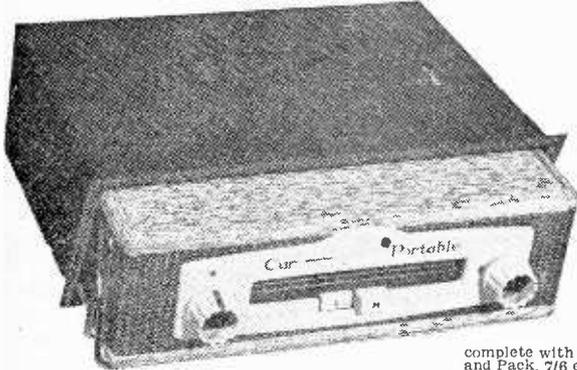
Battery drain is exceptionally low—the life of the self-contained battery within the set is approx. 200 hrs. Transistors used: 1 OC44; 2 OC45; 1 OC82D; 2 OC82 and Diode. Compares with set costing at least double. Properly installed this set will give you years of pleasure and service both in and out of your car.
