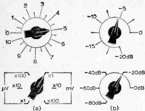
Fig. 20: Two examples of attenuator control markings.
