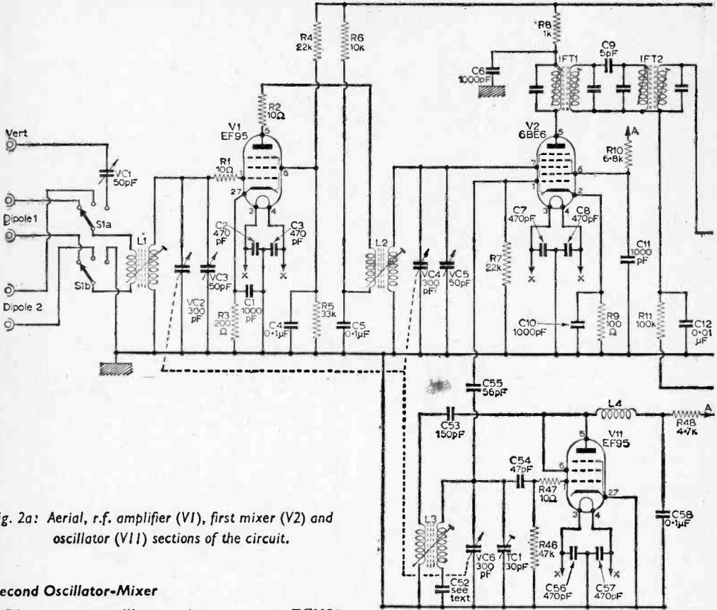
Fig. 2a: Aerial, r.f. amplifier (V1), first mixer (V2) and oscillator (V11) sections of the circuit.
