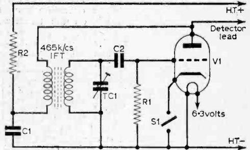
Fig. 1: The circuit of the unit.
