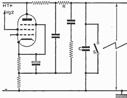
Fig. 3(c): Cathode follower, basic circuit.
