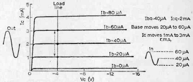
Fig. 3: This shows how a magnified version of the input current waveform appears in the collector circuit.
