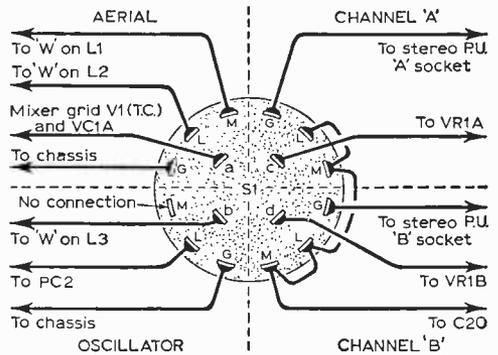
Fig. 5: The wiring of the wave-change/gram switch.
