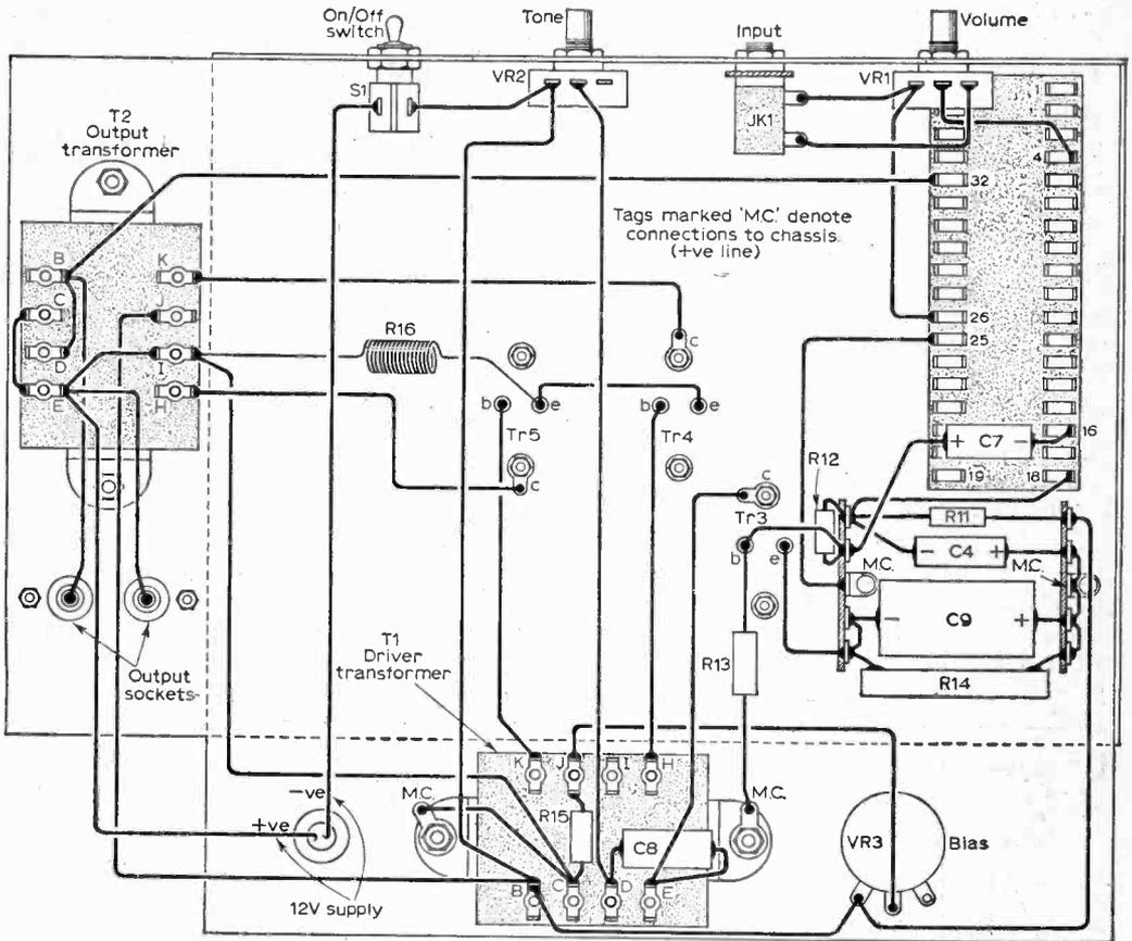
Fig. 2: The underchassis wiring diagram.
