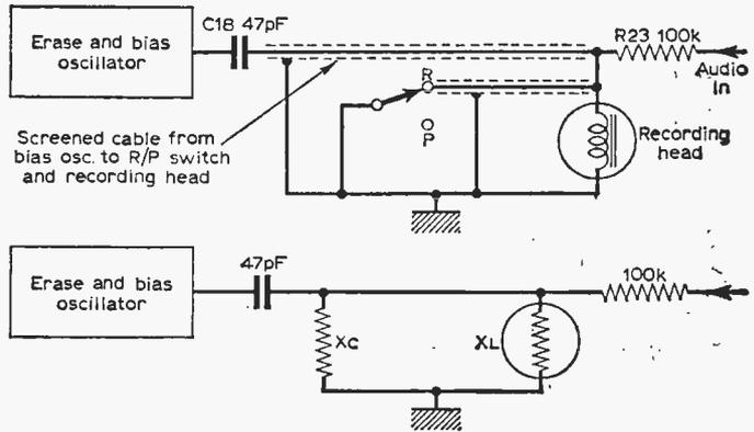
Fig. 5: Illustrating the effect of a long cable on bias power. Ordinary screened cable has a capacity of about 50pF/ft. If one foot of such cable is used at 60kc/s then Xc=50kΩ and XL=60kΩ, thus half the bias power will flow through the cable.
