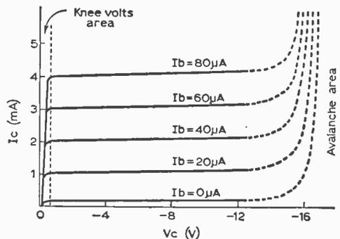
Fig. 1: Family of output-characteristic curves.
