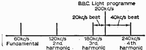
Fig. 7: Relationship between the frequencies of the bias oscillator and the broadcast station.
