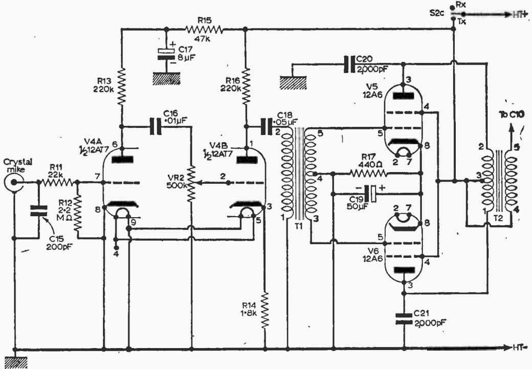
Fig. 2: The modulator stage of the circuit.
