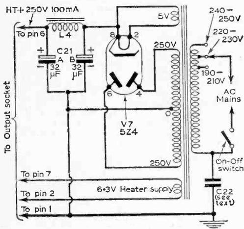
Fig. 6: The circuit of the power supply.
