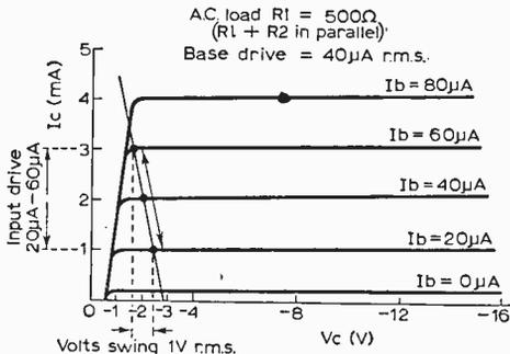
Fig. 6: The graph modified for an effective load of 500Ω.
