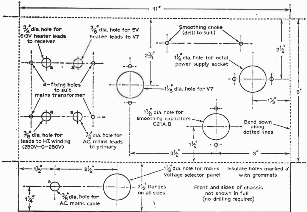
Fig. 7: The dimensions of the power supply chassis.
