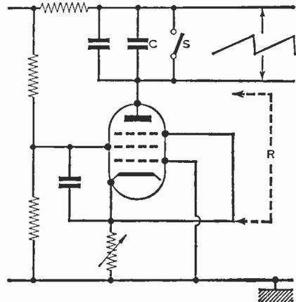
alternative circuits, but this is not the place to enter into a discussion—even a controversy—about oscillator design. Perhaps the most popular method of obtaining a “linear” sawtooth of sufficient output, with short flyback, is the Miller Transitron and this will be discussed at greater length.
