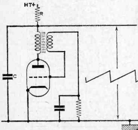
Fig. 3(g): Blocking oscillator timebase.
