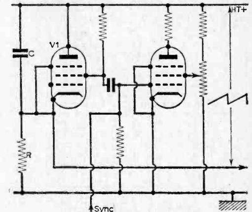
Fig. 3(f): Two-valve timebase with one pentode as feedback element and the other as switch.
