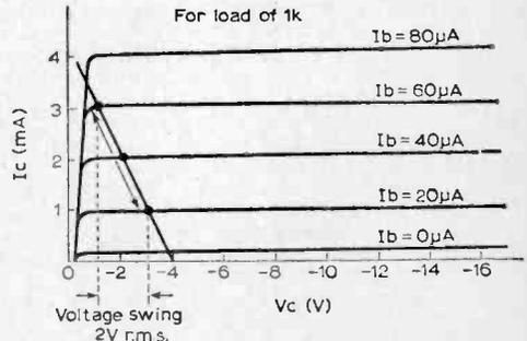
Fig. 4: Loadline for collector load of  $1k\Omega$ .
