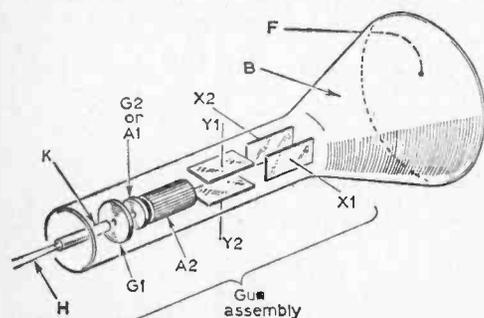
Fig. 1: Schematic view of electrostatically focused c.r.t.
