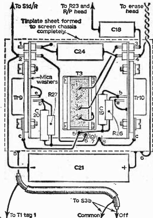
Fig. 6: Layout of the erase oscillator.
