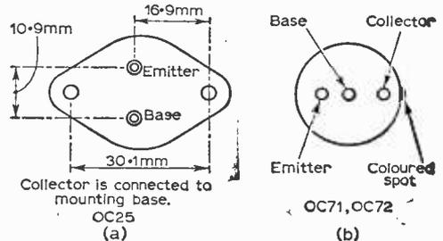
Fig. 6: Transistor connection details.
