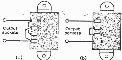
Fig. 5: Output transformer connections for (a) a 3Ω loudspeaker, (b) a 15Ω loudspeaker.
