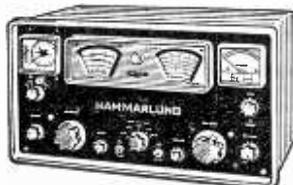
General coverage 540 Kc/s-30 Mc/s in four bands. Band-spread facilities for amateur and other bands. BFO, Noise Limiter, "Q" Multiplier, 10 tubes. Provision for phones and loudspeaker (3 ohms). Complete with "B" Meter 280 (clock extra if required).
