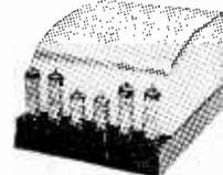
source, inputs—Microphone 5 mV, Tape 5.3 mV, R.L.A.A. 4.3 mV, flat 250 mV, Tuner 100 mV. Valve line-up: 2—EF86, 4—ECC83. Power Amplifier—14 watts per Channel, sensitivity 1 volt r.m.s. for 14 watts output, frequency response  $\pm 0.5db$  20 c/s.—20 Kc/s. Speaker impedance 4, 8 or 16 ohms. surplus power available for Tape Pre-Am. mains supply 105/240 v. A.C. Valve line-up, 2—ECC83, 4—EL84, 1—GZ34.
