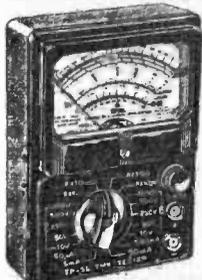
**20,000 O.P.V. MODEL TP-5S.** Reads voltage up to 1,000 D.C. at 20,000 ohms per volt and A.C. at 10,000 O.P.V.; D.C. Current to 500mA; Resistance to 10 Megs.; Capacitance to 0.1µF; Decibels from -20 to +36. Size 9 1/2 in. x 5 1/2 in. x 1 1/2 in. **£5.19.6**
