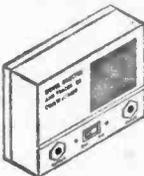
The first combined transistorised signal injector plus signal tracer in same case. Injector covers 2 K/c to 2 M/c. Tracer has R.F. detector. Separate flexible probes. Small battery lasts months. Easy to assemble with all diagrams provided.
