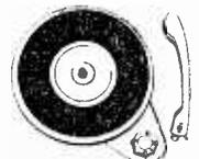
Heavy 8 1/2 in. metal turntable. Low flutter performance 200/250 v. shaded motor with tap at 45v. for amplifier valve filament if required. Turnover LP/78 head.
