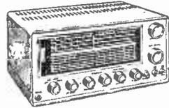
4 bands covering 550Kc/s to 30Mc/s (continuous). Operation 200/240 volt A.C. Special features include: Easy to read illuminated slide rule dial—Built in Q multiplier—Aerial trimmer—calibrated electrical bandsread on amateur bands—0-100 logging scale—noise limiter—AVC/MVC B.F.O. for clear CW and SSB reception—built in edgewise "S" meter. Output for phones or STD speaker. Supplied brand new and guaranteed with manual. £42 carriage paid. S.A.E. for full details. Part exchange welcome.
