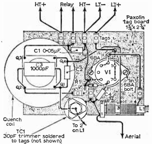
The receiver is built on a tag board or paxolin panel, refer to the layout shown in Fig. 6. Leads to the 27Mc/s coil, 30pF trimmer, valveholder, and 100pF and 200pF capacitors must be very short and direct. The quench coil can be held with a woodscrew.
