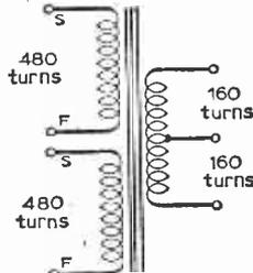
Fig. 4: Winding details for the driver transformer, T1.
