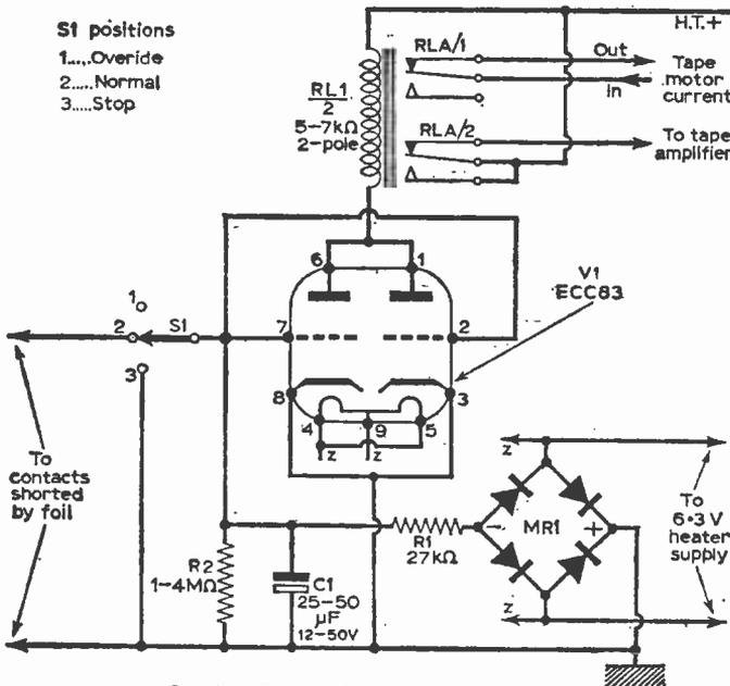
Fig. 1: The simple circuit of the device.
