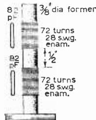
Fig. 2: Winding details of the 3.0Mc/s i.f. transformer.
