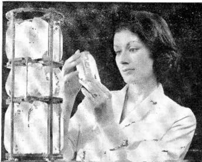
The quartz crystals shown in this illustration were grown in three weeks at STC's factory at Harlow.
