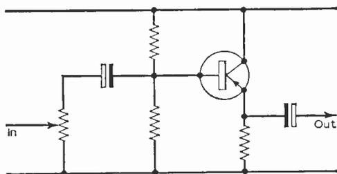
Fig. 1: A transistor in the emitter-follower configuration.
