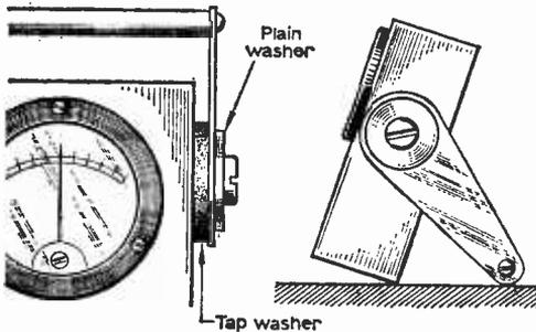
Fig. 11: Illustrating a suitable handle, for the meter which may double as an inclined support.
