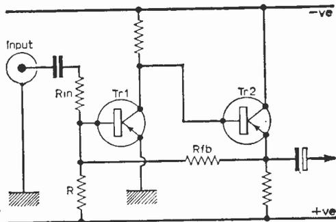
Fig. 2: The basic arrangement for a "Bow's brick" circuit.
