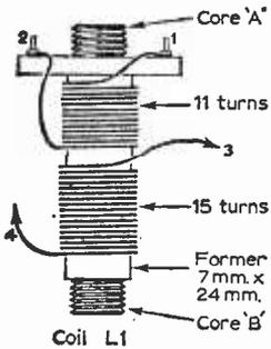
Fig. 4 (left): Winding details of the 27Mc/s coil.
