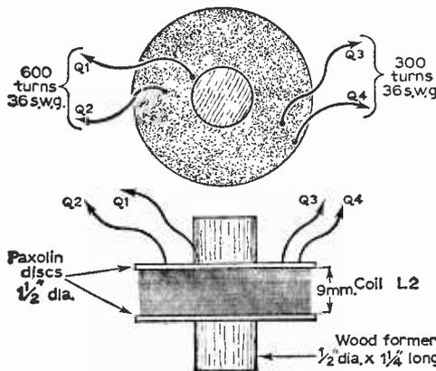
adjusting its core and the 30pF trimmer TC1. Regeneration is obtained from the feedback winding which is coupled to L1.
