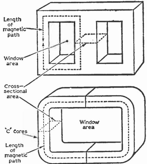
Fig. 5: Critical measurements for the transformer cores.
