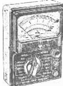
**20,000 O.P.V. MODEL TP-5S.** Reads voltage up to 1,000 D.C. at 20,000 ohms per volt and A.C. at 10,000 O.P.V.; D.C. Current to 500mA; Resistance to 10 Mers.; Capacitance to 0.1µF; Decibels from -20 to +30. Size 3½in. x 5½in. x 1½in. **£5.19.6**
