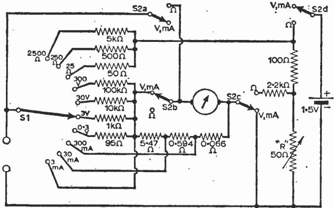
Fig. 10: The complete multimeter circuit.
