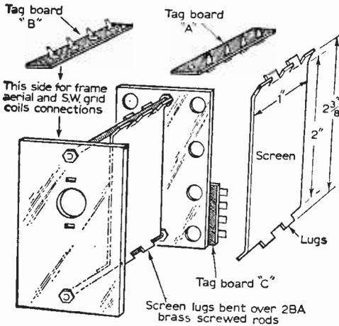
The diagrams are fully dimensioned, although generally sizes have been given for centres. Diameters of holes should be checked with the actual components to be used. Sometimes makers provide templates and these should be used for marking—this applies particularly to i.f. transformers.
