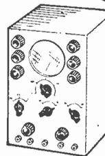
Cathode ray oscilloscope to show how circuits work . . .
