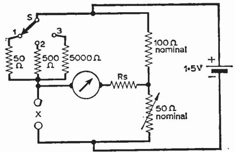
Fig. 9: A three-range bridge circuit for resistance measurements.
