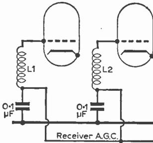
Fig. 3 (above): A modification to incorporate a.v.c.
