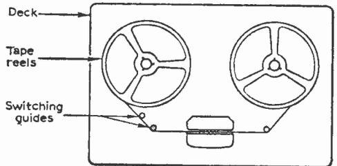
Fig 3: A suitable arrangement for the 'switching guides'.
