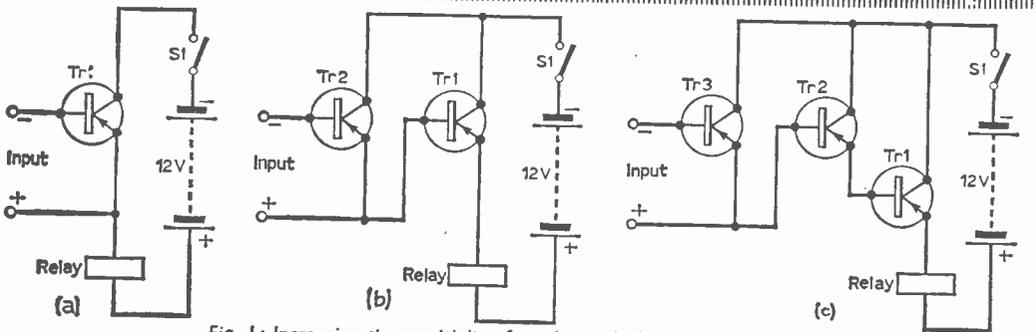
Fig. 1: Increasing the sensitivity of a relay with the aid of transistors.
