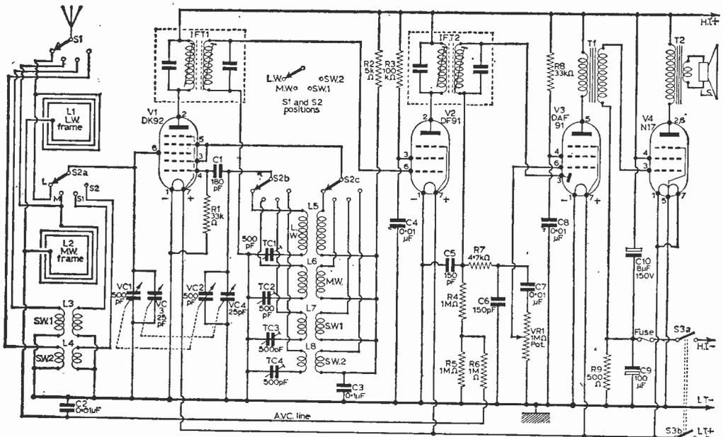
Fig. 1: The circuit diagram of the Chelmer.
