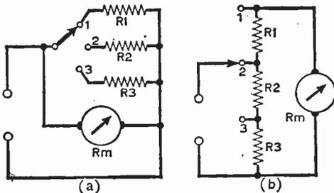
Fig. 7: Two arrangements for incorporating the current shunts.
