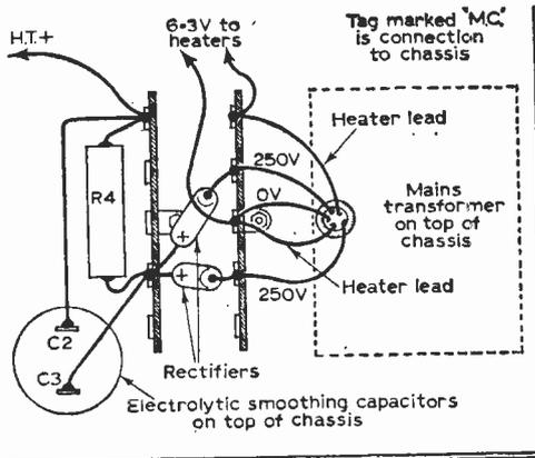
Fig. 4 (right): Wiring for the power supply.
