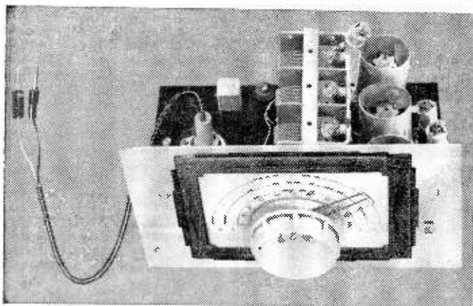
**T**HIS versatile unit can be built in a number of ways, depending upon the pocket and requirements of the constructor. In the first place it can be made as a one transistor tuner as described in the March 1963 issue of PRACTICAL WIRELESS, in which we had to wind on an extra coil for the base, on to the plug in coils designed by Denco for valve circuits.
