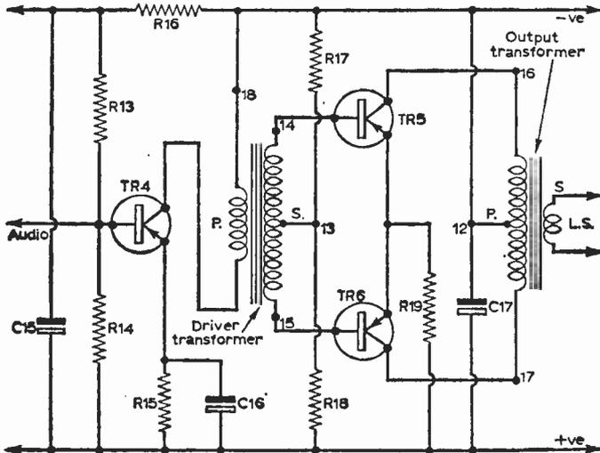
Fig 2: Driver and push-pull output stages of a typical receiver
