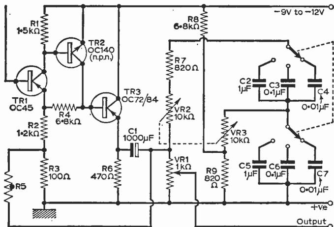
Fig. 5: The final, improved design for a Wien-bridge oscillator.
