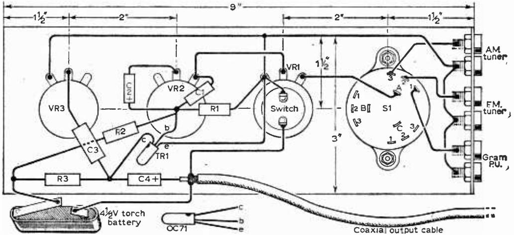
Fig. 2: Layout of components for the pre-amplifier, with dimensions for the four panel-control holes.
