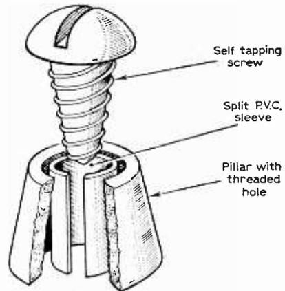
Fig. 3: Method of overcoming worn threads in plastic cabinets and mountings.
