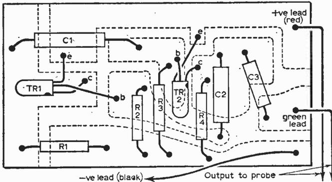
Fig. 4: The complete component layout and wiring diagram.
