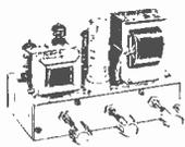
Designed for Hi-Fi reproduction of records A.C. Mains operation. Ready built on plated heavy gauge metal chassis, size 7 1/2 in. w. x 4 in. d. x 4 1/2 in. h. Input sockets E.C. 85, EL84, E280 valves, heavy duty double-wound mains transformer and output transformer matched for 3 ohm speaker, separate Bass, Treble and volume controls. Negative feedback line. Output 4 1/2 watts. Front panel can be detached and leads extended for remote mounting of controls.
