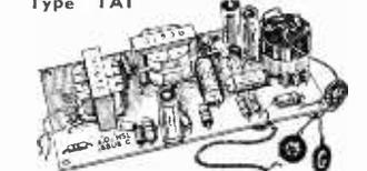
● Peak output in excess of 1 1/2 watts. ● All standard British components. ● Built on printed circuit panel size 6 x 3 in. ● Generous size Driver and Output Transformers. ● Output transformer tapped for 3 ohm and 15 ohm speakers. ● Transistors (4EFT114) or 81 Mullard (081D) and matched pair of 081 (4) ● 9 volt operation. ● Everything supplied, wire, battery clips, solder, etc. ● Comprehensive, easy to follow instructions and circuit diagram 1/6 (Free with Kit). All parts sold separately.
