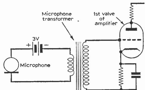
Fig. 2: The input circuit used with the microphone.
