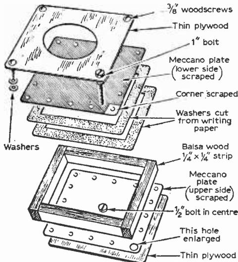
Fig. 1: Illustrating the simple construction of the microphone.
