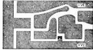
Fig. 3: An actual-size representation of the printed circuit board ( $1\frac{3}{8}$ in. x  $\frac{7}{8}$ in.).
