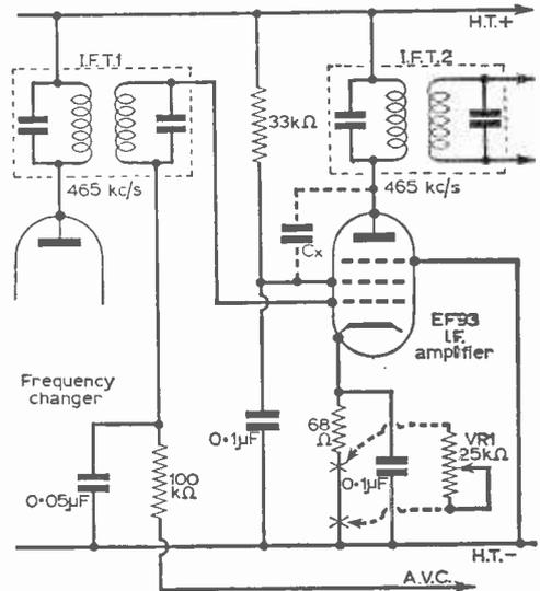
Fig. 4: A simple Q-multiplier circuit, using capacitor feedback between output and input tuned circuits, and incorporated in a typical i.f. stage using an EF93 or similar variable- $\mu$  pentode. Additional components are shown dotted. For value of  $C_x$ , see text.
