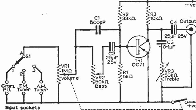
Fig. 1: Circuit diagram of the transistor audio pre-amplifier.
