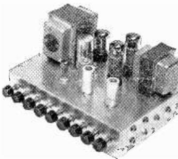
Five jack socket inputs, four with separate mixing volume controls, and one input "straight through". All inputs are of very high sensitivity, only 10 millivolts input is required for full output, making them suitable for all types of guitars and microphones. Separate Bass and Treble
