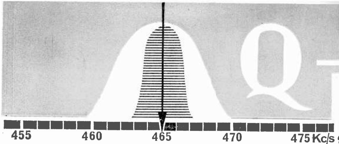
**I**N recent years the Q-Multiplier circuit has been widely used as a cheaper and more flexible method of varying selectivity than the crystal filter.
