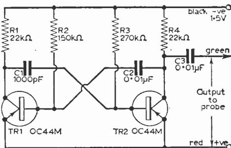
Fig. 1: The two-transistor circuit for this handy instrument.
