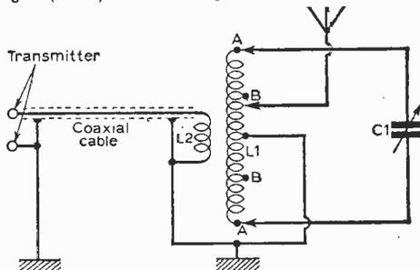
Resonance is indicated by a dip in anode current, as read on the meter. If the anode current is too low, C2 is opened slightly, and C1 re-tuned, this being repeated until the valve is drawing its expected anode current.
