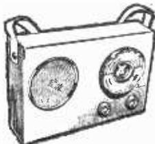
● 8 stages—6 transistors and 2 diodes
