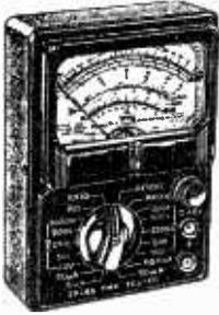
**50,000 O.P.V. MODEL TP 58.** Reads voltage up to 1,000 D.C. at 20,000 ohms per volt and A.C. at 10,000 O.P.V.; D.C. Current to 500mA; Resistance to 10 Megs.; Capacitance to 0.1µF; Decibels from -20 to +36. Size 3 1/2 in. x 5 1/2 in. x 1 1/2 in., £5.19.6.
