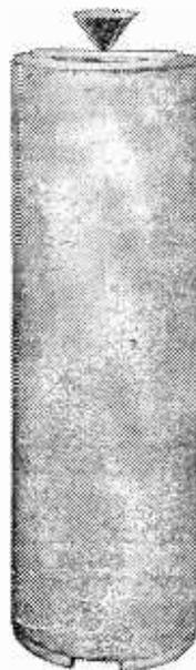
An inexpensive column speaker constructed from a concrete pipe and fitted with a good 8in. or 10in. unit has attracted much interest and admiration because of its clean open sound.
