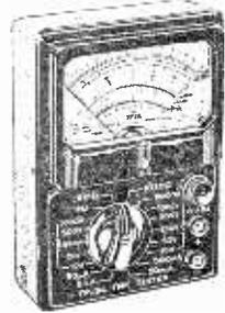
**20,000 O.P.V. MODEL TP 55.** Reads voltage up to 1,000 D.C. at 20,000 ohms per volt and A.C. at 10,000 O.P.V.; D.C. Current to 300mA; Resistance to 10 Megs.; Capacitance to 0.1µF; Decibels from -20 to +36, Size 3 1/2 in. x 5 1/2 in. x 1 1/2 in. £3.19.6.
