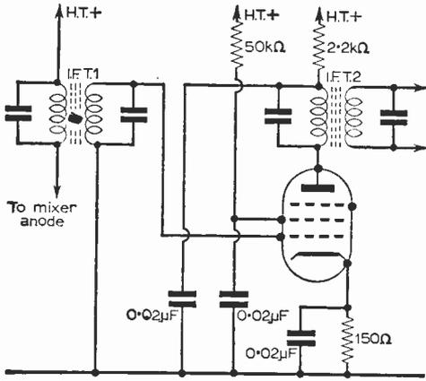
Fig. 80: The circuit of a simple i.f. amplifier.
