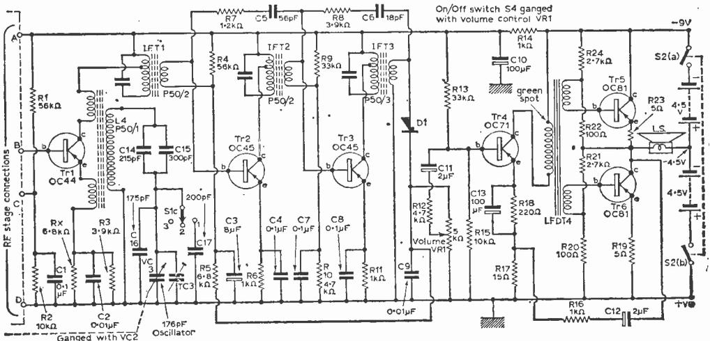
Fig. 3: The mixer, i.f. and audio stages which are built on a commercially available printed circuit board.
