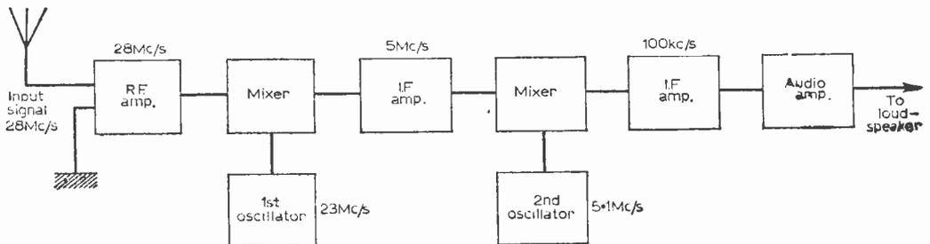
Fig. 79: A block diagram showing the stages of a double conversion superhet receiver.
