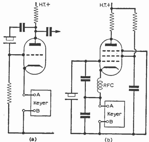
Fig. 2(a): The Pierce crystal oscillator and (b): the circuit modified somewhat.
