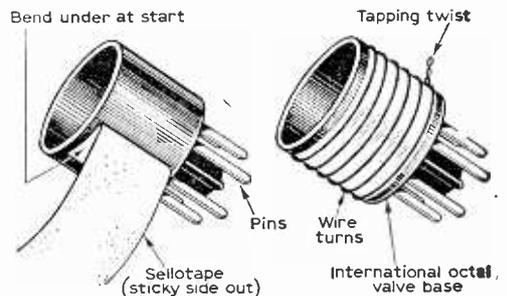
Fig. 1: Preparing a valve-base "former" and winding a typical coil.
