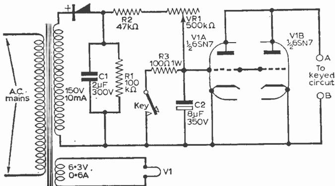
Fig. 3: The relatively simple valve keying circuit. This particular power supply arrangement was adopted as a matter of convenience, and a full-wave circuit could easily be used instead. The double-triode 6SN7 may be replaced by two 6J5's if desired.
