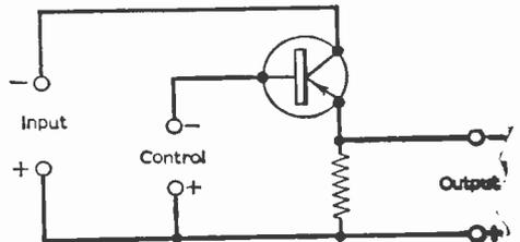
Fig. 3: The basic transistor "regulator".
