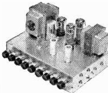
Five jack socket inputs, four with separate mixing volume controls, and one input "straight through". All inputs are of very high sensitivity only 10 millivolts input is required for full output, making them suitable for all types of guitars and microphones. Separate Bass and Treble controls, giving a wide range of lift
