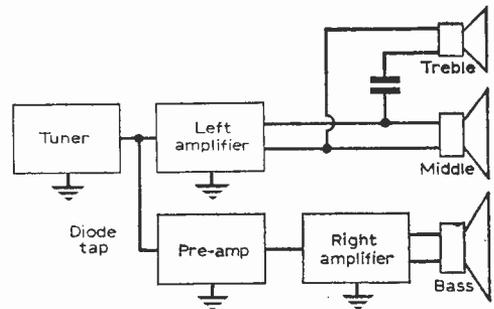
Fig. 2: A block diagram representation of the author's equipment set-up.
