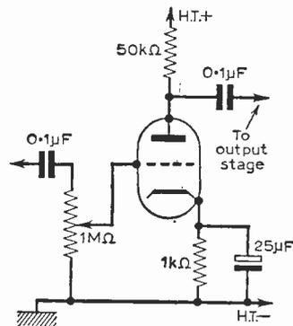
Fig. 83: A simple Class A triode a.f. amplifier.
