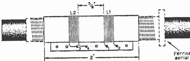
Fig. 3: Showing how L1 and L2 are wound over the receiver aerial.
