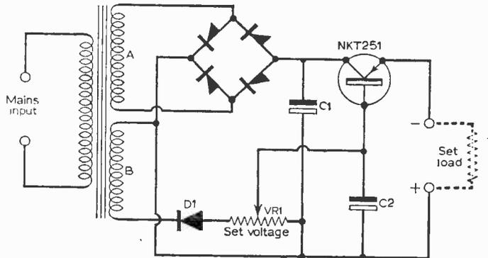
Fig. 4: A simple stabilised power supply used commercially.
