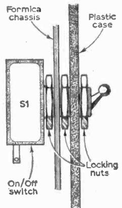
Fig. 3: The mounting of S1 which serves to clamp the chassis to the case.
