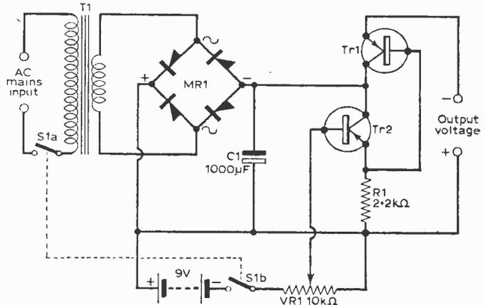
Fig. 5: A fully variable and regulated power supply.
