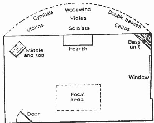
Fig. 1: The author's arrangement for his loudspeakers, indicating the area of "stereo" effect (Focal area) and the apparent displacement of the instruments of the orchestra.
