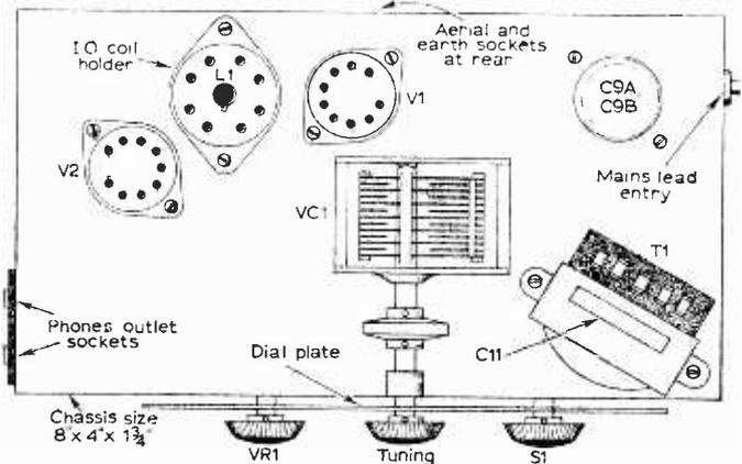
Fig. 5: A suggested chassis layout for the receiver.
