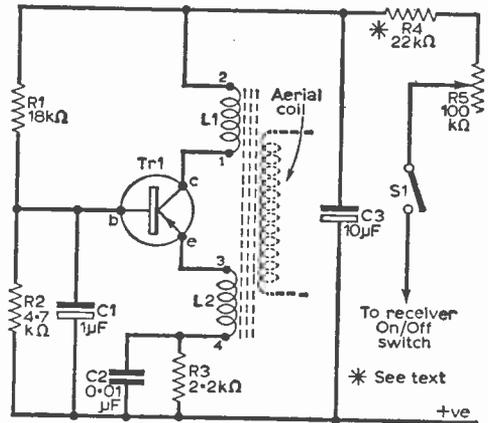
Fig. 1: The simple circuit of the device.
