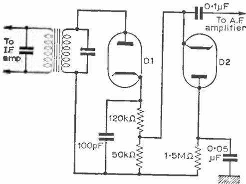
Fig. 87: A shunt noise limiter circuit.
