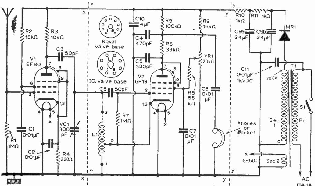
Fig. 3: A regenerative s.w. receiver design suitable for use with valve-base coils.
