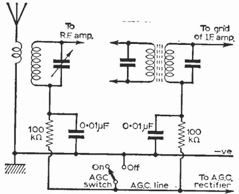
Fig. 82: How a.g.c. is applied to the controlled stages.
