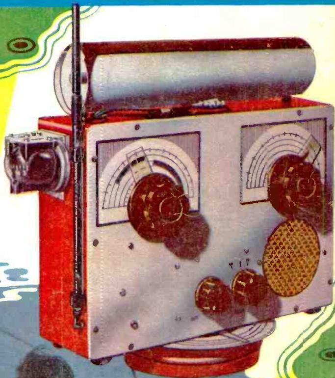
**8 Transistors - Printed Circuit**
