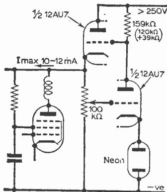
Dr. Wagner's alternative stabiliser circuit for F. G. Rayer's "Stabilised V.F.O." article in the March issue. Apart from saving the expense of a special valve, this circuit has other advantages over the original.
