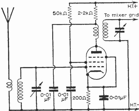
Fig. 85: Circuit of an r.f. amplifier.
