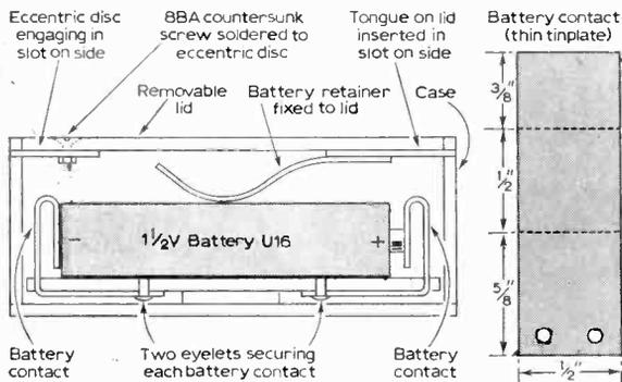
Fig. 6: Sectional elevation showing battery contacts.
