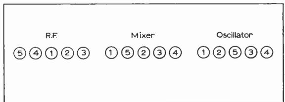
Fig. 2: Layout of the trimmers, viewed from the front of the receiver.
