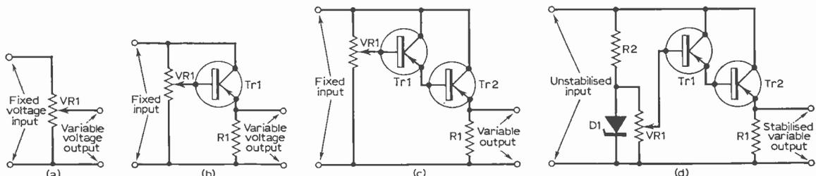
Fig. 1: (a) Basic circuit, (b) improvement by the addition of an emitter follower, (c) replaced by super-alpha pair emitter follower, (d) the Zener diode stabilises the circuit against changes in the supply voltage.
