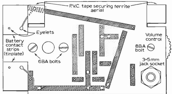
Fig. 2: Mounting board using "Cir-kit".
