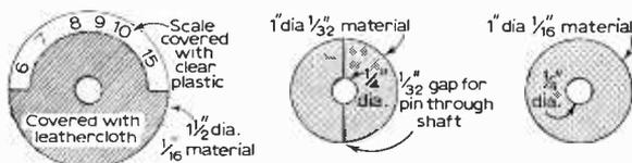
the shaft with the No. 60 drill. The knob is covered with leathercloth to match the case, except for the end of the shaft exposed in the centre for decorative effect. The scale round the edge is marked approximately in hundreds of kilocycles and is covered with clear plastic.
