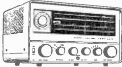
Outstanding value. High-class 4 band receiver covering 550kc/s-31 Mc/s. Seven valves plus rectifier, RF stage, illuminated "S" meter, 1.5µV sensitivity. Electrical bandspread on 80/40/20/15 and 10 metre bands. Slide rule dial, aerial trimmer. B.F.O., ANL, Output for phones or speaker. 115/220/240V. A.C. Brand new, guaranteed, with manual. 24 Gns. Carr. 10/-.
