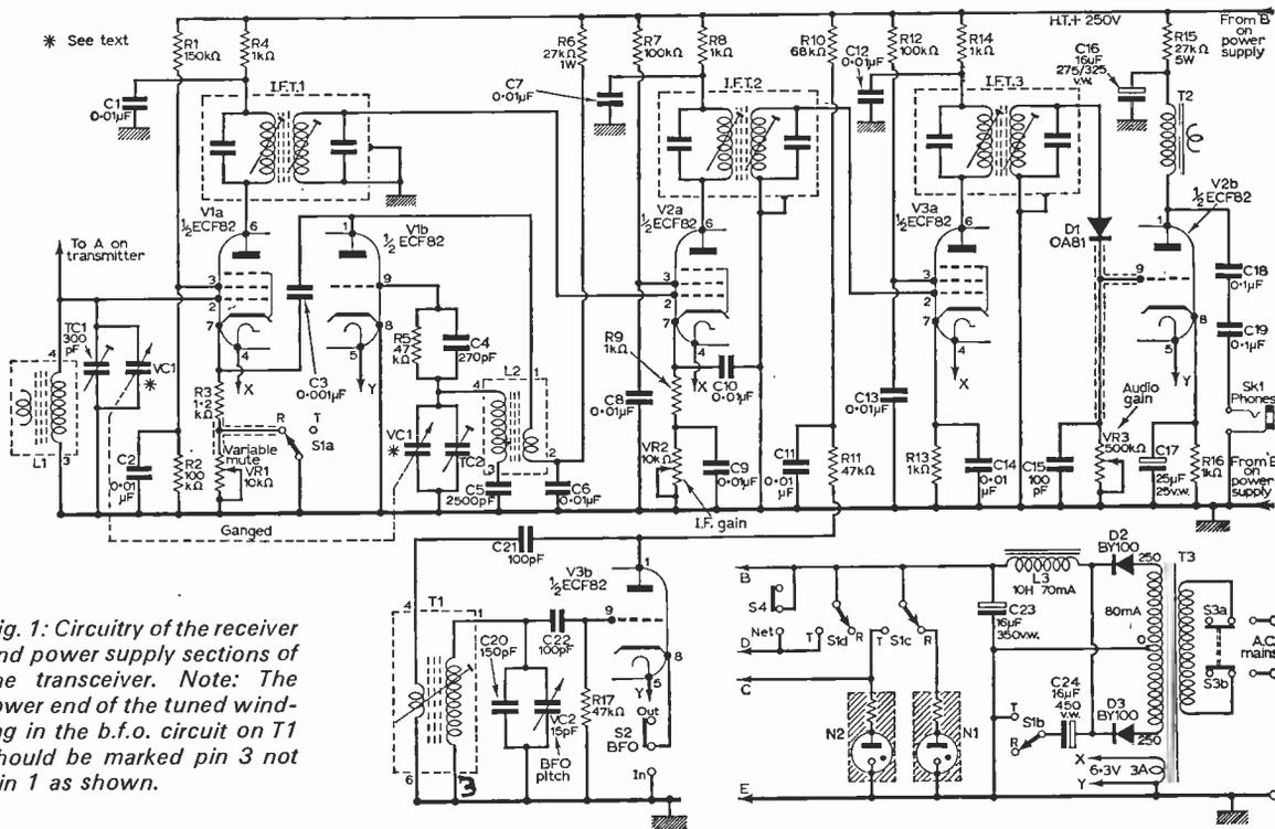
Fig. 1: Circuitry of the receiver and power supply sections of the transceiver. Note: The lower end of the tuned winding in the b.f.o. circuit on T1 should be marked pin 3 not pin 1 as shown.
