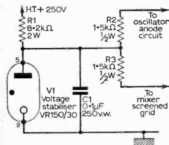
Fig. 4 (left): Simple stabiliser, see text for details.
