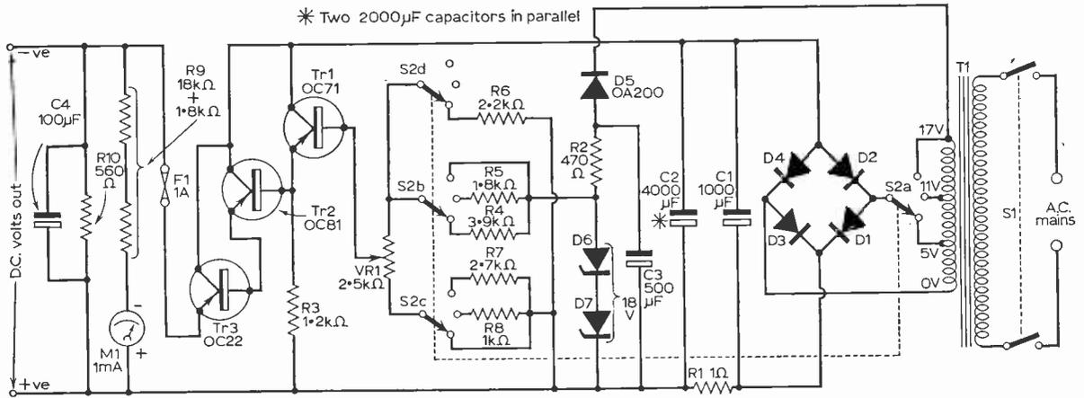
Fig. 2 (above): Complete circuit of the power supply unit. S2 is a four-pole, three-way wafer switch. D6-D7 could be a single 18V  $\frac{1}{2}$ W Zener diode.
