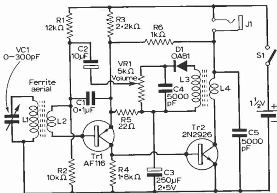
Fig. 1: Circuit diagram of the two-transistor radio.
