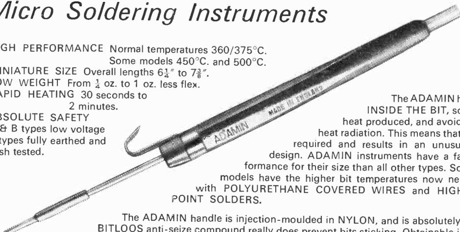
The ADAMIN has its element INSIDE THE BIT, so using all the heat produced, and avoiding excessive heat radiation. This means that less power is required and results in an unusually compact design. ADAMIN instruments have a far higher performance for their size than all other types. Some ADAMIN models have the higher bit temperatures now needed to cope with POLYURETHANE COVERED WIRES and HIGH MELTING-POINT SOLDERS.
