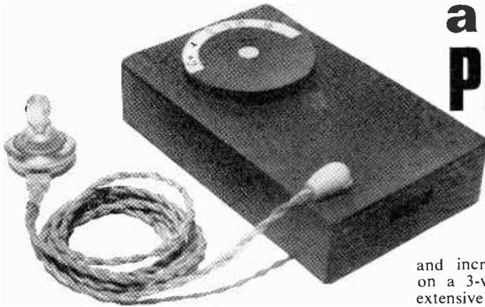
**R**EFLEXING in this personal radio makes two transistors do the work of four. Often it is not easy to carry out successfully, but works reasonably well in this circuit, even over an output stage feeding an earpiece. The quality depends upon using a good earpiece and the type specified is Ardenite ER250.
