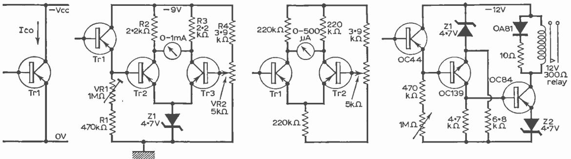
Left to right. Fig. 1: Path of leakage current  $I'_{co}$ . Fig. 2: A simple thermometer circuit using  $I'_{co}$  to record temperature fluctuations. Fig. 3: Alternative circuitry using a long tailed pair. Fig. 4: Circuit of a simple thermostat. (Tr1, Tr2, Tr3—OC70, 71, 44 etc).
