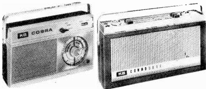
The latest in the K-B range of portable radios are the Cobra (left) and Commodore (right). Both models feature modular construction which makes servicing a very easy job—the r.f., i.f. and a.f. sections being three plug-in units. The transistor complement is the same in both receivers: 2 × AF117, OC70, 2 × AC127 and 2 × OC81.
