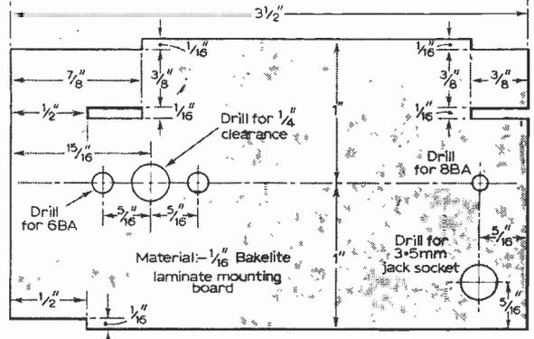
Fig. 4: Details of the mounting board.
