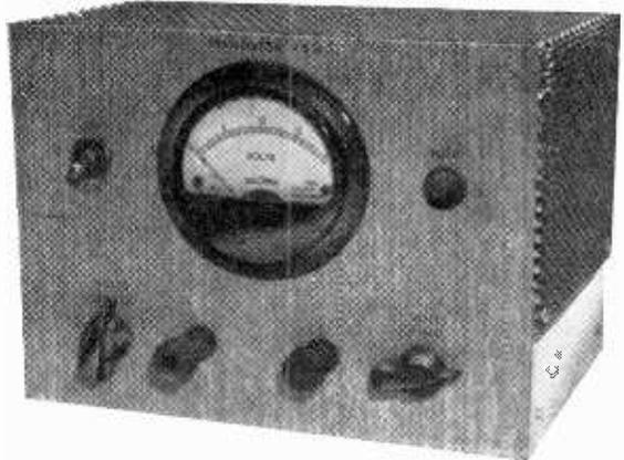
IN professional laboratories, considerable use is made of stabilised power supply units for experimental and development work, since these units have a low output impedance and give a constant output voltage over a very wide range of current demands.
