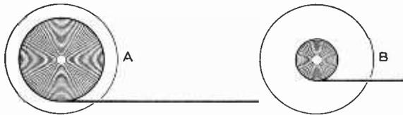
After one revolution the tape unwound at A is much longer than that at B. Length unwound =  $2\pi R$  where R is radius from centre of tape spindle to outer layer of tape.
