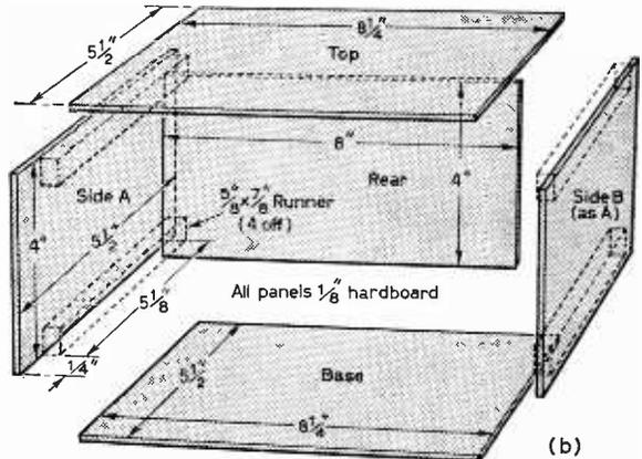
Fig. 5: 'a' shows the wiring details and 'b' cabinet details.
