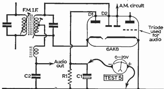
Fig. 3—4: The ratio-detector formed by two isolated diodes in a triple-diode-triode valve. A ratio detector test is shown.
