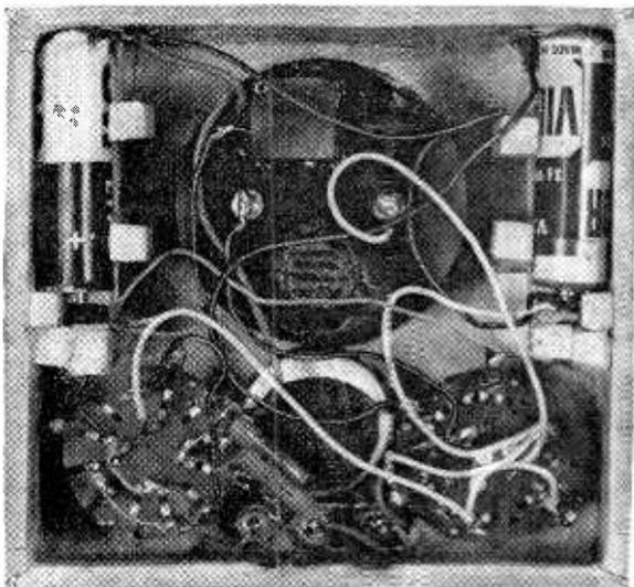
made either from bolts or from three crocodile clips as shown in Fig. 5. Constructors may use their ingenuity as to terminals but whichever type is used they must provide good positive action holding the wires tightly. They should also be kept clean.
