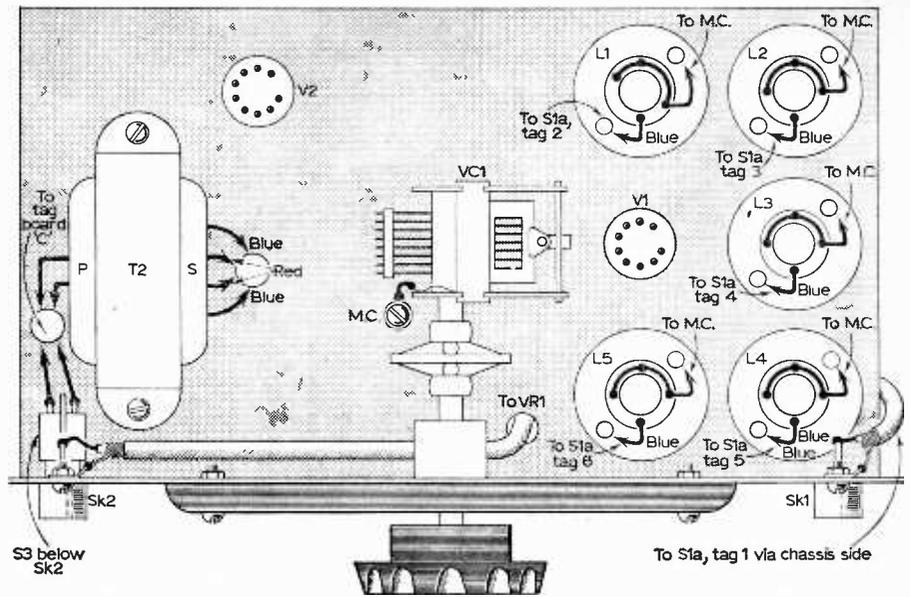
Fig. 4: Layout of components above chassis.
