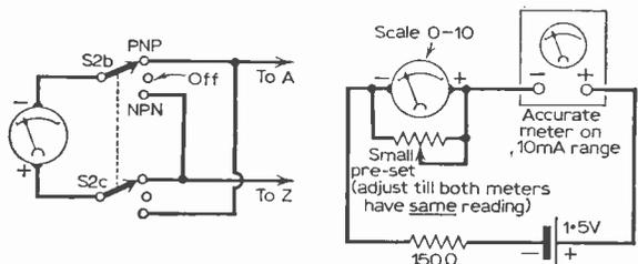
Fig. 2 (left): Modification for testing n-p-n transistors.
