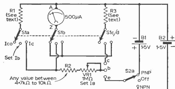
Fig. 1 (above): Basic circuit of the tester.
