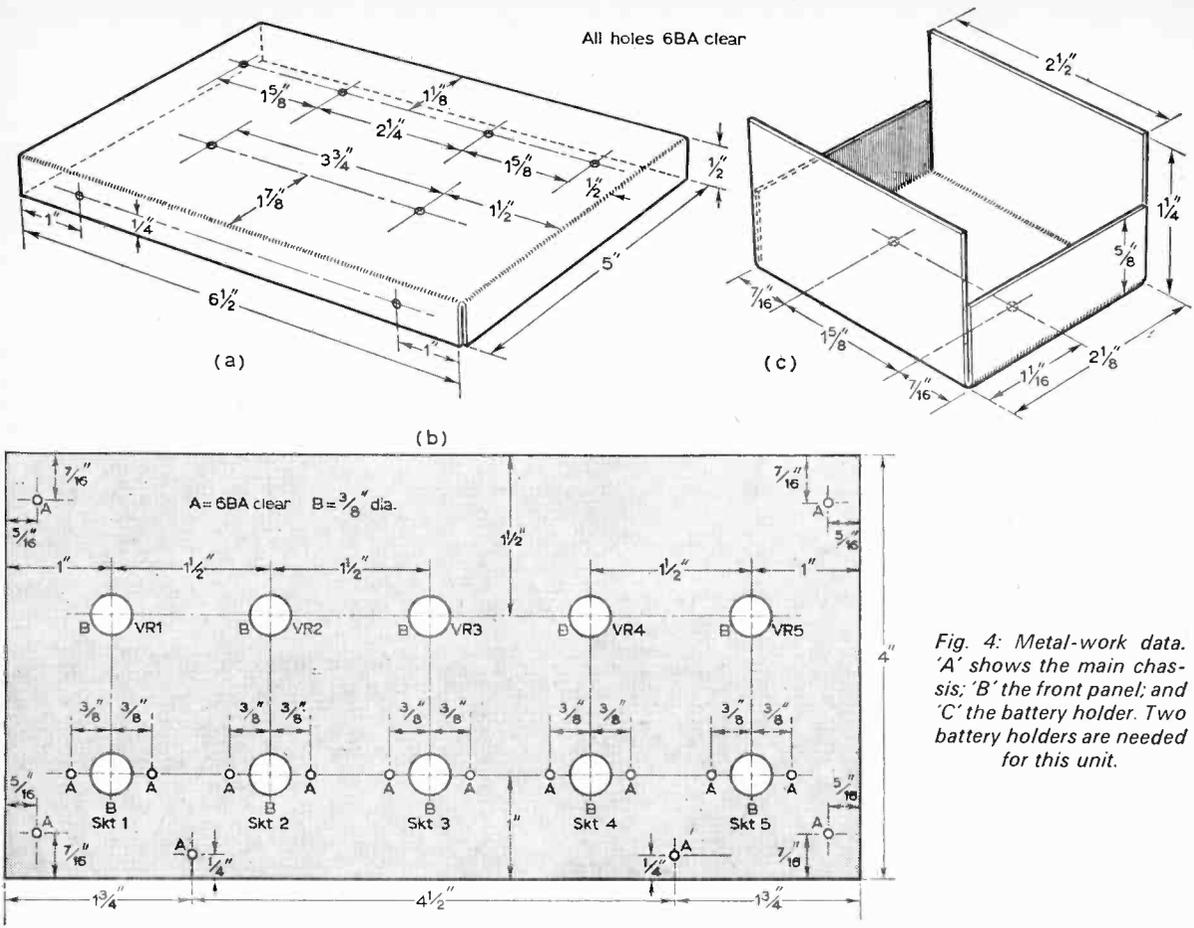
Fig. 4: Metal-work data. 'A' shows the main chassis; 'B' the front panel; and 'C' the battery holder. Two battery holders are needed for this unit.
