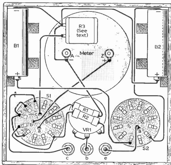
Fig. 4: Layout of the prototype tester. Compare this with the photograph in the heading on the right.
