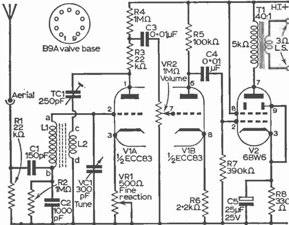
Fig. 1 (above): Circuit diagram of the Denette.
