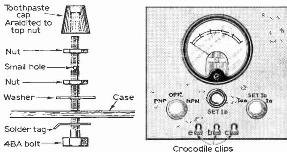
Fig. 5: Suggested approach to the problem of making suitable terminals, these may be modified bolts, or made from crocodile clips.
