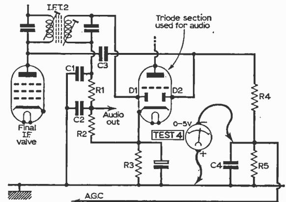
Fig. 3—3: An a.m. detector and a.g.c. circuit, showing a test for a.g.c.
