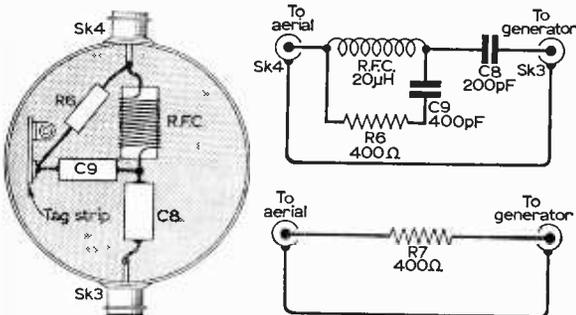
Fig. 5 (left): Layout of dummy aerial.
