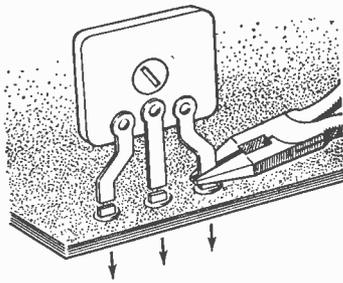
Fig. 5: Make extension "bit" to reach awkward spots. Wire can also be looped around a meter probe to gain access to remote points.
