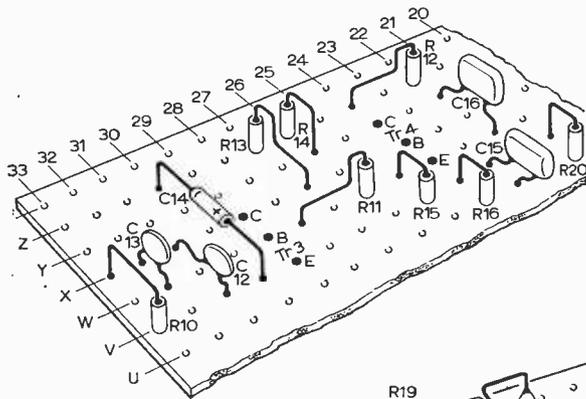
*Fig. 7 (above): I.F. stage, plus underside view of XA102 transistor.*
