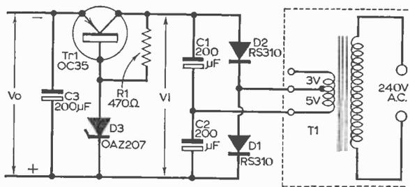
Fig. 1: Circuit diagram of the complete unit.
