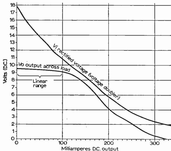
Fig. 3: Regulation curves of the power unit.
