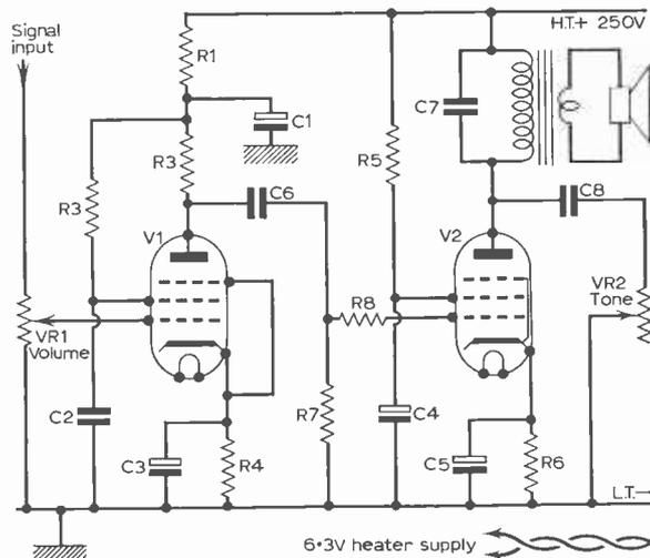
Fig 2: Theoretical circuit of simple audio amplifier
