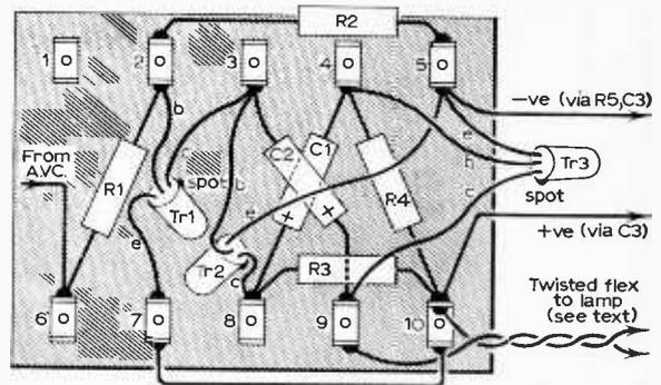
Fig. 2: Groupboard showing layout of components—note that C5/R3 are mounted externally but, this is not essential if a larger (ie. 12 or 14 way) groupboard is utilised.
