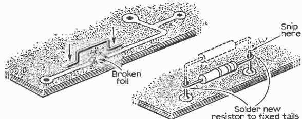
Fig. 2: Bridge joint with new section of wire. Avoid loose ends of foil and apply as little heat as possible to prevent broken ends from lifting.
