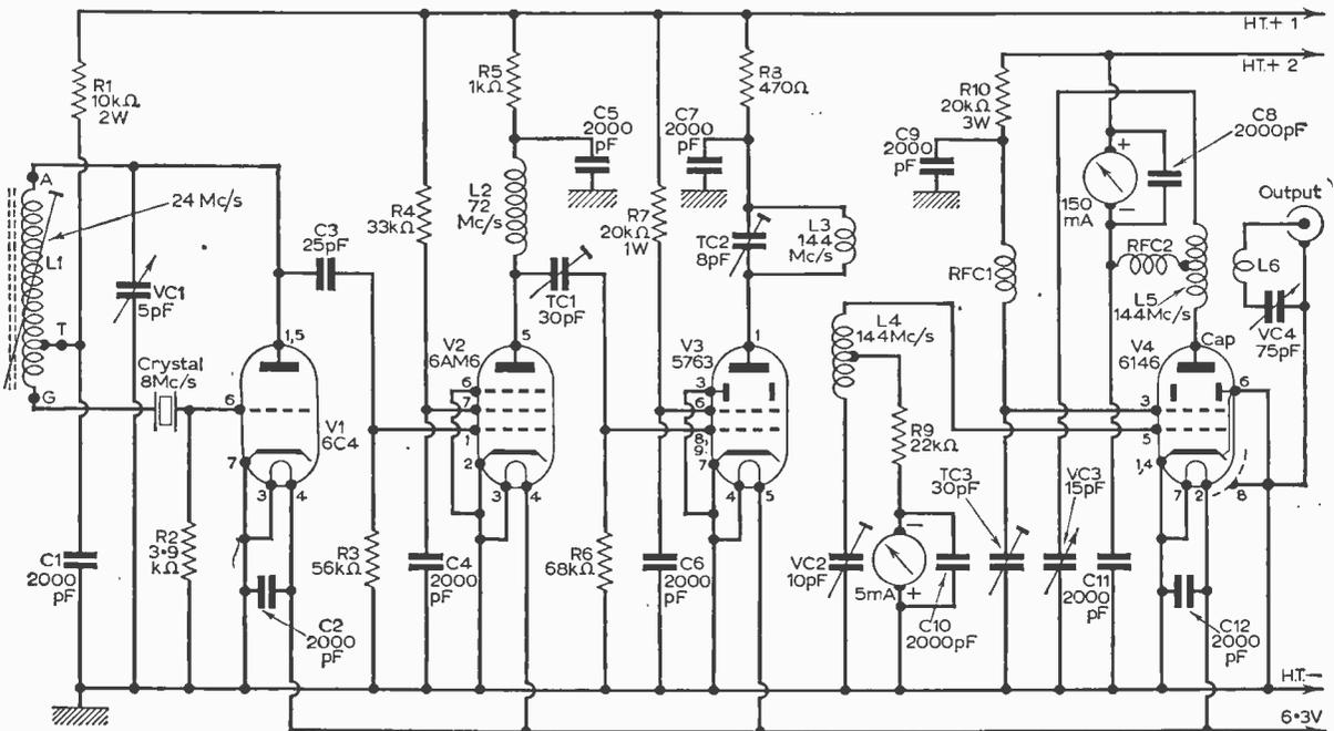
Fig. 1: Circuit diagram of the two metre transmitter.
