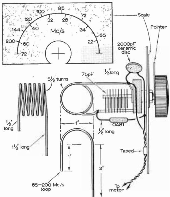
Fig. 5: Details and layout of suitable wavemeter.
