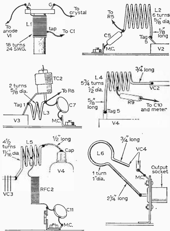
Fig. 4: Coil details. For winding instructions see text.
