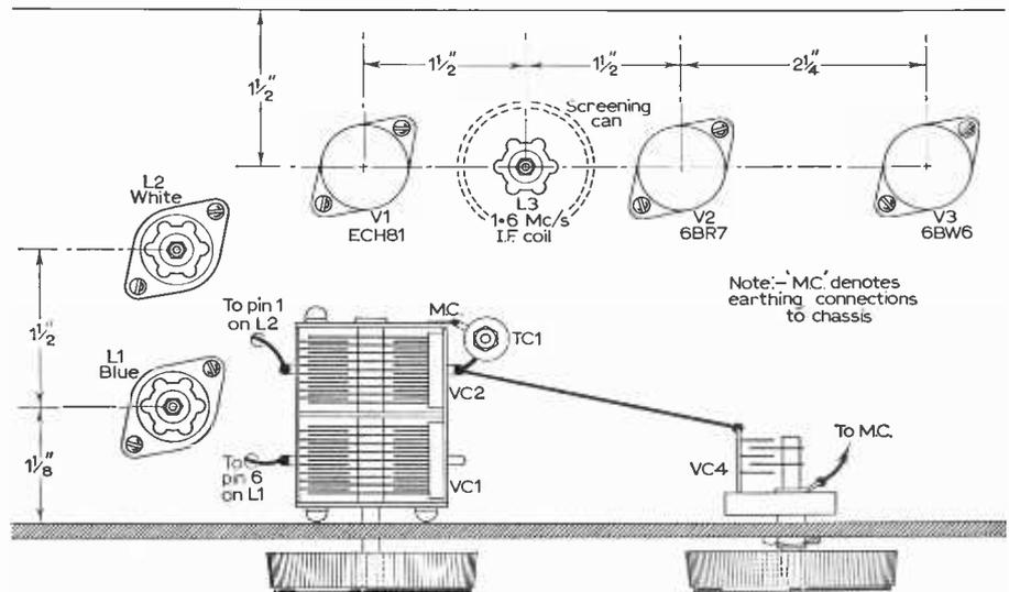
Fig. 2: Above-chassis layout and main drilling dimensions.
