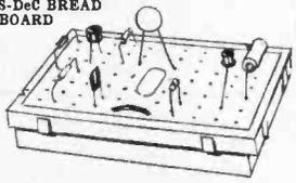
Solderless breadboard panels, for fast reliable component connections. Single De-Cs. One S-DeC with Control Panel, Jig and Accessories for solderless connections to controls, etc., with booklet "Projects on S-DeC" giving construction details for a variety of circuits. 29/6 P. & P. 2/6.
