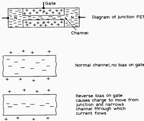
Fig. 15: Principle of the junction-gate field effect transistor.
