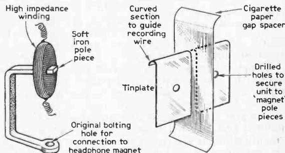
Fig. 1: The headphone electromagnet.
