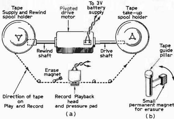
Fig. 7: The tape transport and erase systems.
