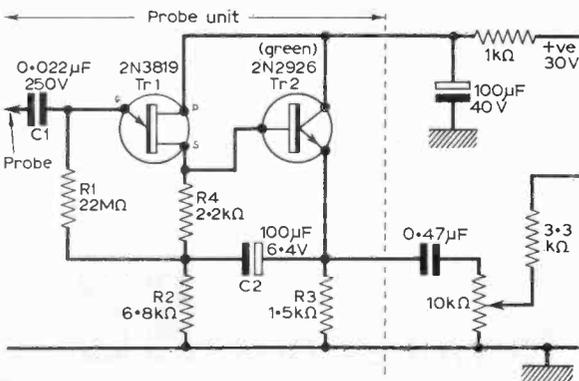
Fig. 3: The final circuit of the probe, using an f.e.t. in the first stage.
