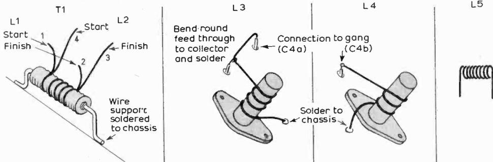
5+5 turns, 32s.w.g. enamelled, bifilar wound in groove of RS type A core.
