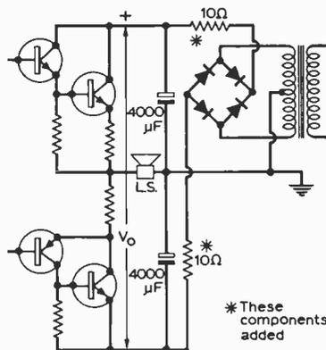
have found that the cause is the output d.c. blocking capacitor charging through the loudspeaker.
