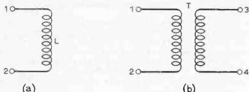
Fig. 1: Circuit symbols. (a) Inductor. (b) Transformer.
