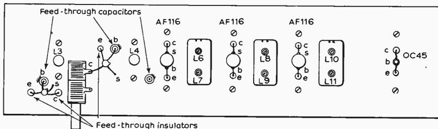
drilled through the paxolin centres showing through the holes previously drilled in the chassis, and through which the transistor leads will be inserted later.
