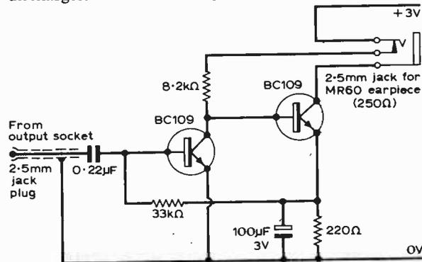
Fig. 6: A simple transistor amplifier suitable for use with the G.D.O.
