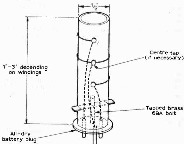
Fig. 11: The Author's method of coil construction.
