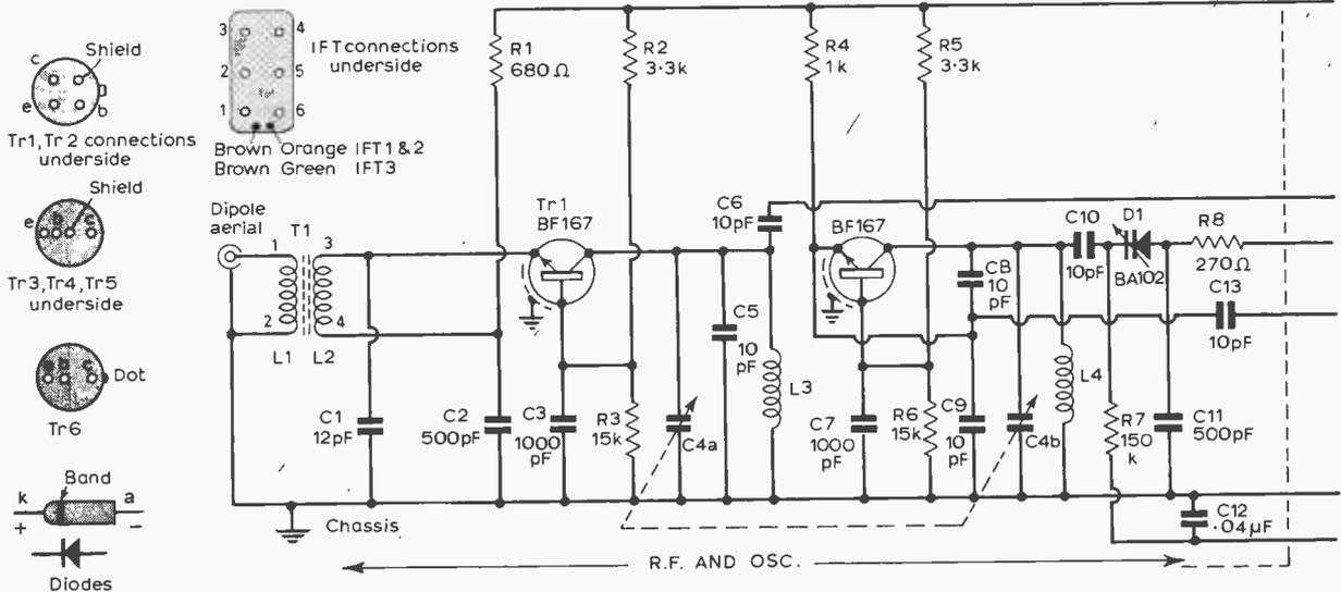
Fig. 1: The complete circuit of the transistor f.m. tuner, with automatic frequency control incorporated. Automatic gain control and an
