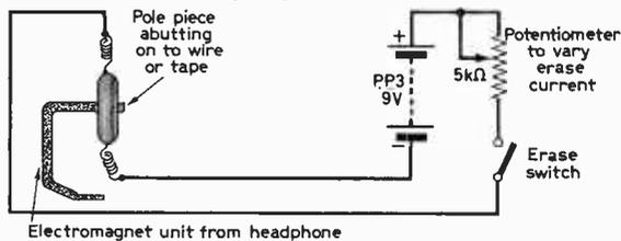
Fig. 6: The arrangement for switched D.C. erasure.
