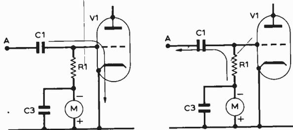
Fig. 2: Showing the flow of grid current.
