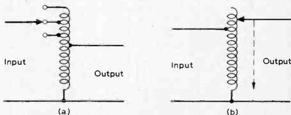
Fig. 8: Auto transformers. (a) Fixed tapped. (b) Variable.
