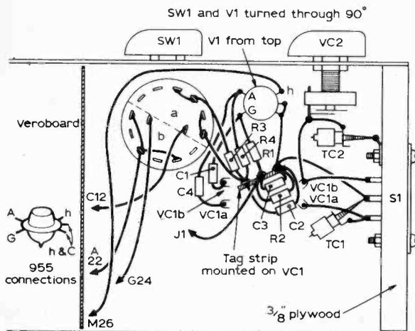
Fig. 10: The wiring of the Oscillator section.
