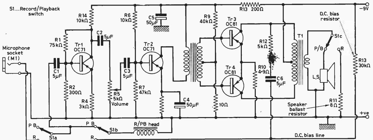
Fig. 8: A practical transistor tape recorder amplifier.
