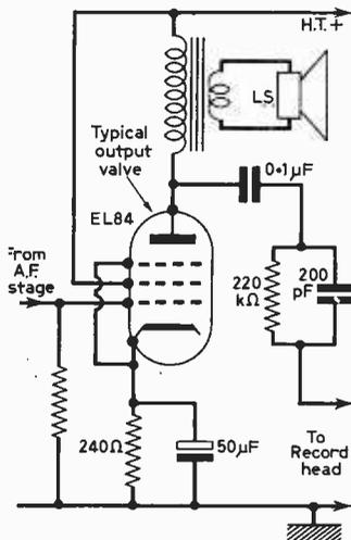
Fig. 3: Tapping off from an output valve.
