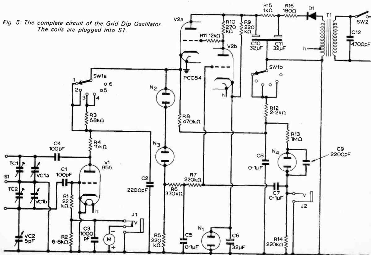
stabiliser output variations, thus providing an audible indication of the stabilisation efficiency. R8 and C8 filter out any negative feedback of the modulation signal.
