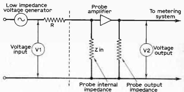
Fig. 5: Measuring the input impedance of the probe.
