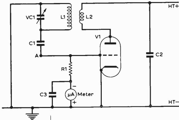
Fig. 1: A basic Grid Dip Oscillator circuit.
