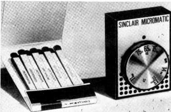
**SPECIFICATIONS**—Size: 1 13/16" x 1 7/16" x 1/2" (46x33x13mm). Weight incl. batteries: 1 oz. (28.35gm) approx. Tuning: Medium wave band with bandspread at higher frequency end. Earpiece: Magnetic type. Case: Black plastic with anodized aluminium front panel, spun aluminium dial.
