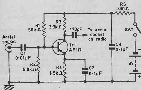
Fig. 1: The circuit of the signal booster.
