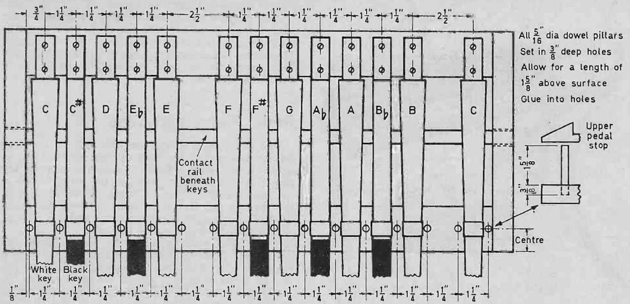
Fig. 3: Positioning of the pedals on the frame. Compare with the heading photograph of the completed unit.
