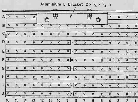
Fig. 2. Circuit board showing breaks required in conductor strips.
