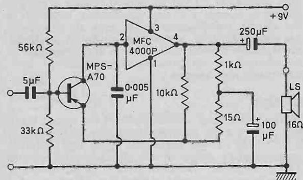
Fig. 3. Alternative circuit using a discrete pre-amplifier
