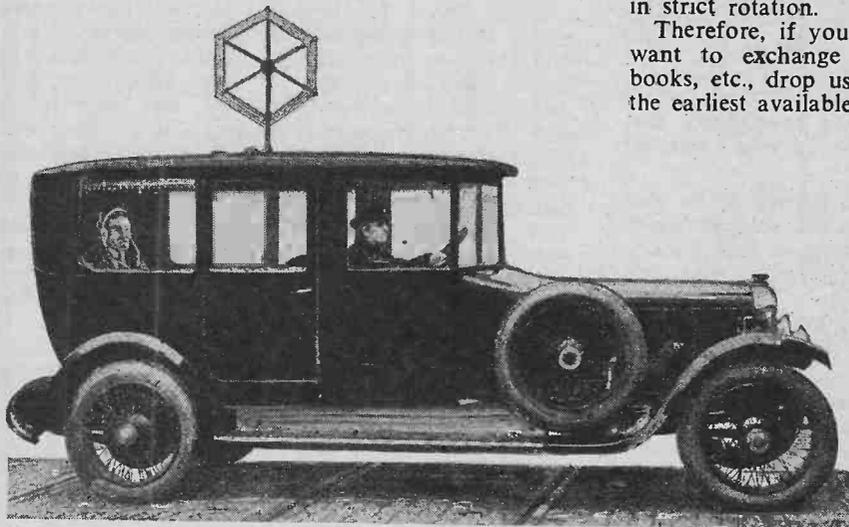
*This photograph shows a Daimler car equipped with a Marconiphone receiver and frame aerial. A similar car was used in the Lord Mayor of London's procession 1922.*
