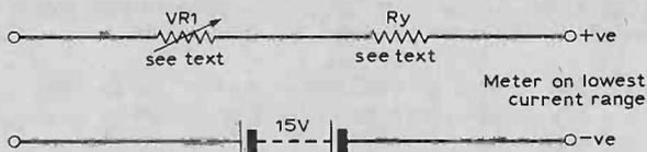
Fig. 3: A high resistance range can be added to nearly all test meters by using the above arrangement on the lowest current range.
