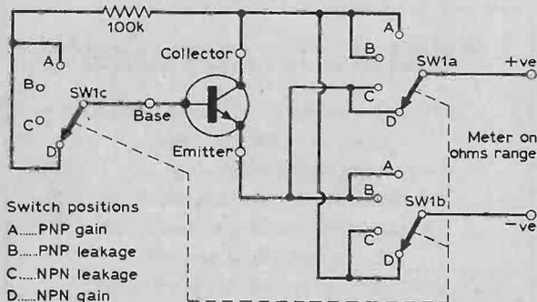
Fig. 1: The circuitry necessary for converting a multimeter to a transistor tester.
