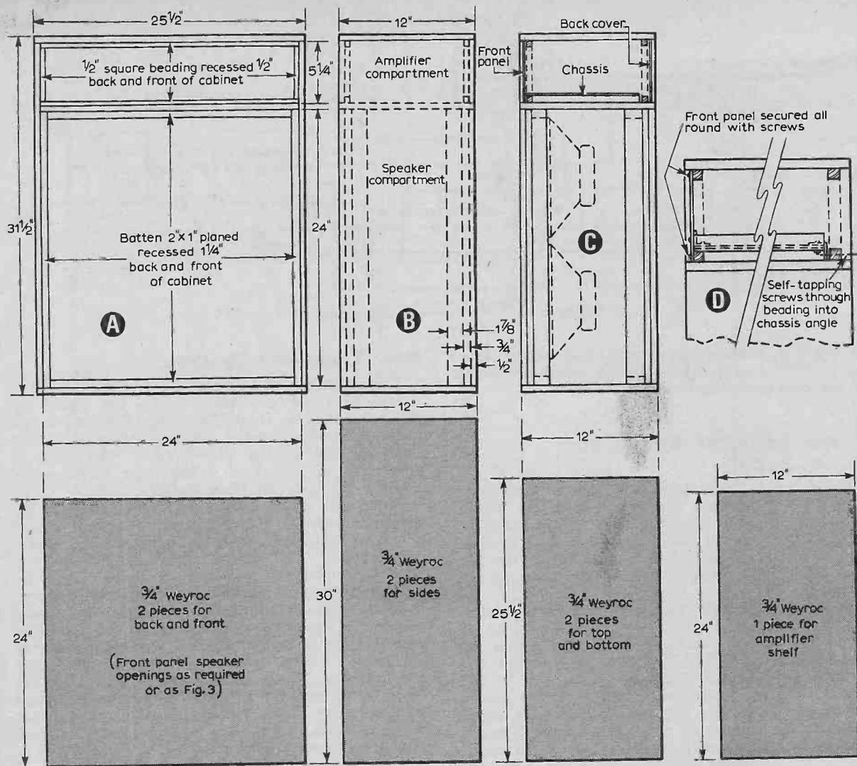
Figs. 2. (above) and 3 (right) give full details for the construction of the cabinet.
