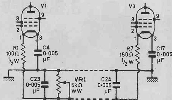
Fig. 3. Modified circuit incorporating an r.f. gain control.
