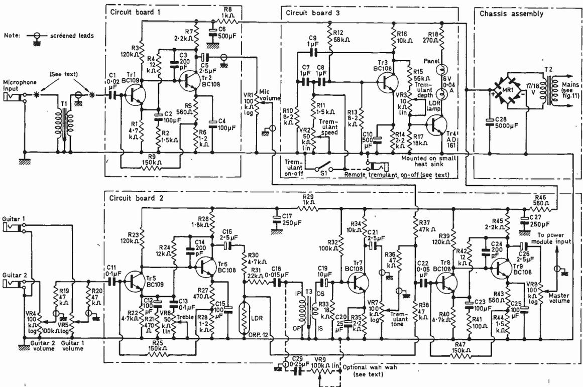
Fig. 5. Circuit of the complete pre-amplifier and its power supply.
