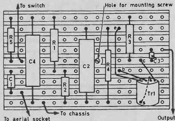
Fig. 2: The component layout on Veroboard.
