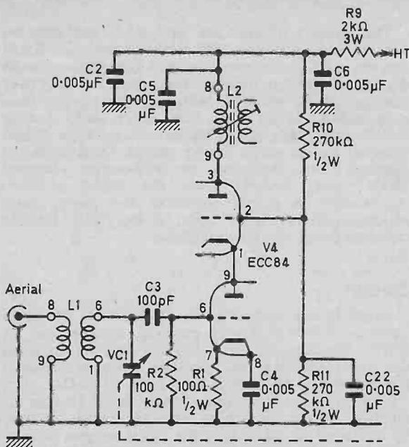
Fig. 2. Alternative r.f. stage using the cascode circuit.
