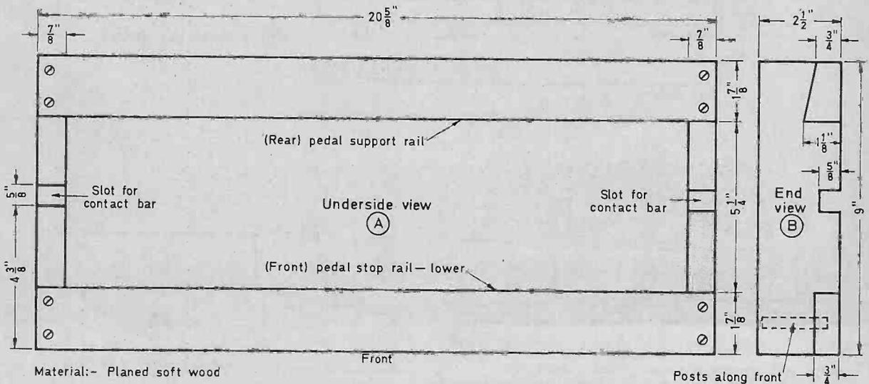
Fig. 2: Constructional details of the wooden pedal frame of the unit.
