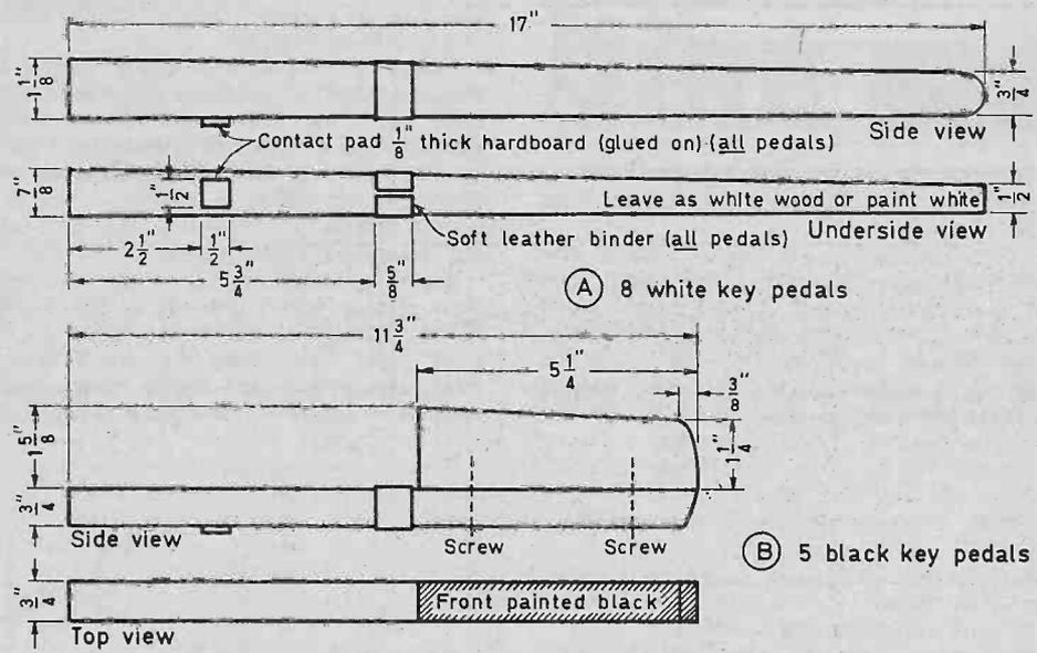
Fig. 4: Details for making the key pedals.
