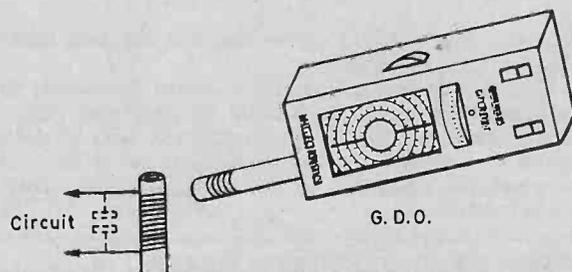
Fig. 1: Conventional use of a g.d.o. to investigate the resonant frequency of a tuned circuit.
