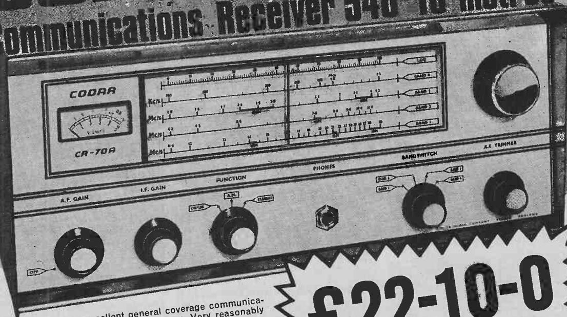
The Codar CR.70A is an excellent general coverage communications receiver for the keen short wave listener. Very reasonably priced at just £22.10.0 the CR.70A is outstanding value for money. In four stable ranges, the receiver covers from 540 metres medium wave, right through the shipping and coastguard frequencies all the short wave and international amateur bands up to and including 10 metres.
