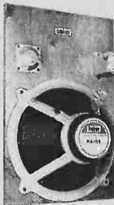
The remarkable quality and performance of the "Major" makes possible truly brilliant and rich sound from a single loudspeaker. It recreates the entire musical spectrum from 30 to 14,500 c.p.s. The unit consists of the latest double cone, woofer and tweeter cone together with a special Baker CERAMIC magnet assembly having a flux density of 14,000 gauss and a total flux of 145,000 Maxwells. Bass resonance 45 c.p.s. For Hi-Fi or P.A. Rated 20 watts. Voice coils available 3 or 8 or 15 ohms.
