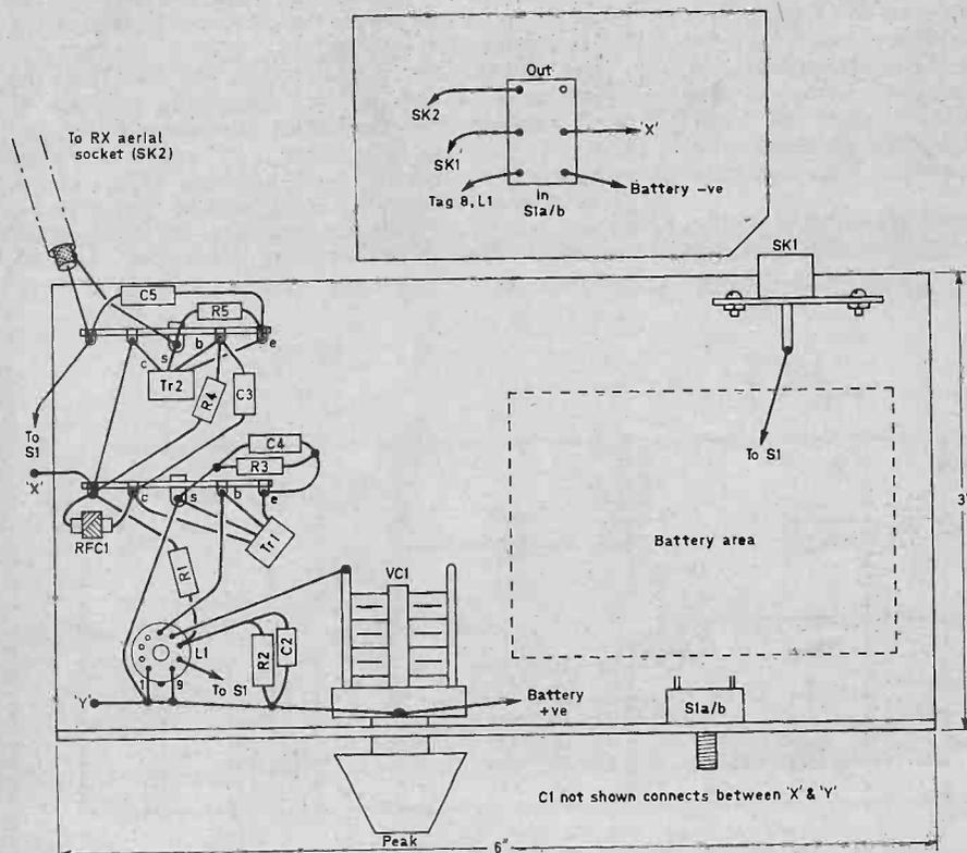
Fig. 2. Layout of the completed pre-selector.
