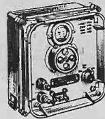
Small portable crystal controlled wavemeter. Size 7 x 7 1/4 x 4 in. Frequency range 500 Kc/s-10 Mc/s (up to 30 Mc/s on harmonics). Calibrated dial. Power requirements 300V. D.C. 15mA and 12V. D.C. 0.3A.
