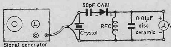
Fig. 4. Use of a signal generator instead of a g.d.o. to determine frequency of crystal.
