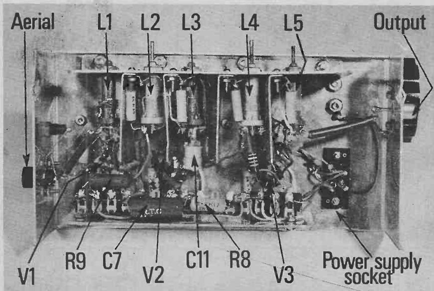
Bottom view of converter with identification of major components.
