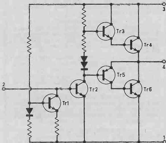
Fig. 1. Equivalent circuit of the MFC 4000P
