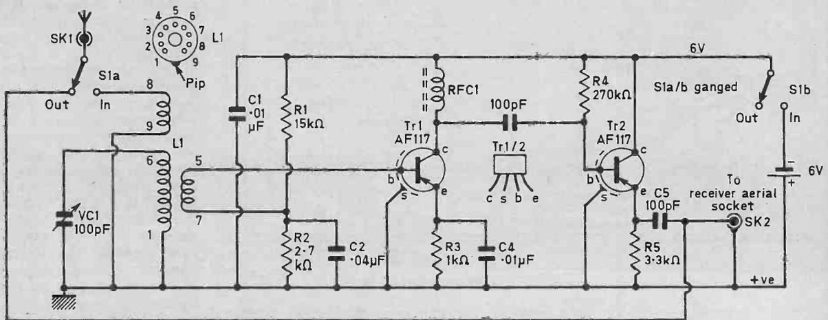
Fig. 1. Circuit of preselector. (Note:—the capacitor between Tr1 and Tr2 is C3, 100pF).
