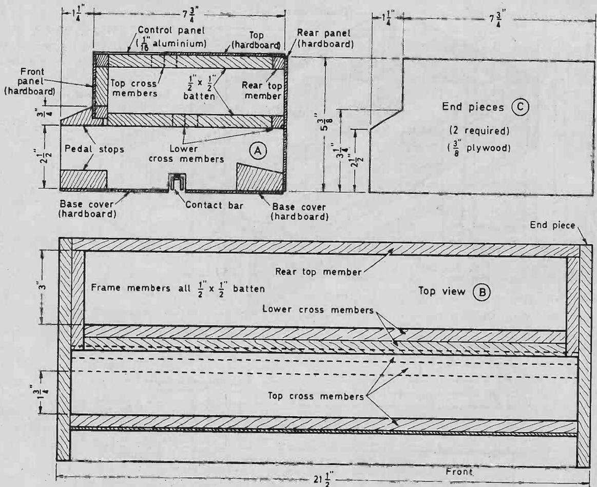
Fig. 7: Construction of the framework for the case.
