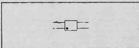
Actual size of the MFC 4000P. The dot identifies pin 1, the numbering going clockwise
