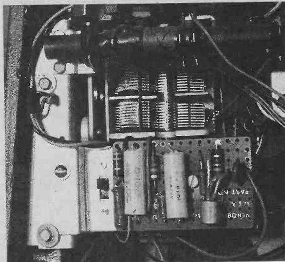
The signal booster may be mounted inside the existing cabinet as shown.
