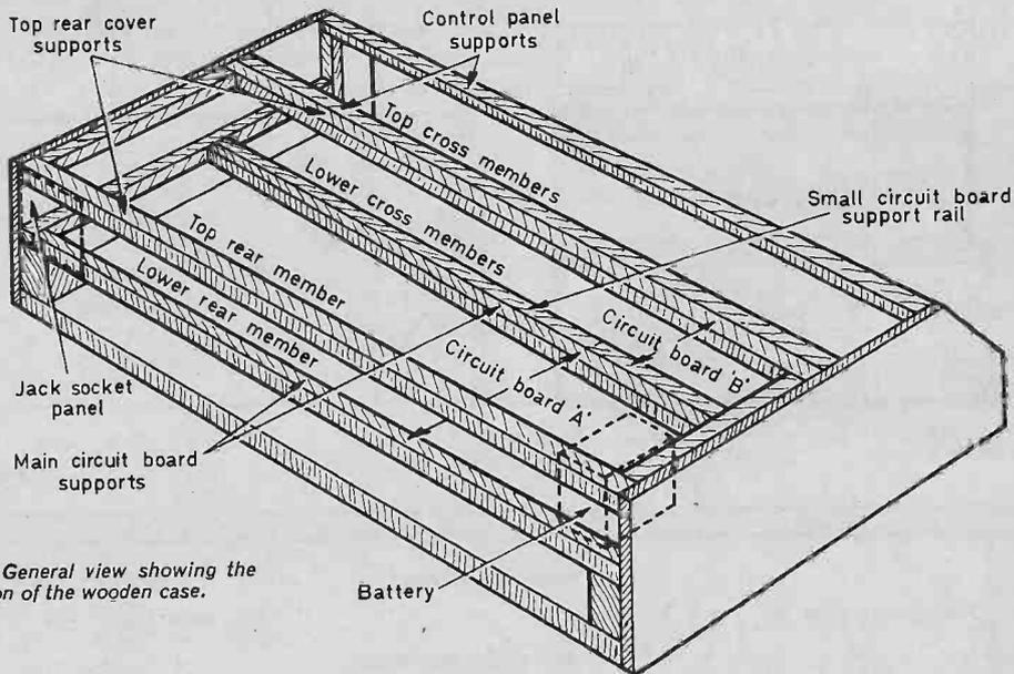
Fig. 8 (above): General view showing the construction of the wooden case.
