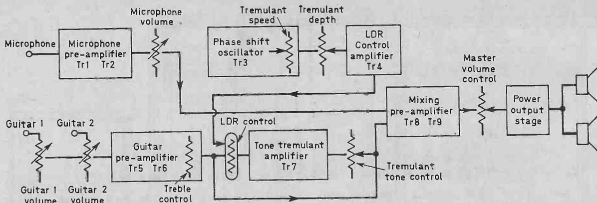
Fig. 1. Block diagram illustrating the function of each stage of the amplifier.
