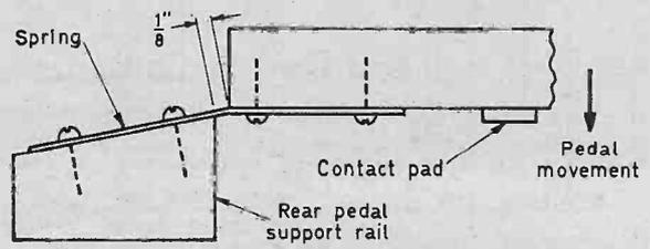
Fig. 6: Fitting of the springs to the pedal frame unit.
