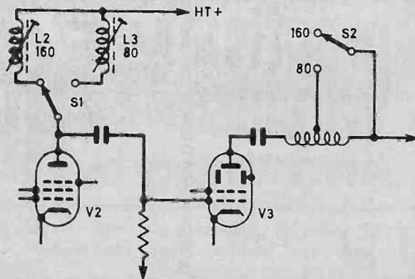
Fig. 2. Switching arrangements for 2-band operation of the b.a. and p.a. stages.
