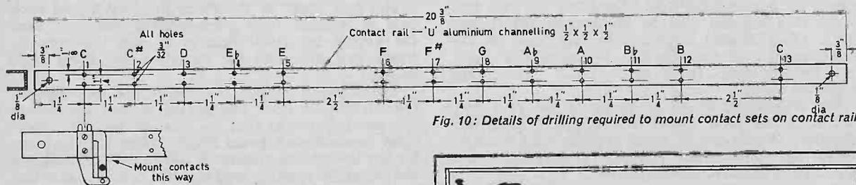
Fig. 10: Details of drilling required to mount contact sets on contact rail.
