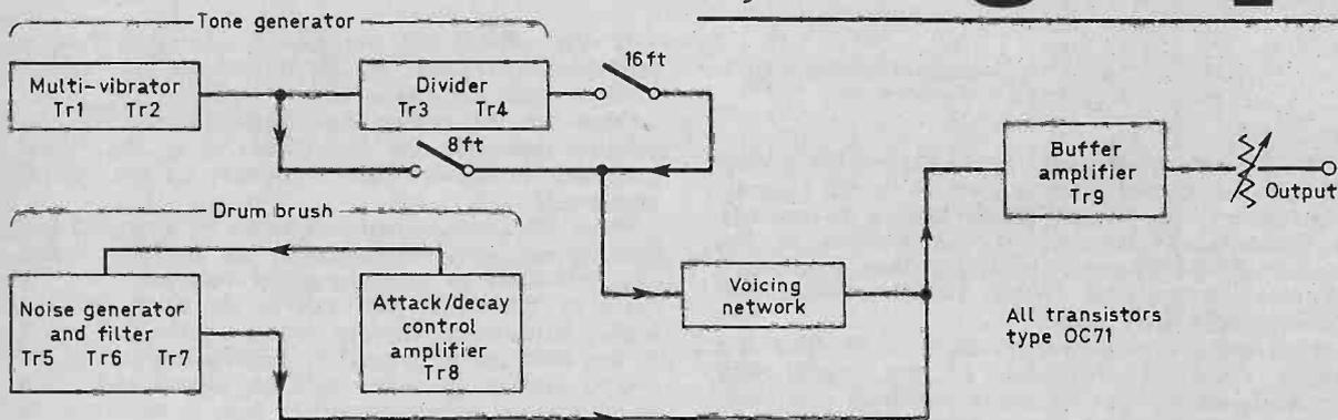
Fig. 1: Diagram showing the function of each stage of the Pedal Bass unit.
