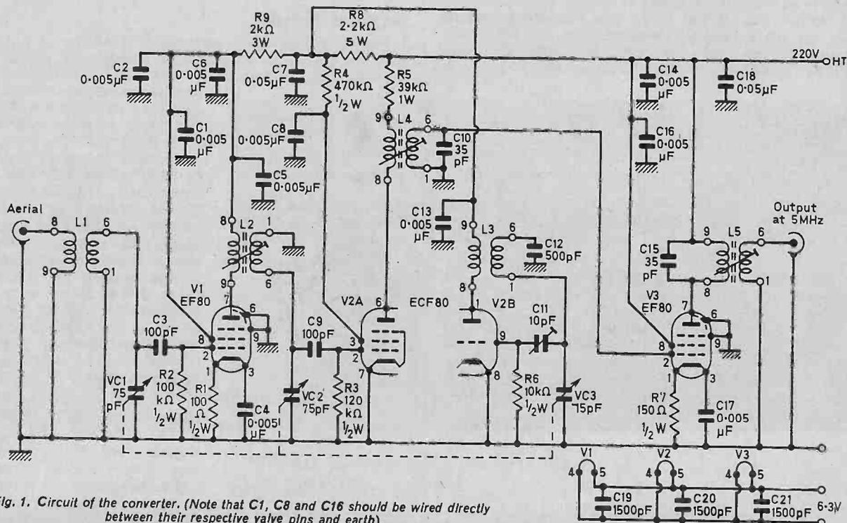
Fig. 1. Circuit of the converter. (Note that C1, C8 and C16 should be wired directly between their respective valve pins and earth).
