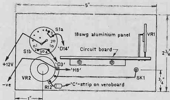
Fig. 4. Mounting of circuit board, function switch, attenuator and output socket on panel.
