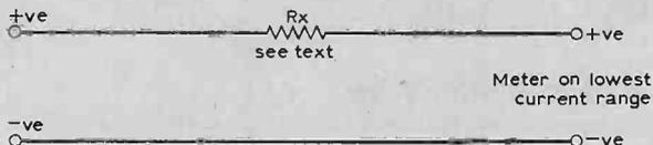
Fig. 2: Adding a 1V range is a simple matter but refer to the text for the value of Rx
