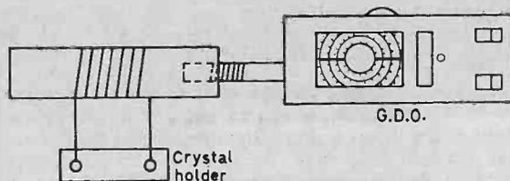
Fig. 2: Using a g.d.o. to "excite" a crystal at its fundamental frequency.
