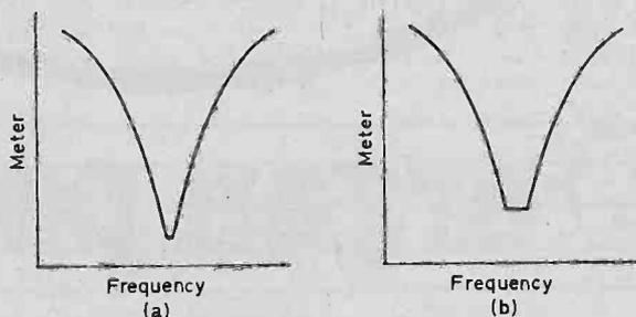
Fig. 3. (a) Grid current of g.d.o. when used conventionally as in Fig. 1. (b) grid current when used to "excite" crystal.
