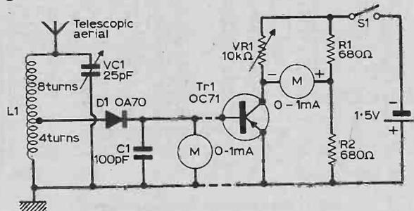
Fig. 1: The circuit of the field strength meter. Components to the right of the dotted line are only needed where the extra sensitivity version is required and here the meter is across the bridge circuit.
