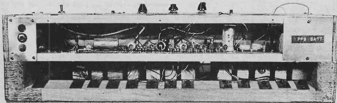
Rear view of unit shows, above, the circuit boards with the battery compartment to the right, and, below, the spring mounting of the pedals.
