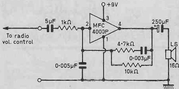
Fig. 2. Circuit of an audio stage suitable for a pocket radio
