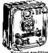
Small portable crystal controlled wavemeter. Size 7 x 7 1/2 x 4in. Frequency range 500 Kc/s-10 Mc/s (up to 30 Mc/s on harmonics). Calibrated dial. Power requirements 300V. D.C. 15mA and 12V D.C. 0.8A.
