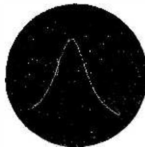
the i.f. circuits aligned for maximum output. The correct procedure, again, is to start at the rearmost and work forward, but even more care is needed and constant rechecking is necessary.
