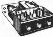
A superb solid state audio amplifier. Brand new components throughout. 6 silicon transistors plus 2 power output transistors in push-pull. Full wave rectification. Output approx. 13 watts
